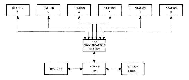
A special time-shared programming system has been developed providing each control area with immediate access to the central processor computer, and allowing ease of interpretation of data by computer users.
