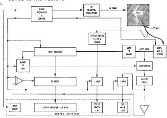
The pulses are encoded by the tables as serial x, y Gray-code position information which is sensed by the high-input impedance, pen-like stylus from the epoxy-coated tablet surface. This information is strobed, converted from Gray to binary code, assembled in a shift register, and gated in parallel to an interface register.
