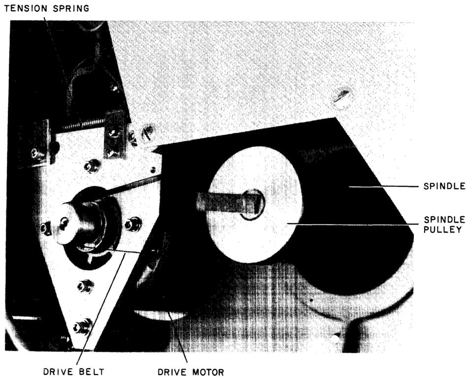
Figure 1-3 Spindle and Drive System
