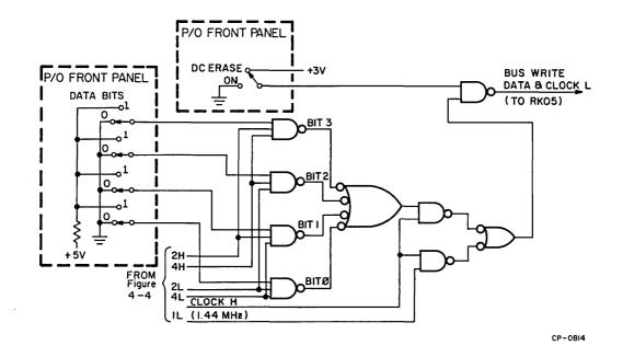
Figure 4-6 Clock and Data Multiplexer Logic
