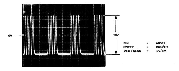
Figure 6-4 Cosine Amplitude/Offset Waveform
