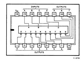
Figure A-1 7442 Package and Logic Diagrams
