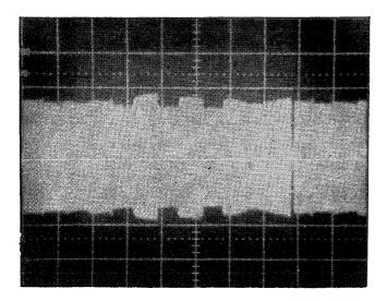
Figure 6-1b Spindle Runout (Considerable Runout)
