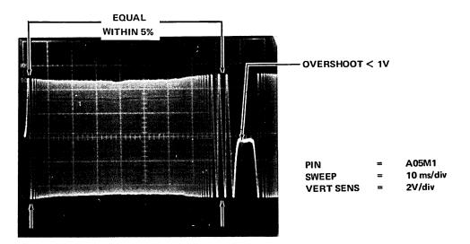
Figure 6-8 Full Stroke Position Waveform
