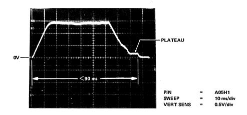
Figure 6-7 Full Stroke Waveform
