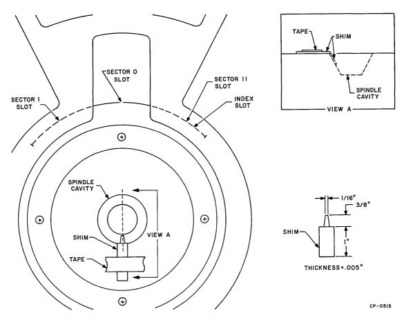
Figure 6-2 CE Test Cartridge Shim Installation
