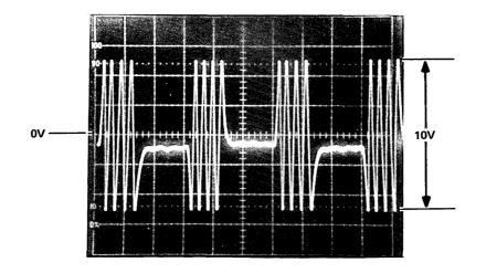
b. Incorrect Waveform (Signal not Symmetrical about Ground)
