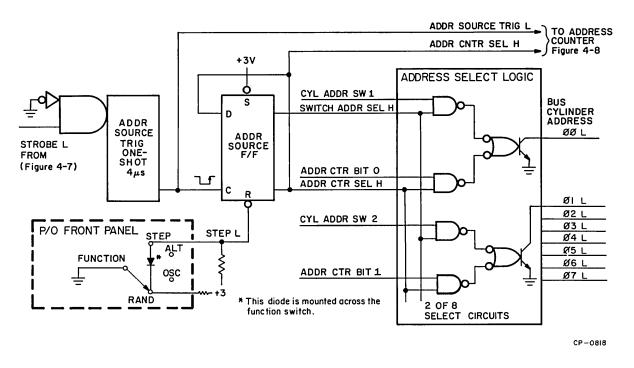
Figure 4-10 Cylinder Address Source Select Logic
