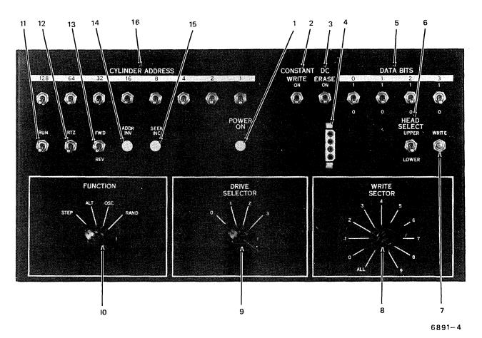
Figure 3-1 RK05 Exerciser Front Panel Controls and Indicators
