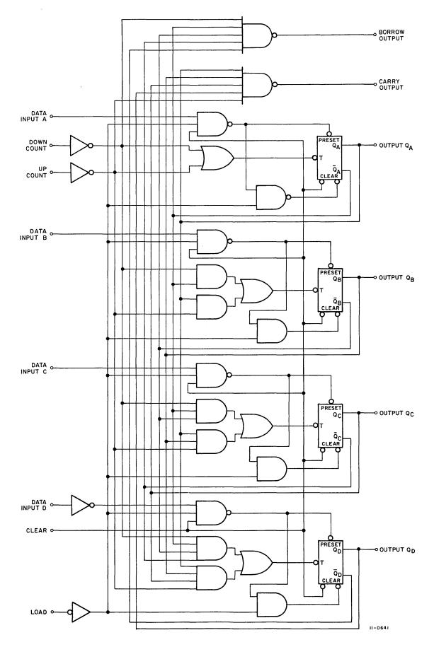
Figure A-4 74193 Logic Diagram
