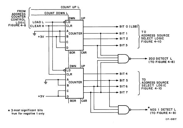
· Figure 4-9 Address Counter Logic
