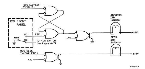
Figure 4-11 Fault Detect Logic
