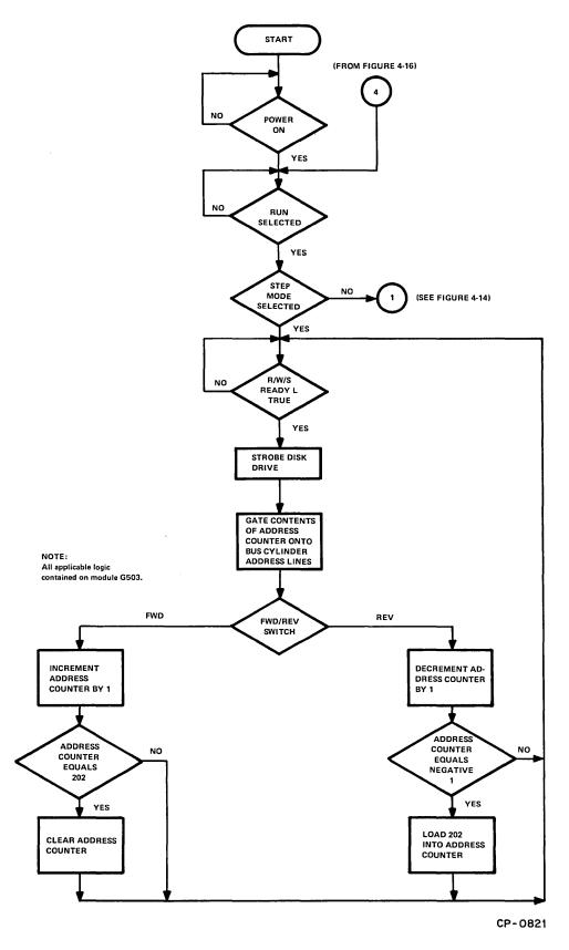
Figure 4-13 Positioner Exerciser Step Mode Flow Diagram
