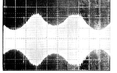
e. Head slightly misaligned. Larger left null indicates head position more than CYL 105.
