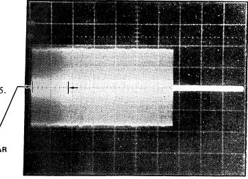
NOTE The alignment error is denoted as a signed percentage. The percentage is derived from the relative amplitudes of the two signal modes  $(x_1 \text{ and } x_2)$  according to the following
