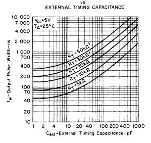
Figure A-3 DEC 74123 IC Output Pulse Width vs. External Timing Capacitance
