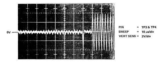
Figure 6-13 Index/Sector Waveform
