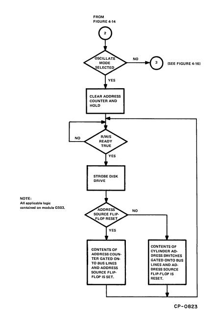
Figure 4-15 Positioner Exerciser Oscillate Mode Flow Diagram
