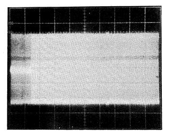
Figure 6-1a Spindle Runout (Negligible Runout)
