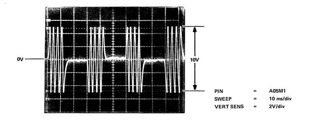
a. Correct Waveform (Symmetrical Signal)
