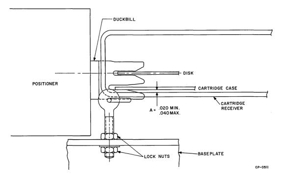
Figure 6-14 Cartridge to Receiver Clearance
