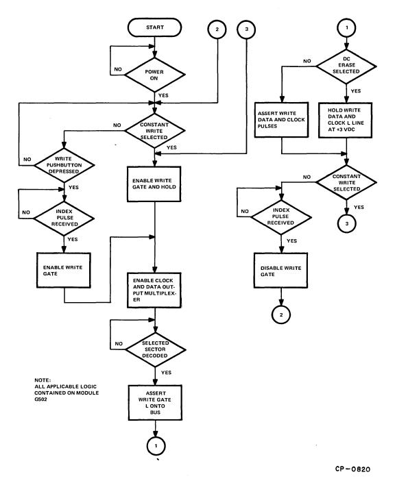
Figure 4-12 Writer Exerciser Flow Diagram
