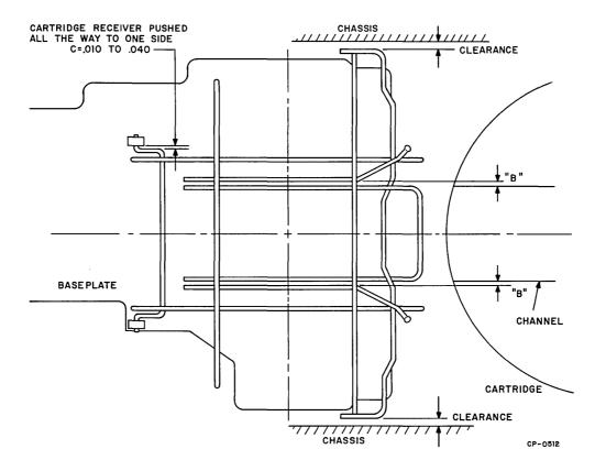
Figure 6-15 Cartridge Receiver Clearances
