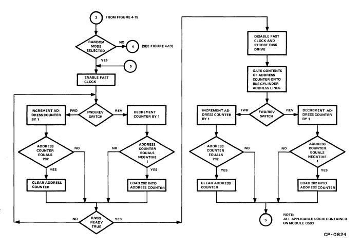
Figure 4-16 Positioner Exerciser Random Mode Flow Diagram
