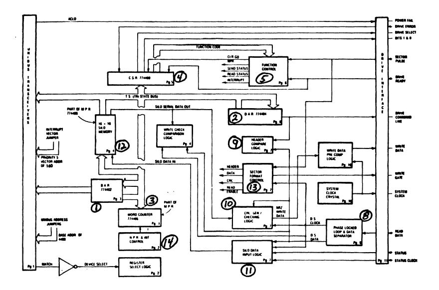
Figure **5** M7762 RL11 Basic Block Diagram
