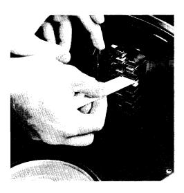
FIGURE 4-3. CLEANING HEADS IN DRIVE
