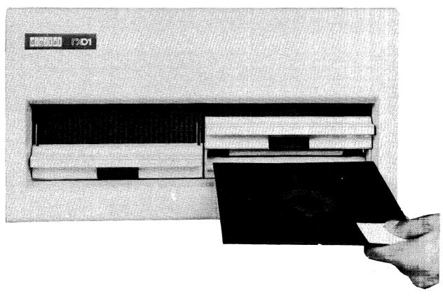
Figure 2-7 Flexible Diskette Insertion
