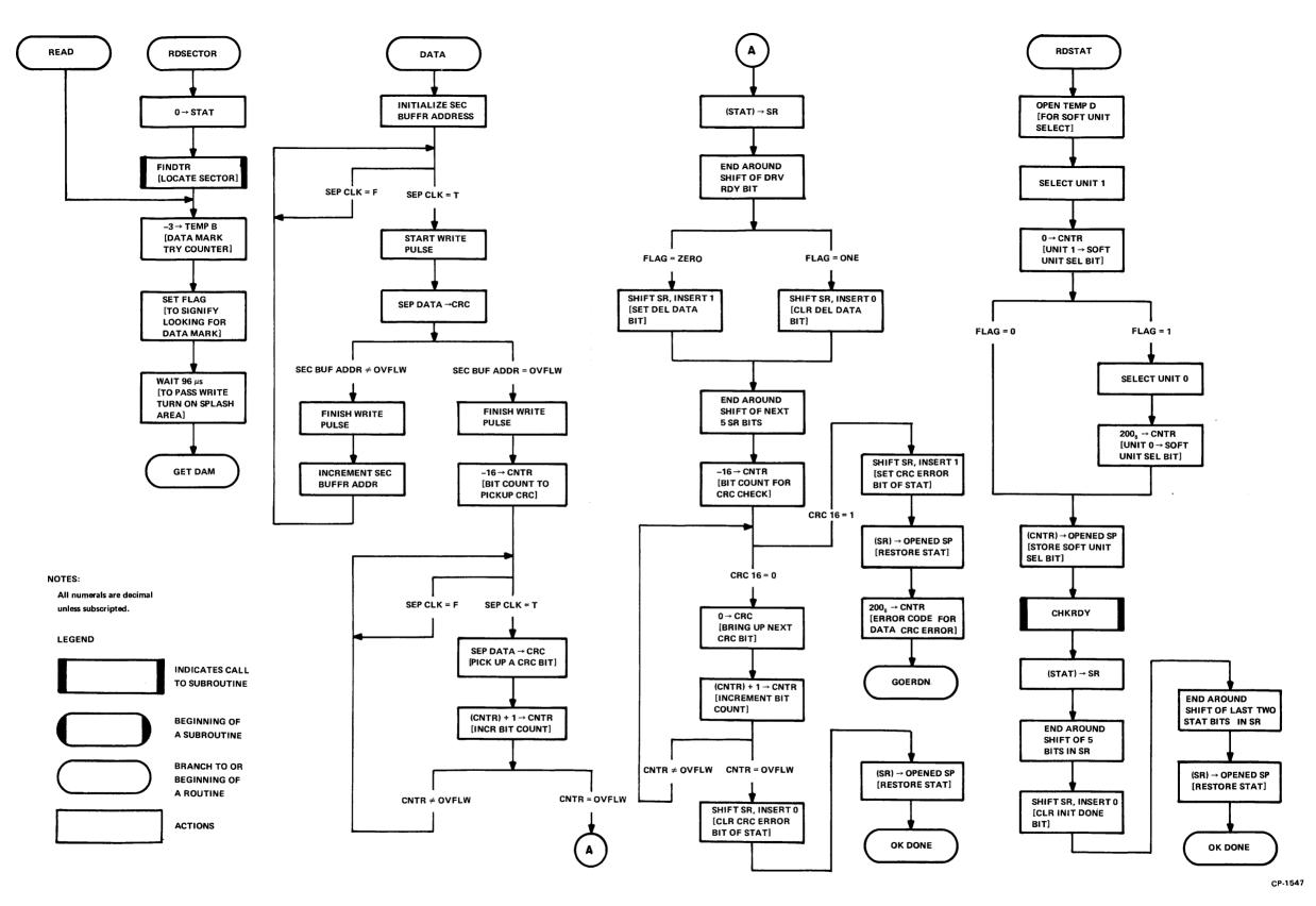
Figure 5-14 Read Sector and Read Status Functions Flowchart
