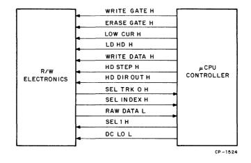
Figure 5-5 µCPU Controller to Read/Write Electronics Signals
