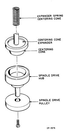
Figure 5-25 Centering Cone and Drive Hub
