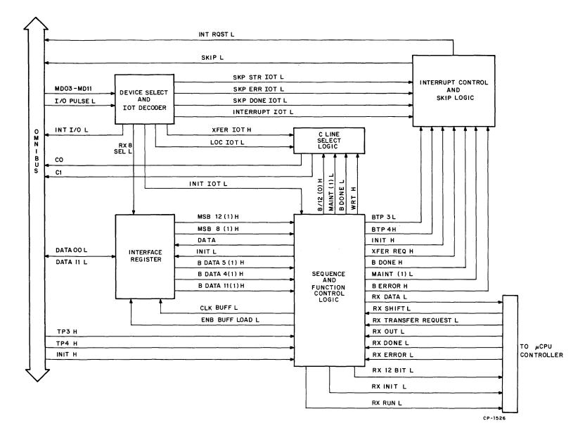
Figure 5-7 RX8E Interface Block Diagram
