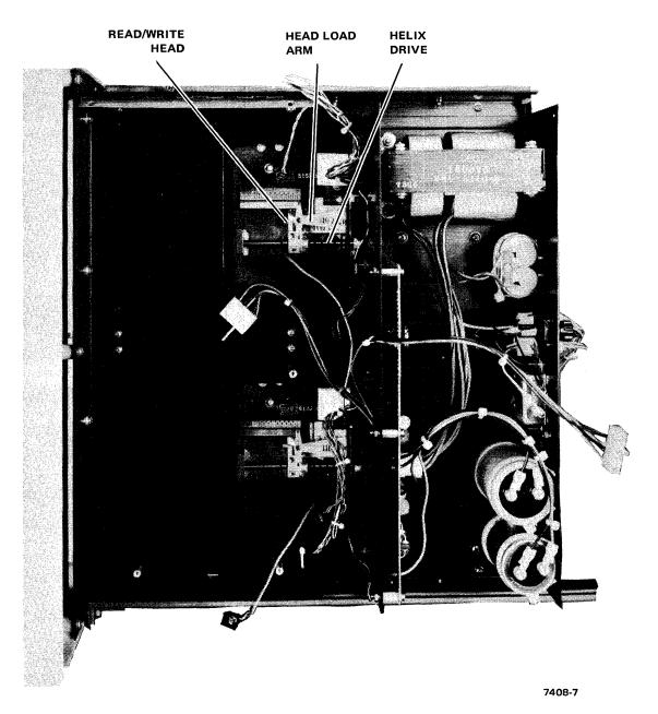
Figure 1-7 Top View of Drive
