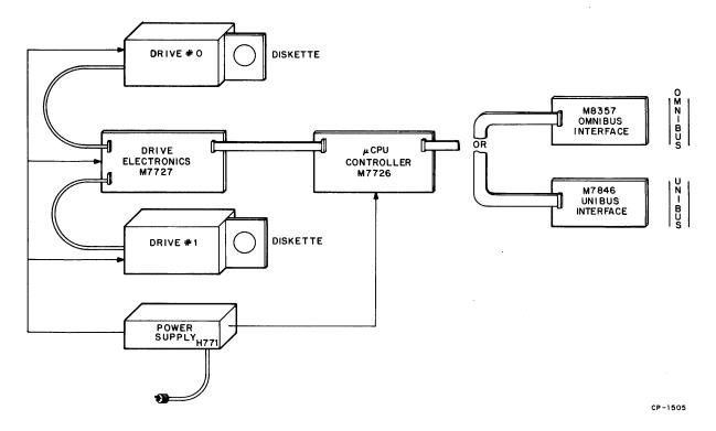
Figure 1-1 Floppy Disk System Configuration
