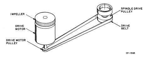
Figure 5-24 Drive Mechanism
