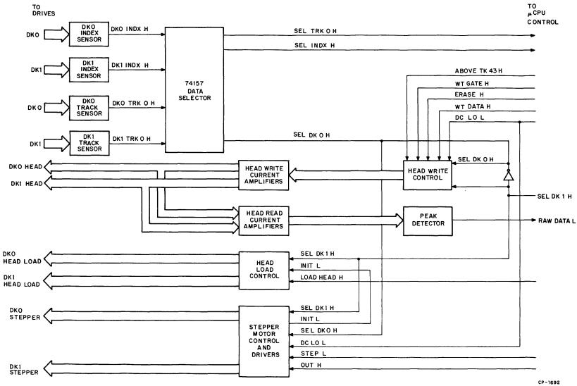
Figure 5-22 Read/Write Electronics Block Diagram
