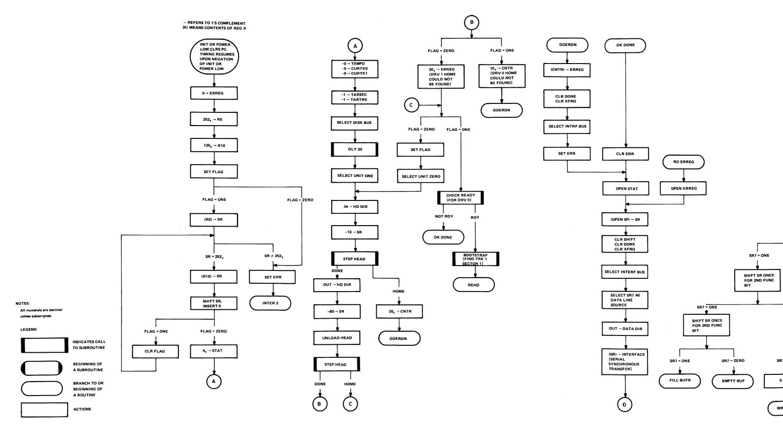
Figure 5-12 Initialize and Function Decode Flowchart
