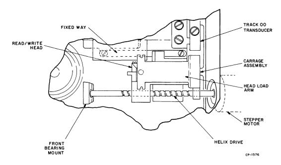
Figure 5-26 Positioning Mechanism
