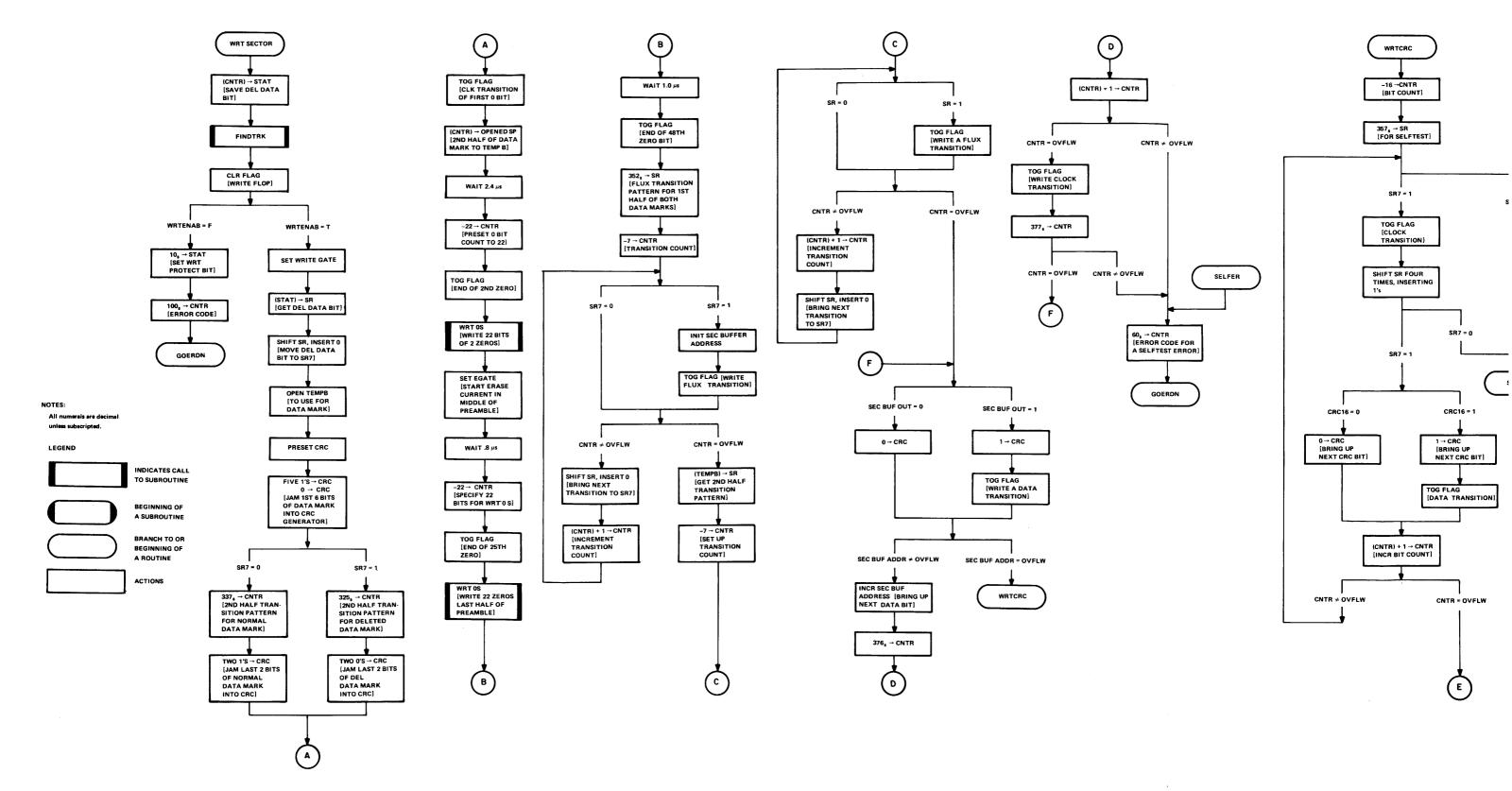
Figure 5-15 Write Sector Function Flowchart
