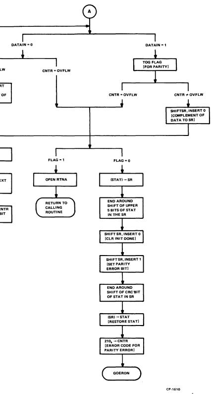
Figure 5-19 DELAY, FINDSE, WRTOS, GETWRD Subroutines Flowchart
