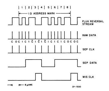
Figure 5-11 ID Address Mark Data Separation
