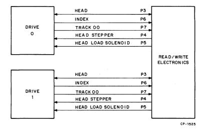
Figure 5-6 Read/Write Electronics to Drive Signals
