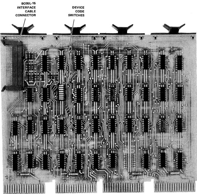
Figure 1-3 M8357 Module (RX8E Interface)
