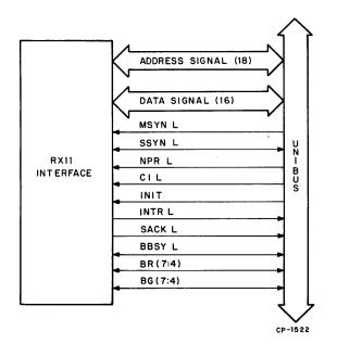
Figure 5-3 Unibus to RX11 Interface Signals
