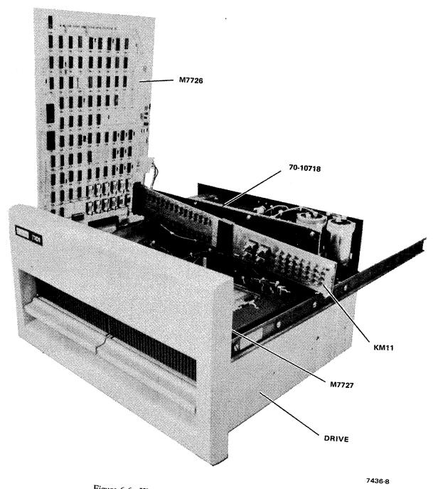
Figure 6-6 KM11 Maintenance Module Inserted
