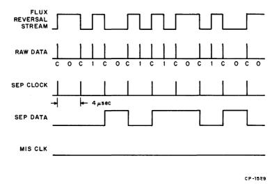
Figure 5-10 Data and Clock Separation
