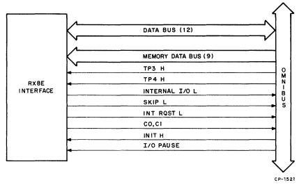
Figure 5-2 Omnibus to RX8E Interface Signals
