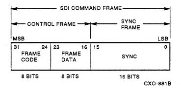
The sync frame portion is always sent first and is a special pattern used to synchronize the drive for receiving a command frame. The control frame consists of an 8-bit frame code and 8 bits of frame data.
