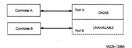
Since the drive can only communicate with one controller at a time, it must assume a "drive unavailable" state with one controller as the other controller brings it to a "drive on-line" state. When the controller which is communicating with the drive completes all of its activities and releases the drive on Port A, the drive will return to a "drive available" state relative to both ports.
