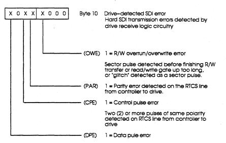
Two (2) or more pulses of same polarity detected on CMD/WRT dta line from controller to drive.
