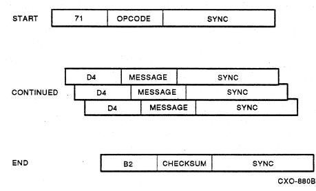
There are 16 level 2 commands. The number in parentheses indicates the number of CONTINUE frames needed to complete the command.
