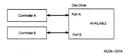
When controller A wants to communicate with the drive, it must bring it to a state called "drive on line." This means that the drive, through Port A, becomes dedicated to the exclusive use of controller A. This is illustrated in Figure 8–7. During this time, the drive is visible but not available to controller B. Its state relative to controller B is called "drive unavailable."
