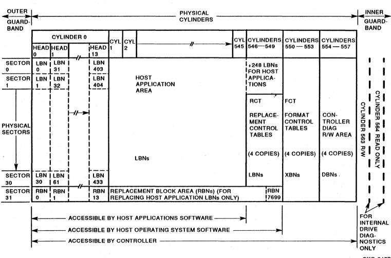
Figure 2-21: RA80 Topology - 16-Bit Format
