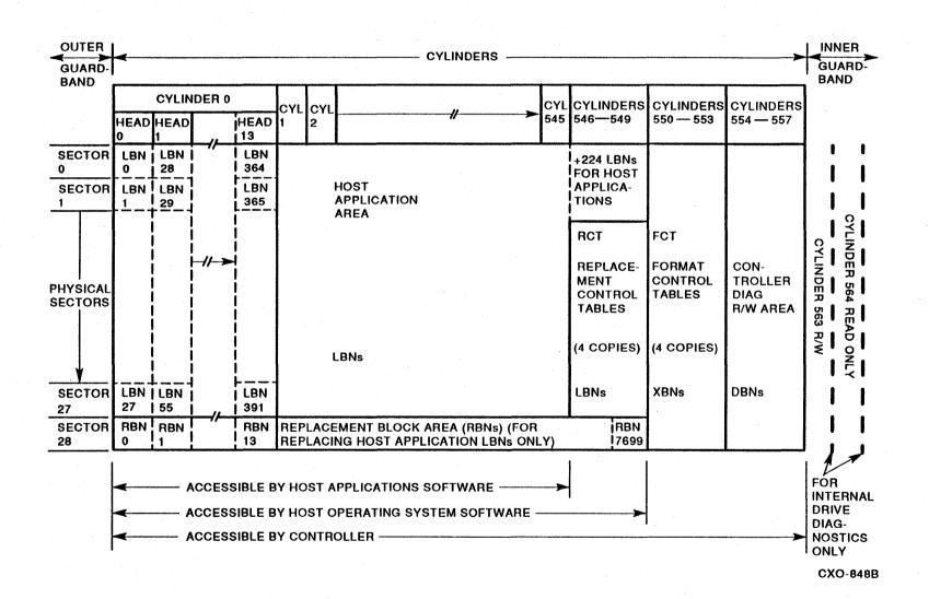
Figure 2–22: RA80 Topology – 18–Bit Format
