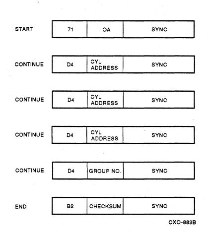
The next frames sent are CONTINUE frames, indicated by the D4 in the frame code field. The message data bytes of the CONTINUE frames contain the cylinder address and the group number for the positioning operation.
