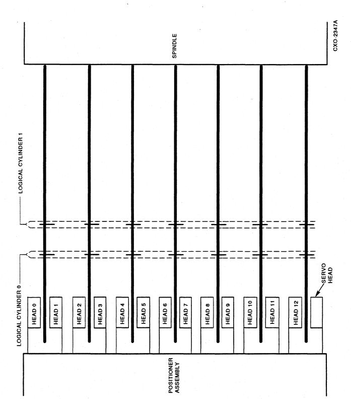
The RA90 has dedicated servo for coarse positioning. The large amount of data and cylinder densities in the RA90 require a more precise mechanism for fine positioning. Therefore, the RA90 incorporates embedded servo to accomplish a fine positioning scheme. The embedded servo exists between every sector on every track.
