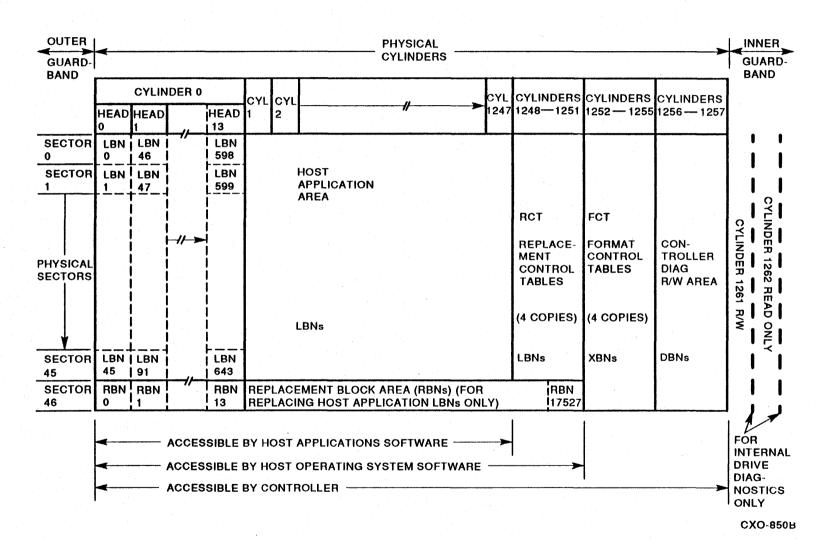
Figure 2-24: RA81 Topology - 18-Bit Format
