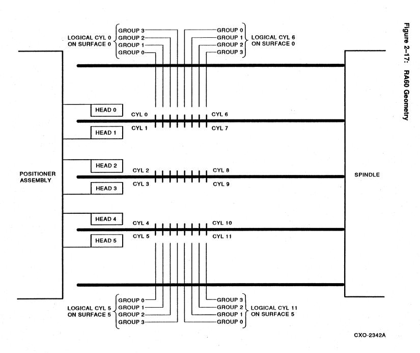
DSDF for RA60/70/80/81/82/90 Lesson 1 The RA60 does not incorporate a dedicated servo surface but relies upon embedded servo information to perform servo positioning. The embedded servo exists between every sector on every track. When performing a head switch, the RA60 servo logic must read several embedded servo bursts from a track to establish fine position before it can continue reading or writing.
