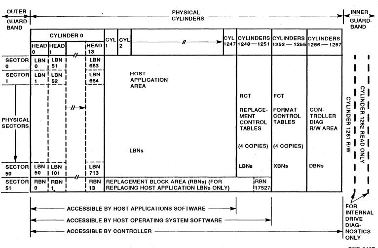
Figure 2-23: RA81 Topology – 16–Bit Format
