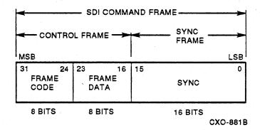
The response protocol uses the same START, CONTINUE, and END frames as the command protocol. The frame codes for the START, CONTINUE, and END frames are also identical to those used in the command frame format.
