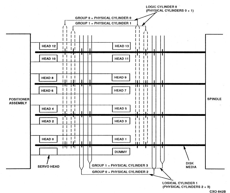
Figure 2–9: RA80 Geometry
