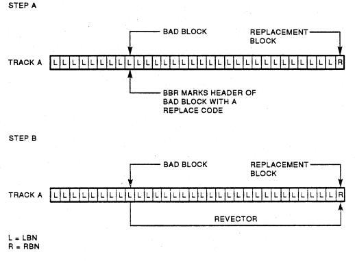
NOTE: BBR MOVES BAD BLOCK'S DATA TO REPLACEMENT BLOCK BY WRITING DATA BACK TO BAD BLOCK'S LBN. THIS CAUSES CONTROLLER TO REVECTOR DATA TO RBN.
