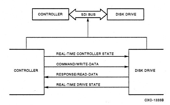
The Real Time Controller State (RTCS) line repeatedly transmits controller state information to the drive.
