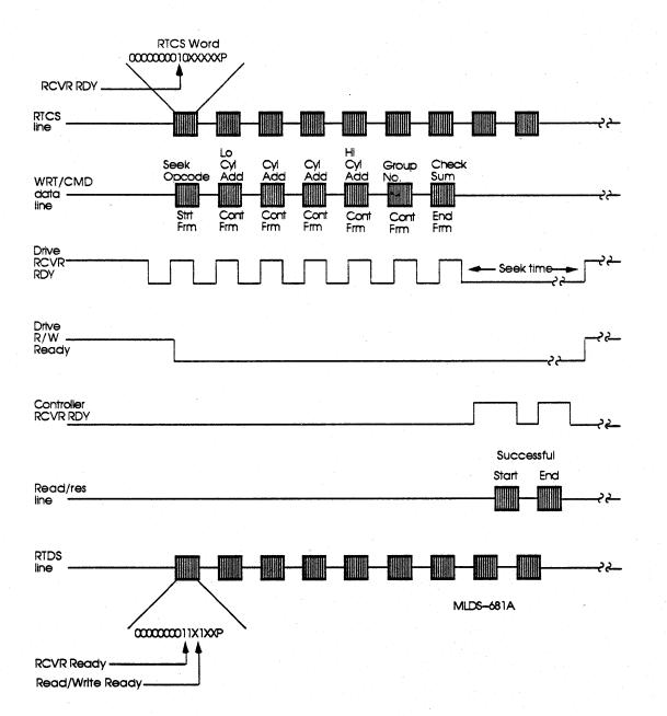
Before the controller sends the SEEK command, the drive has both R/W READY and RECEIVER READY asserted on the RTDS line. This informs the controller that it is ready to receive a command and that no data transfer is currently under way. When the drive receives the seek opcode in the start frame on the Write/Command line, both RECEIVER READY and R/W READY are cleared.
