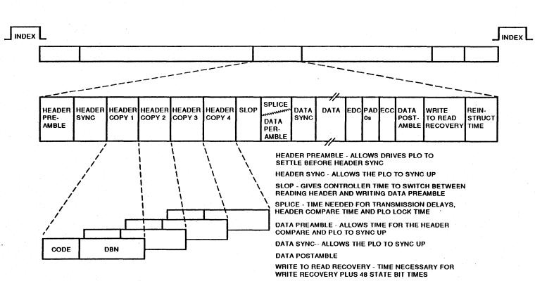
REINSTRUCT TIME - TIME ALLOTTED WHILE CONTROLLER IS CLEANING UP CURRENT SECTOR TRANSFER AND SENDING
