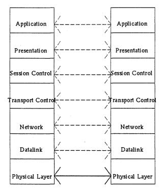
In classic communications architectures there are two types of transports—those built upon datagram services and those built upon virtual circuits. Datagram services force the higher-level protocols to be resilient in ensuring message receipt from end-to-end. Virtual circuit transports exhibit flow control and guarantee delivery of messages (in order) to the higher layers.
