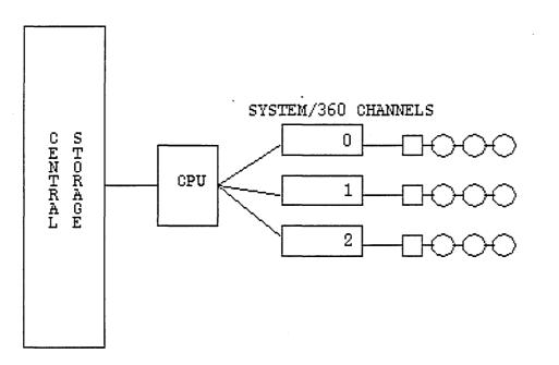
Figure 1–1: System/360 Channel Architecture
