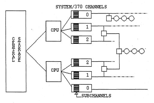
The channel-to-I/O device interface is single path oriented in another way. Once a chain of I/O operations is initiated with a device, all data, status, and commands for the chain of operations must use the physical channel path over which the first command was initiated (*IBM1*). In particular, if a device disconnects from the channel path during a chain of commands, as when block multiplexing occurs, the device must reconnect to the same path to continue
