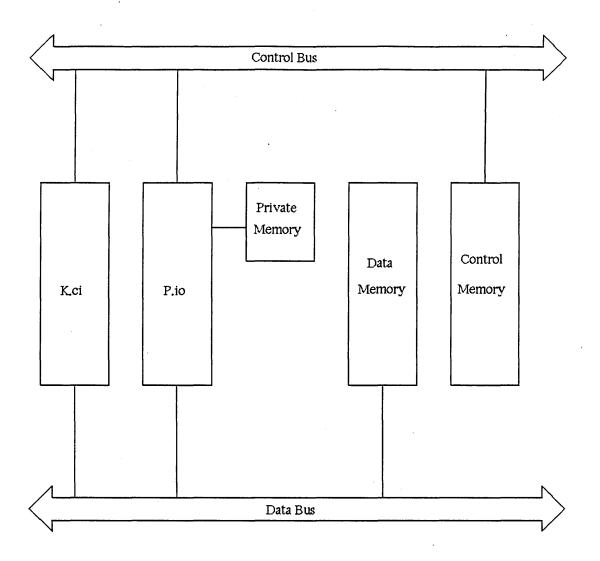
Each of the K's use 2901 bit slices as pictured in Figure 2–9. The upper processor's primary role is accepting requests from the P.io software, while the lower processor's purpose is to move data memory across the data bus. The upper processor cannot interface with the data bus, nor can the lower processor interface with the control bus. The upper and lower processors communicate through the shared "scratchpad" memory that is onboard.
