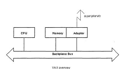
The register transfer level of the VAX is a Complex Instruction Set Computer (CISC) with a fairly orthogonal instruction set. There are 16 General Purpose Registers (GPR); however, the last four are used for stack control and program counter. There is also a Processor Long Word (PSL) that holds the current state of the processor.
