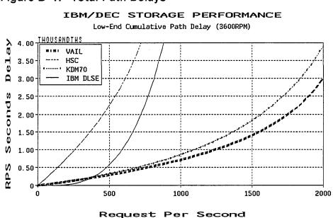
Figure B-1: Total Path Delays
