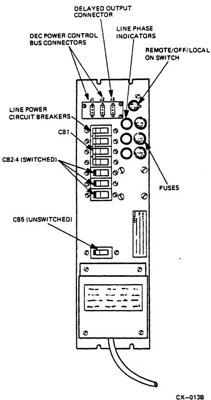
HSC50 AC Power Controller (120/208 Vac) -- Front View
