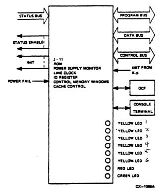
Input/Output Control Processor Module (HSC70)
