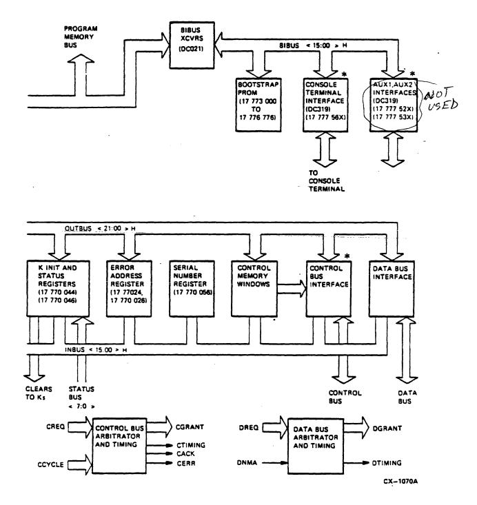
HSC70 Input/Output Control Processor Module Block Diagram (Sheet 2 of 2)
