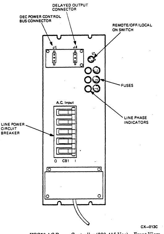
HSC50 AC Power Controller (380-415 Vac) -- Front View
