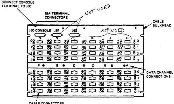
CABLE CONNECTORS WITHIN A DATA CHANNEL
