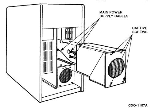
16. Turn the four captive screws on the front of the power supply counterclockwise (Figure 3-47).
