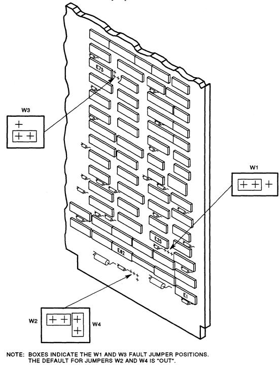
Figure 3-14 shows the LINK (L0118-B1) jumpers.
