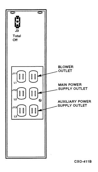
Figure 2–17 HSC50 Power Controller (50 Hz)—Rear View
