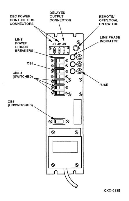
Figure 2–14 HSC50 Power Controller (60 Hz)—Front View
