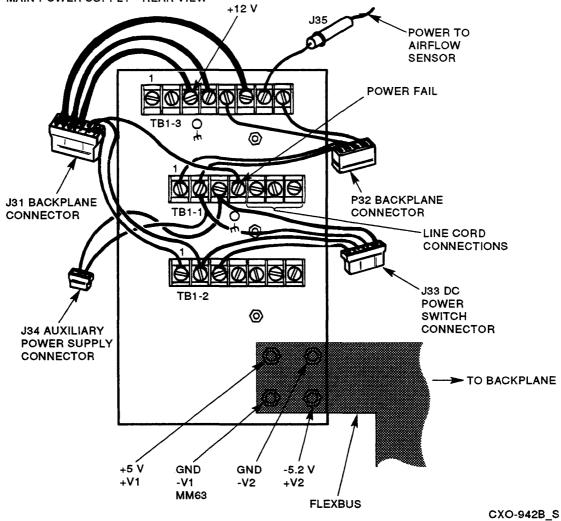
Figure 3–46 HSC Main Power Supply Cables and Test Points
