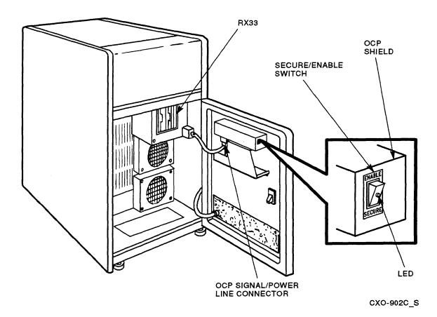
Figure 2–2 Controls/Indicators Inside Front Door
