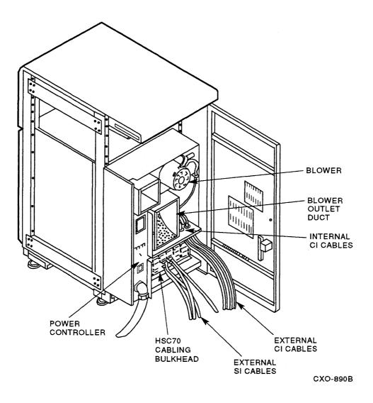
Figure 1--5 HSC Cabinet Inside Rear View
