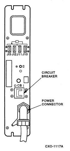
Figure 3–32 881 Power Controller Circuit Breaker
