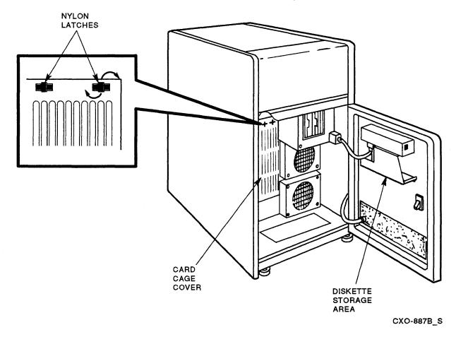
Figure 3–9 HSC Card Cage Cover Removal
