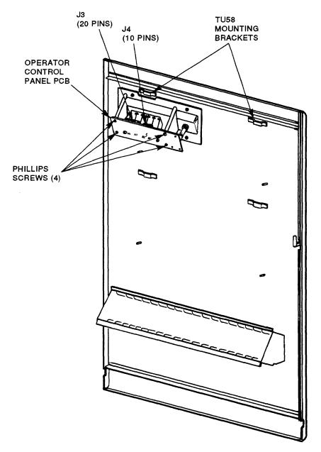
8. Support the bezel assembly with one hand and disconnect J3 and J4 from the OCP (Figure 3-27).
