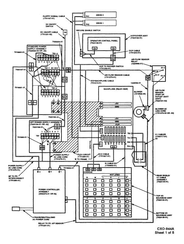
Figure A-1 (Cont.) HSC Internal Cabling
