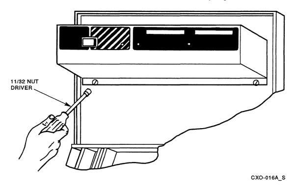
5. Remove the two locknuts on the bottom of the TU58 bezel assembly (Figure 3-26).
