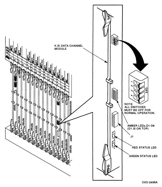
Figure 2–11 K.si Module (L0119-YA) Switches
