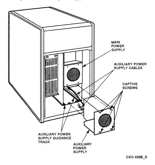
11. Turn the four captive screws on the power supply counterclockwise (Figure 3-56).
