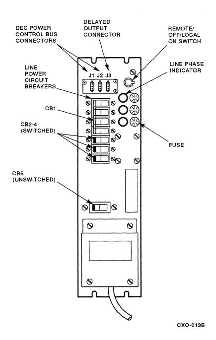
Figure 3–4 HSC50 Line Power Circuit Breakers
