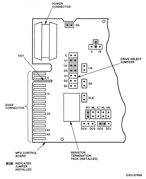
Figure 3-24 shows the jumper locations for RX33 with a revision A3 module.
