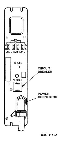
Figure 3–2 HSC 881 Power Controller Circuit Breaker
