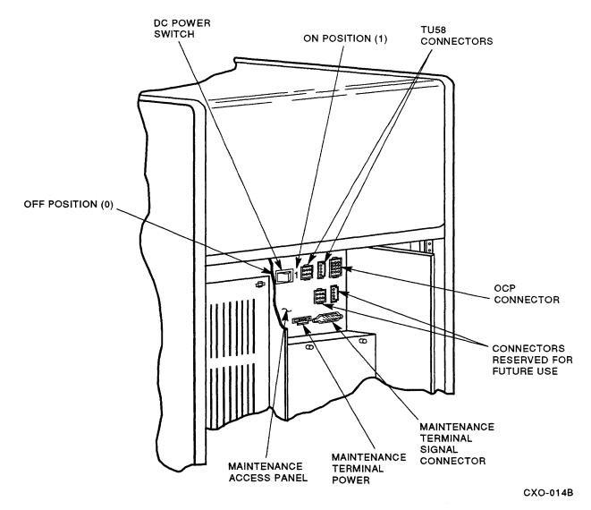
Figure 2–5 HSC50 Maintenance Access Panel
