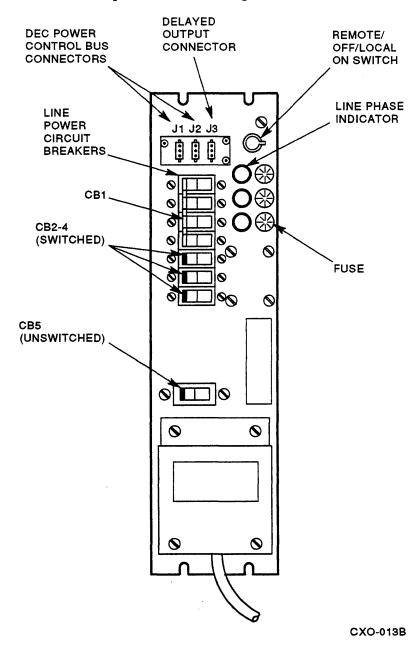
Figure 3–43 HSC50 Power Controller Circuit Breaker
