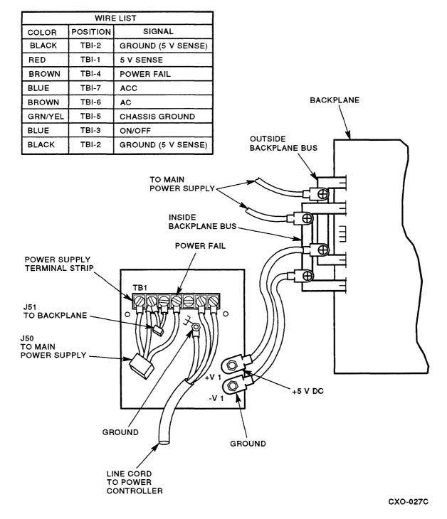
Figure 3–55 HSC50 Auxiliary Power Supply Cable and Voltage Test Points
