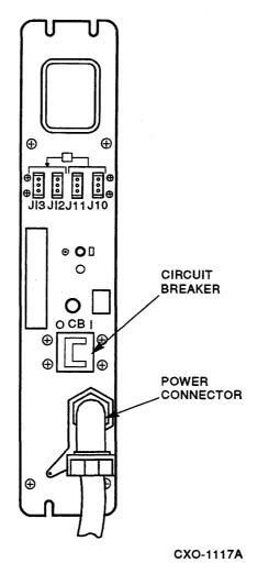
Figure 3–36 881 Power Controller Circuit Breaker
