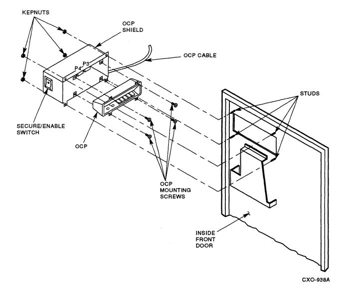
Figure 3–30 Removing the HSC OCP
