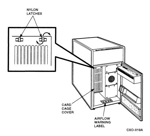
Figure 3–10 HSC50 Card Cage Cover Removal
