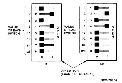
Figure 3–11 L0100 Node Address Switches
