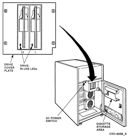
Figure 2–3 RX33 and dc Power Switch
