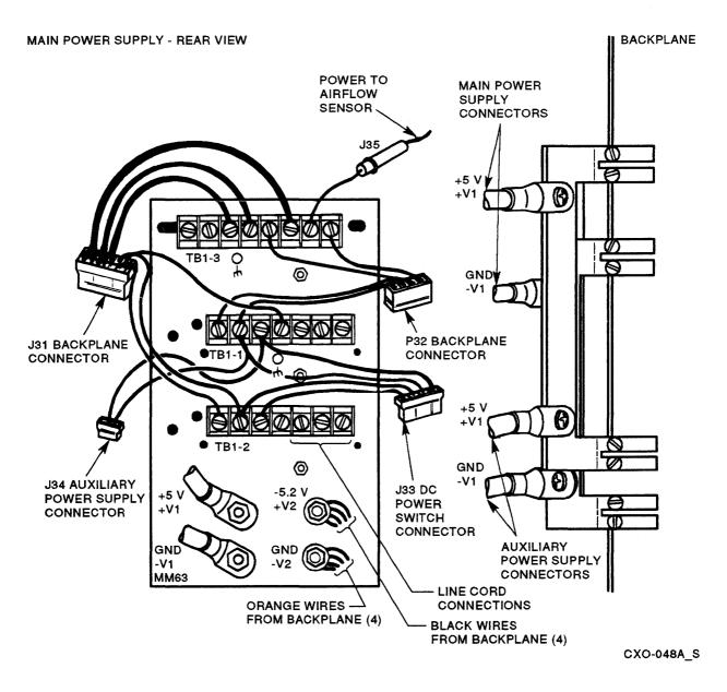
Figure 3–49 HSC50 Main Power Supply Cables and Voltage Test Points
