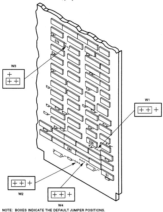
Figure 3–15 shows the LINK (L0118-B2) jumpers.
