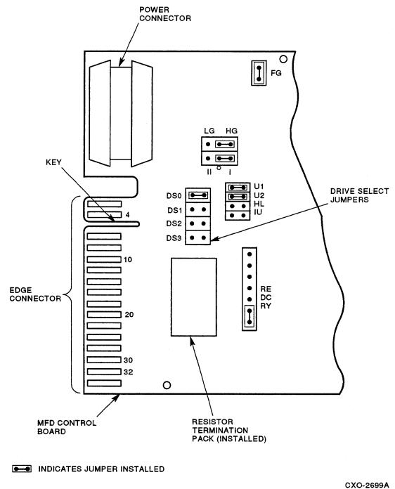
Figure 3-23 shows the jumper locations for RX33 with a revision A1 module.
