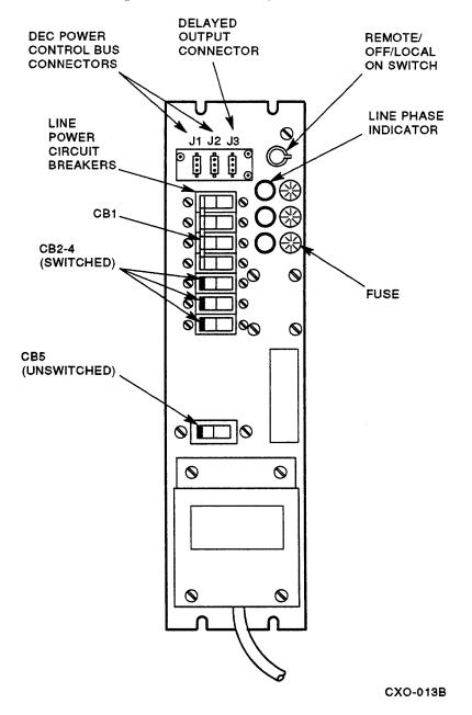
Figure 3–38 HSC50 Power Controller Circuit Breaker
