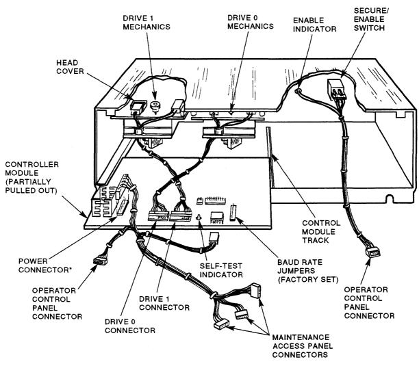
9. Disconnect the cables from the TU58 controller module (Figure 3-28).
