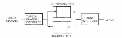
(b) TURBOchannel I/O Module
