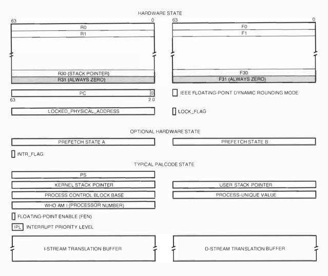
Figure 2 Per-processor State
