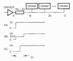
Series termination results in a half-amplitude signal at the first RAM on the line until the signal reflects from point C  $_{\rm e}$
