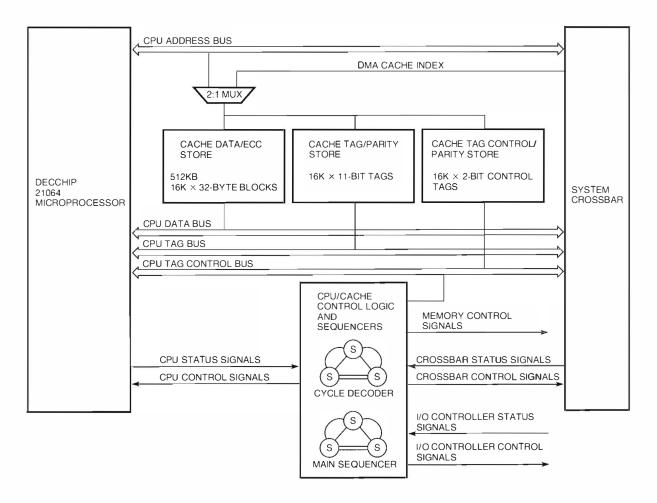
Figure 4 CPU and B-cache Block Diagram
