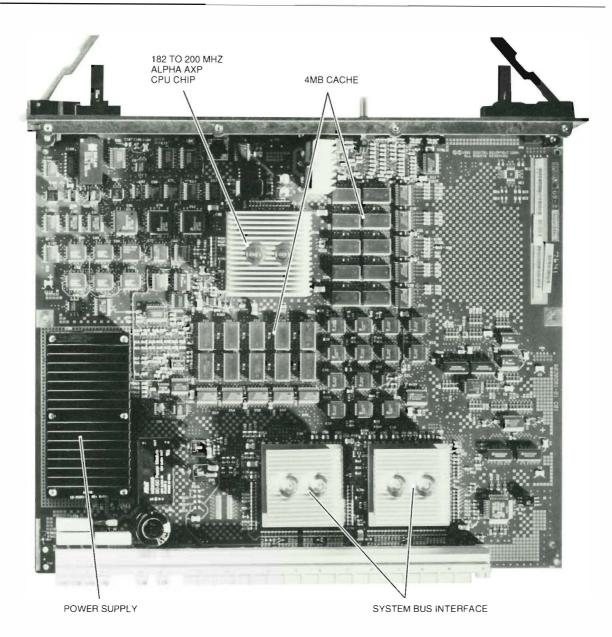
Figure 5 Processor Module, Major Components Highlighted
