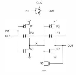
(c) Noninverting Active-low Latch
