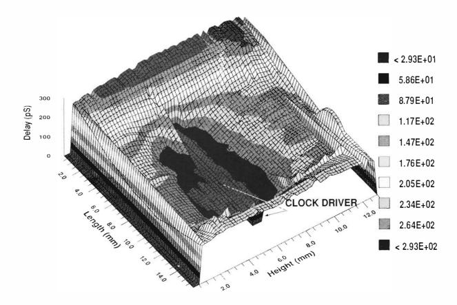
Figure 7 CPU Clock Skew
