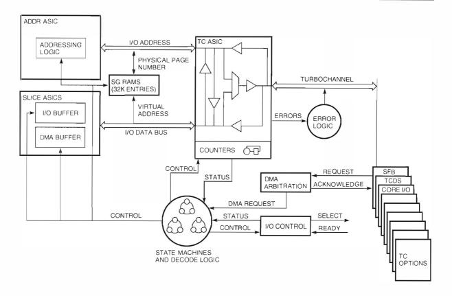
Figure 6 TURBOchannel Interface Block Diagram
