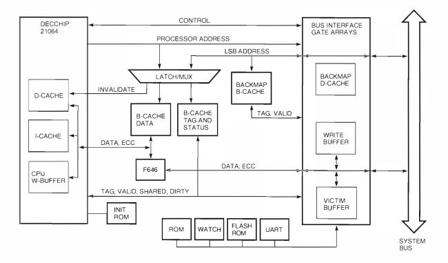
Figure 3 Block Diagram of the DEC 7000 Processor Module
