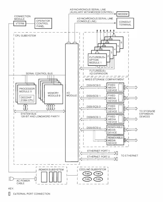
Figure 2 DEC 4000 AXP System Functional Partition
