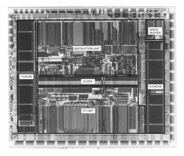
Figure 2 Microphotograph of Chip
