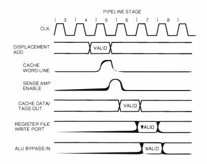
Figure 15 D-cache Timing Diagram
