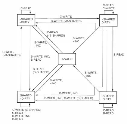
Transitions occur as a result of CPU reads and writes (C-read, C-write) and bus operations initiated by other caches or I/O controllers (B-read, B-write). A C-read or C-write to an invalid block causes a B-read; a C-write to a shared block causes a B-write. The B-shared response indicates that some other cache contains the block. INC indicates that the block is in the CPU's on-chip cache.
