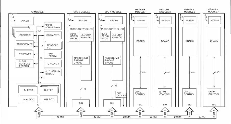
Figure 3 DEC 4000 AXP System Bus
