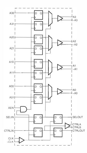
Figure 9 Address and Control Driver
