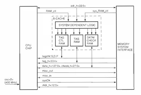
Figure 4 CPU External Interface
