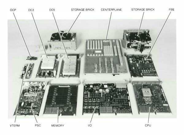
Figure 7 DEC 4000 AXP Modular Electronics
