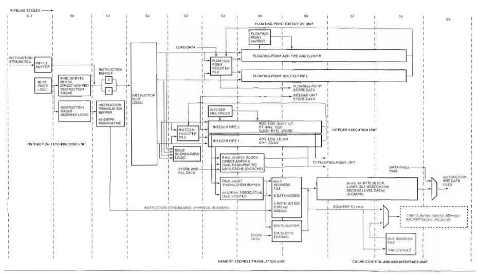
**Figure 1**Five Functional Units on the Alpha 21164 Microprocessor
