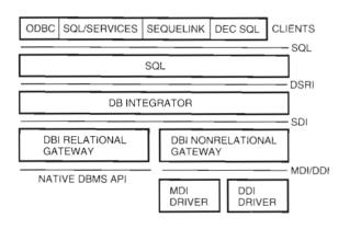
**Figure 5**DB Integrator Architecture
