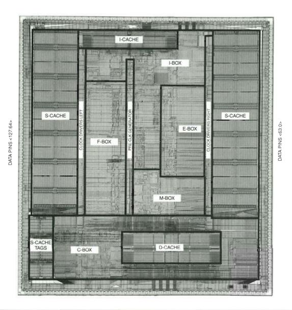
Figure 2 Floorplan of the Alpha 21164 Chip
