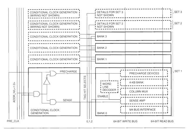
**Figure 10**Schematic of Right Half of L2 Cache Data Arrays
