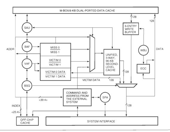
**Figure 5** Functional Units of the C-box
