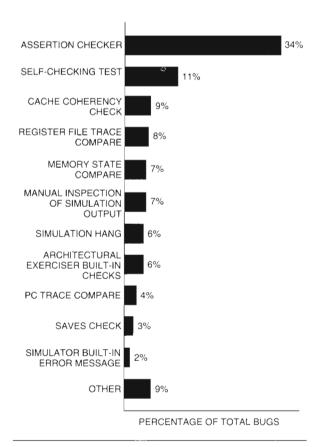
**Figure 5** Effectiveness of Bug Detection Mechanisms
