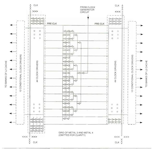
**Figure 3** Schematic of Clock Distribution System
