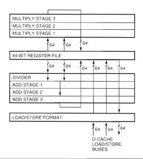
**Figure 3** Physical Layout of the Floating-point Unit
