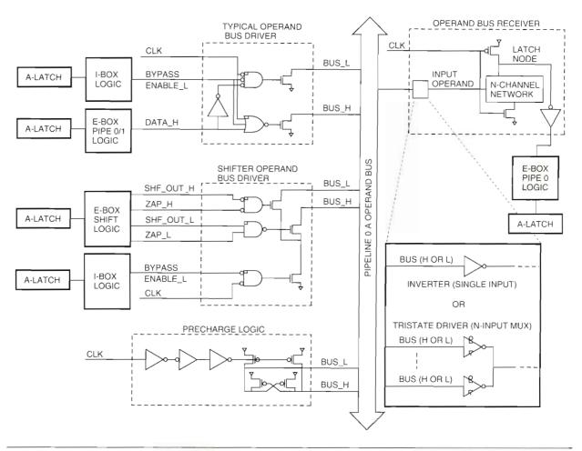
Figure 9 E-box Bypass Bus
