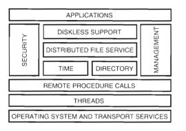
**Figure 2**OSF's Distributed Computing Environment
