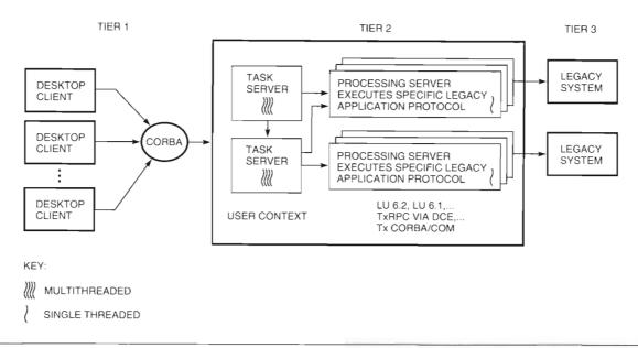
**Figure 4**Overall Three-tier Client-Server Architecture
