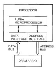
Figure 2 Simple Uniprocessor System Topology
