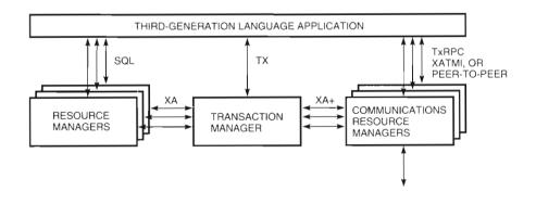
**Figure 3** X/Open Distributed Transaction Processing Model
