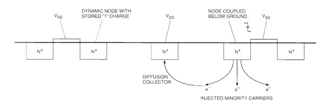
**Figure 13** Dynamic Node Protected from Minority Carrier Injection
