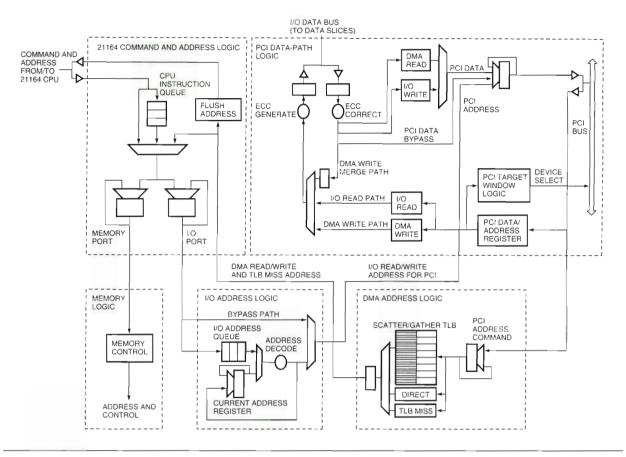
Figure 3 Control Chip Block Diagram
