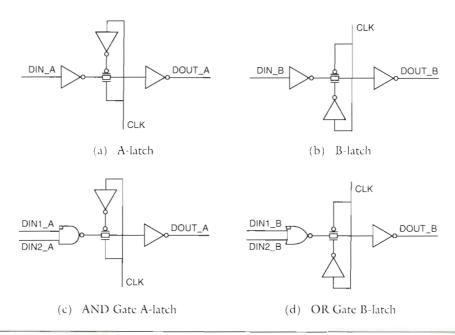
Figure 6 Alpha 21164 Standard Latch Examples
