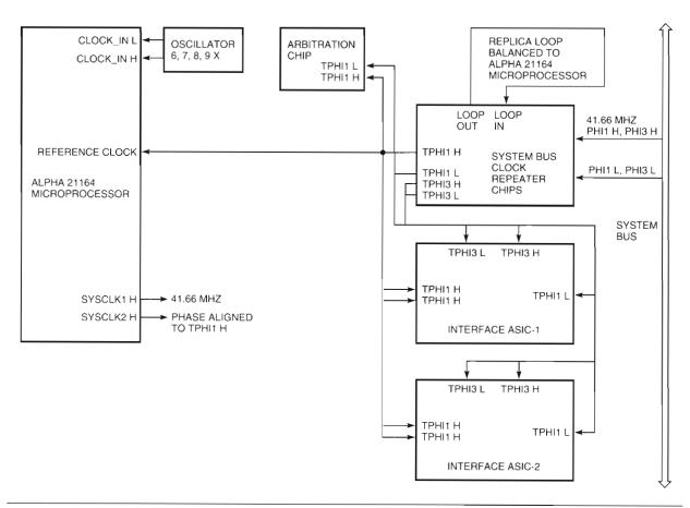
**Figure 2** KN470 Clocking Scheme
