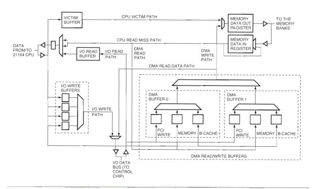
Figure 2 Data Slice Block Diagram
