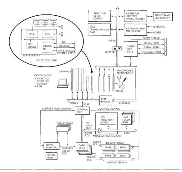
**Figure 1** AlphaStation 600 5-series Workstation Block Diagram
