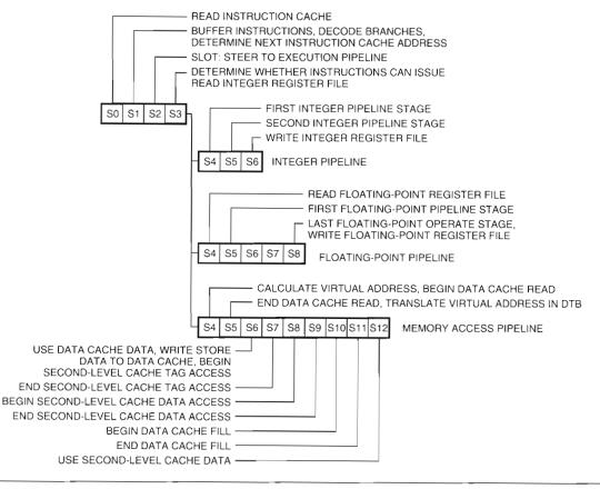
**Figure 2** Alpha 21164 Pipeline Stages
