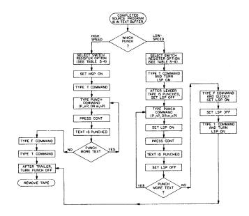
Figure 5-4 Generating a Symbolic Tape Using the Editor
