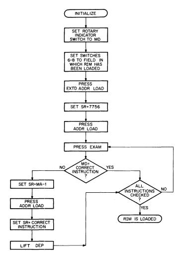
Figure 4-9 Checking the RIM Loader
