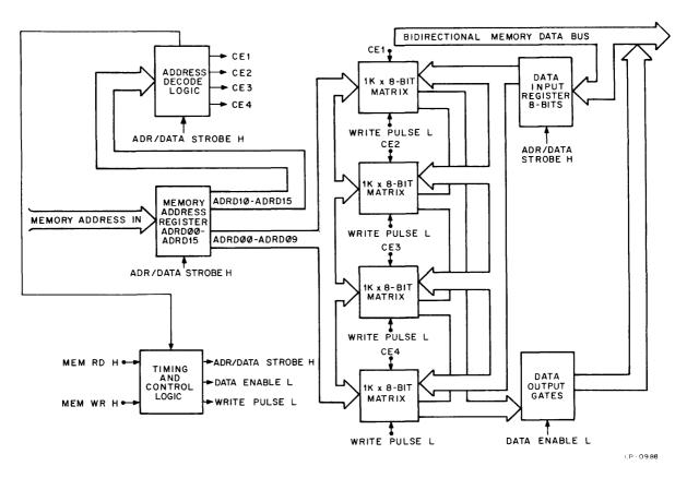
Figure 2-5 M7344 Block Diagram
