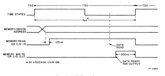
Figure 2-4 I/O Timing Diagram
