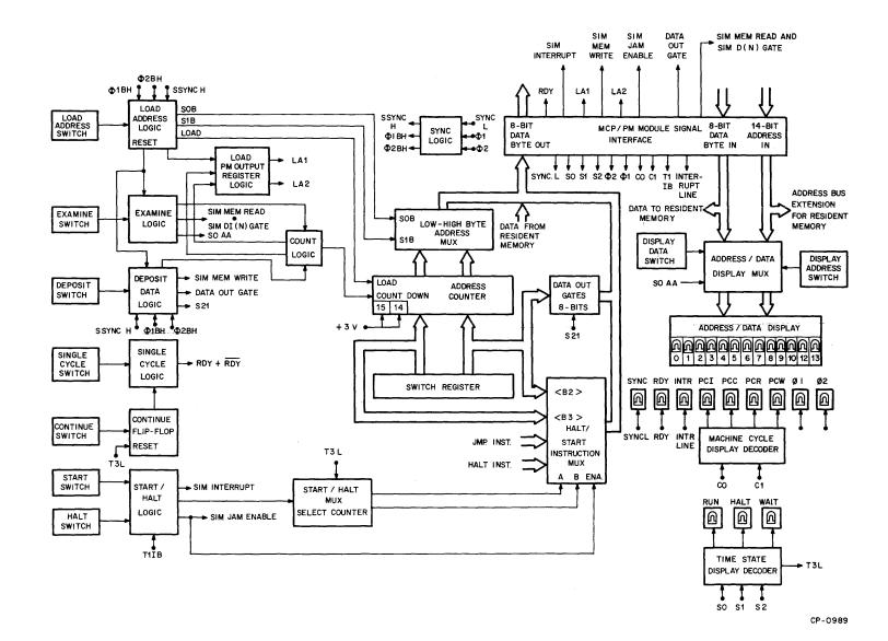
Figure 2-13 MCP Block Diagram
