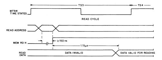
Figure 2-9 Memory Timing Diagram
