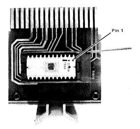
Figure 9-3 Y168 Socket Module (with PROM inserted)
