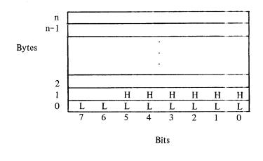
Bit 5 of byte 1 above is therefore the most significant bit of the 14-bit address stored in bytes 0 and 1, as shown below:
