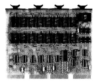
Figure 1-3 Programmable Read-Only Module
