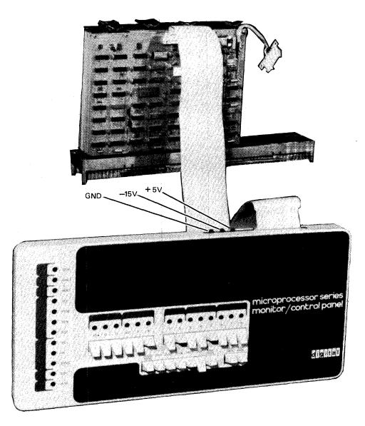
Figure 2-11 MCP Cable Connections
