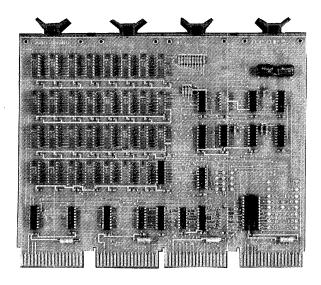
Figure 1-2 Read/Write Module
