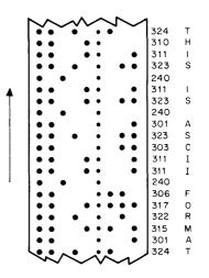
Figure 4-4 ASCII Format
