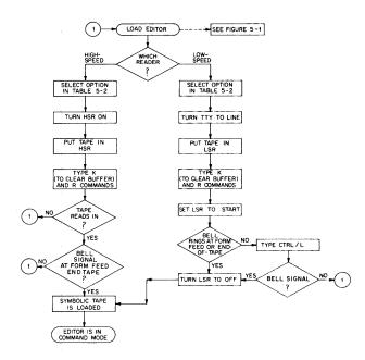
Figure 5-3 Loading a Symbolic Tape Using the Editor
