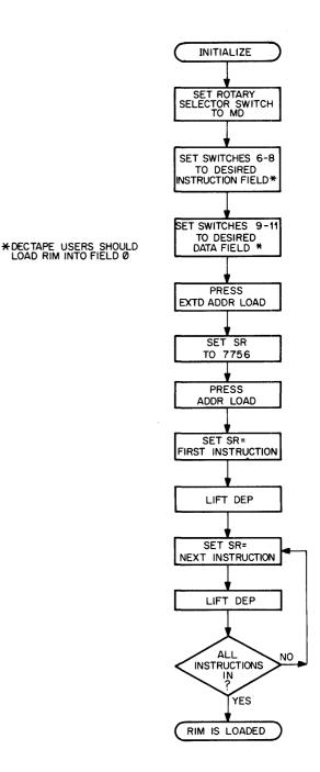
Figure 4-8 Loading the RIM Loader
