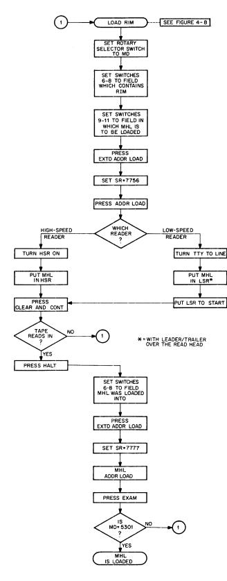
Figure 4-10 Loading the Microprocessor Host Loader
