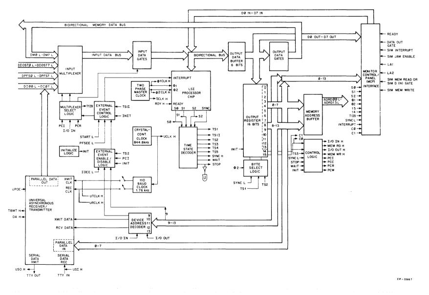
Figure 2-1 PM Block Diagram
