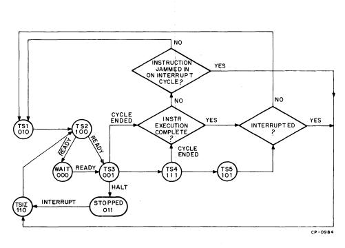
Figure 2-3 Time State Flow Diagram
