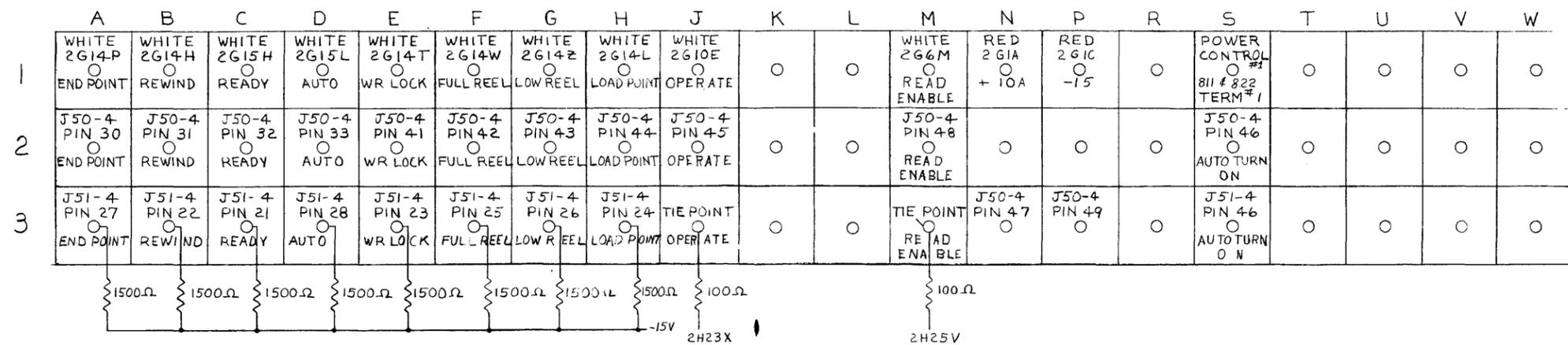
NOTE: ALL RESISTORS ARE LOCATED ON TERMINAL BOARDS ON FACE OF CONTROL 51 LOGIC
