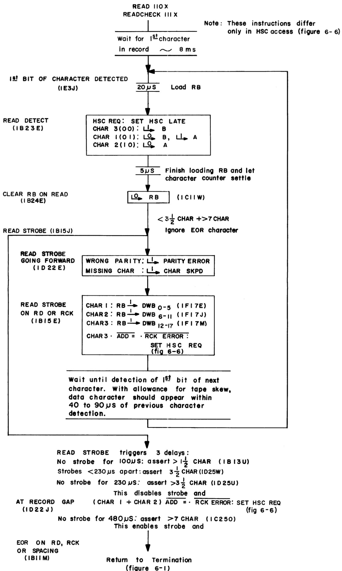
Figure 6-3 Flow Chart: Read and Readcheck
