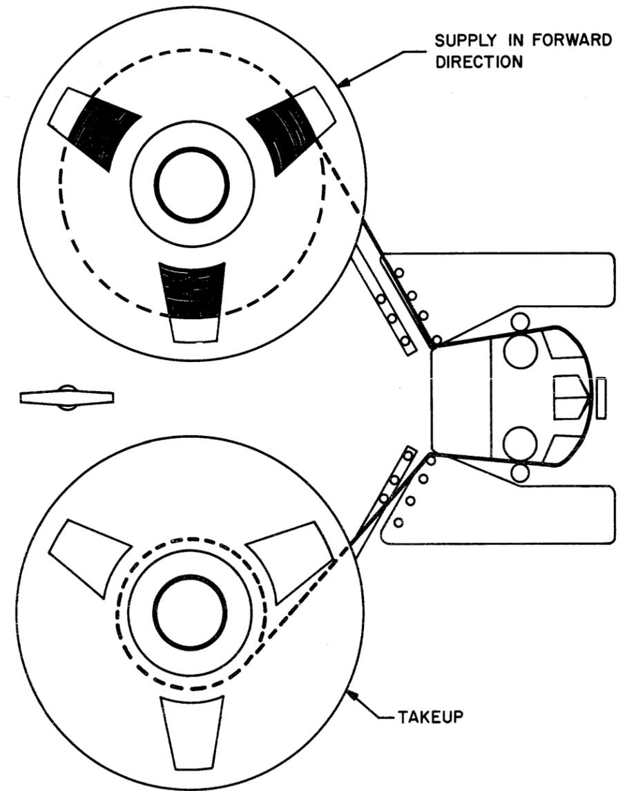
Figure 5-5 Tape Threading
