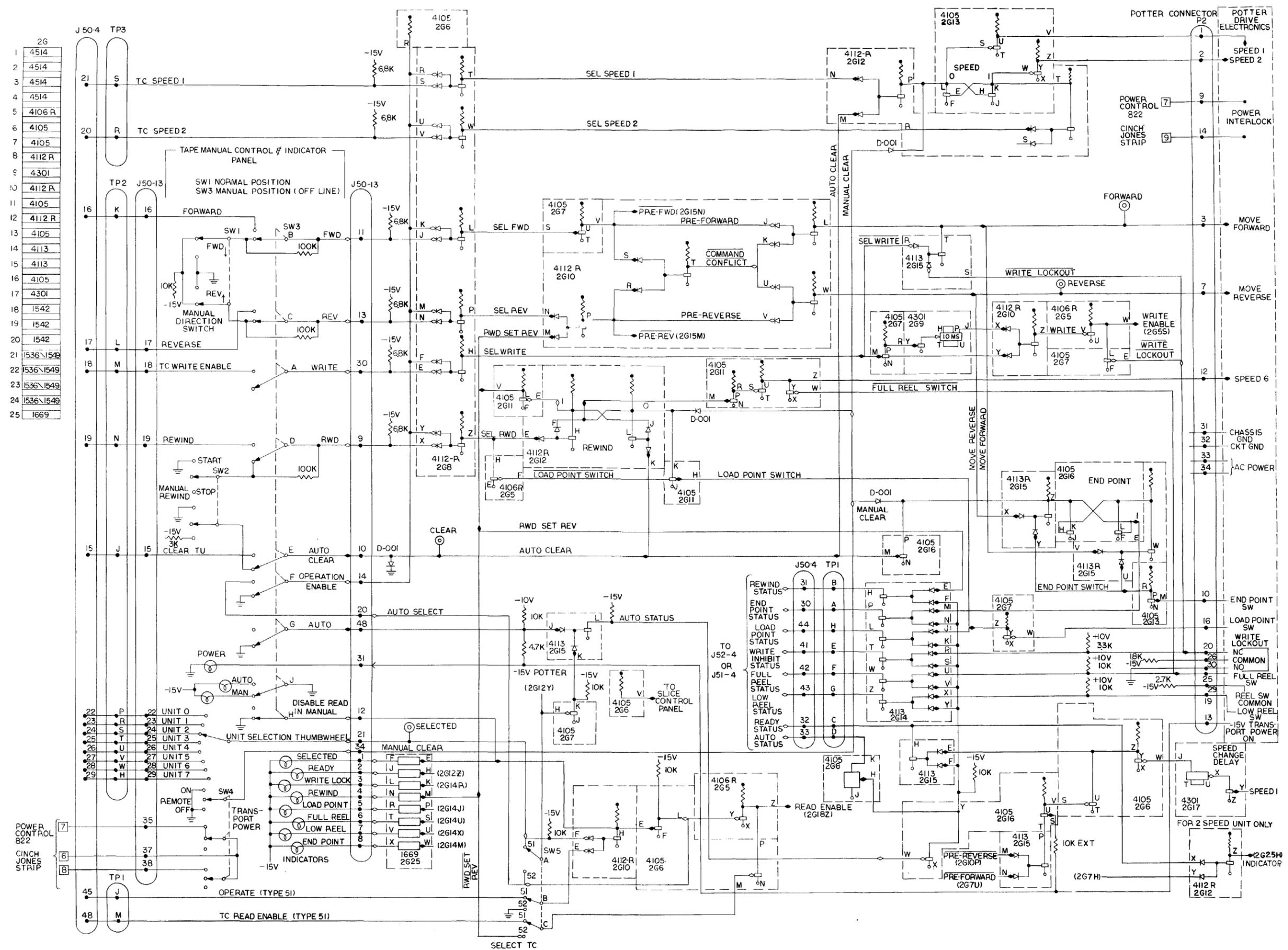
Figure 6-18 Tape Unit 50: Transport Logic
