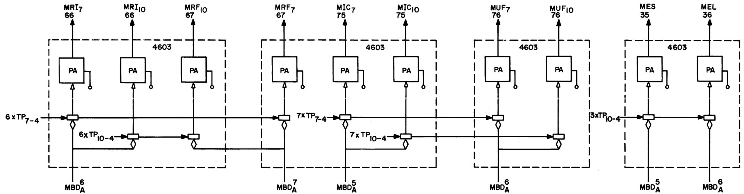
Figure 6-7 IOT Control for Type 52 Tape System
