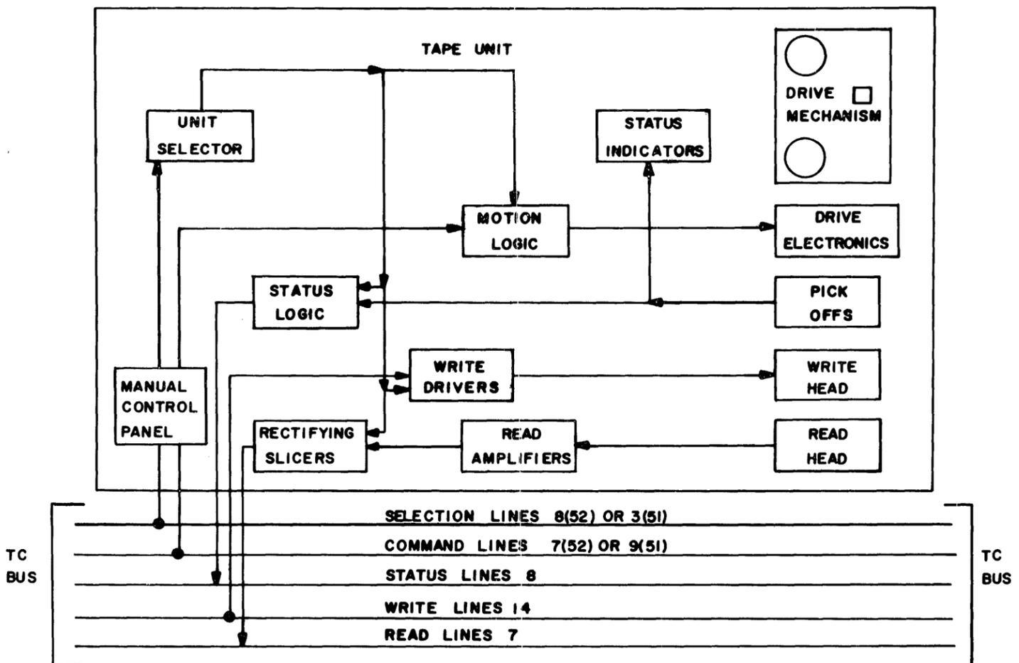
Figure 4-5 Tape Unit 50 Block Diagram
