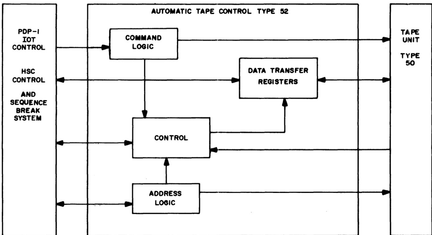
Figure 4-1 Automatic Tape System Block Diagram
