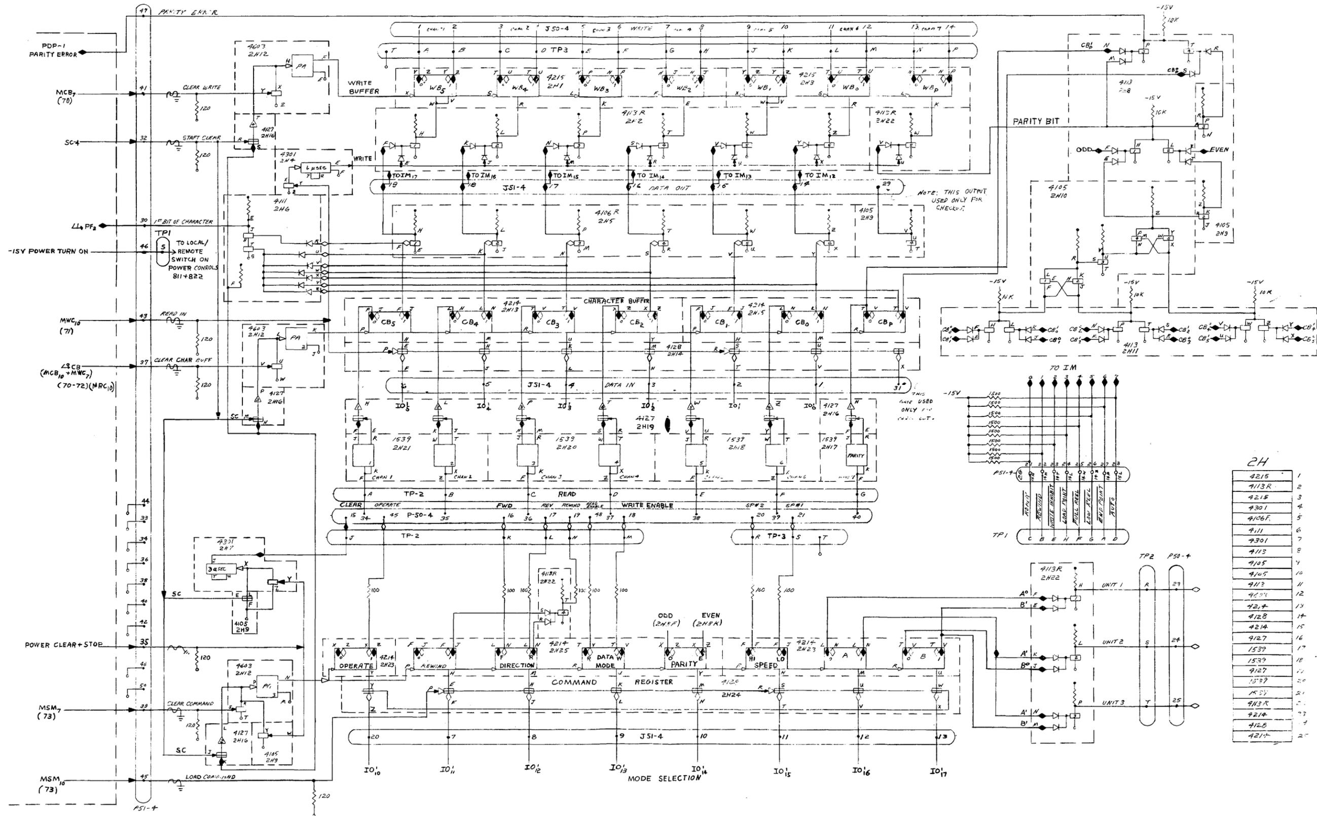
Figure 6-17 Programmed Tape Control Type 51
