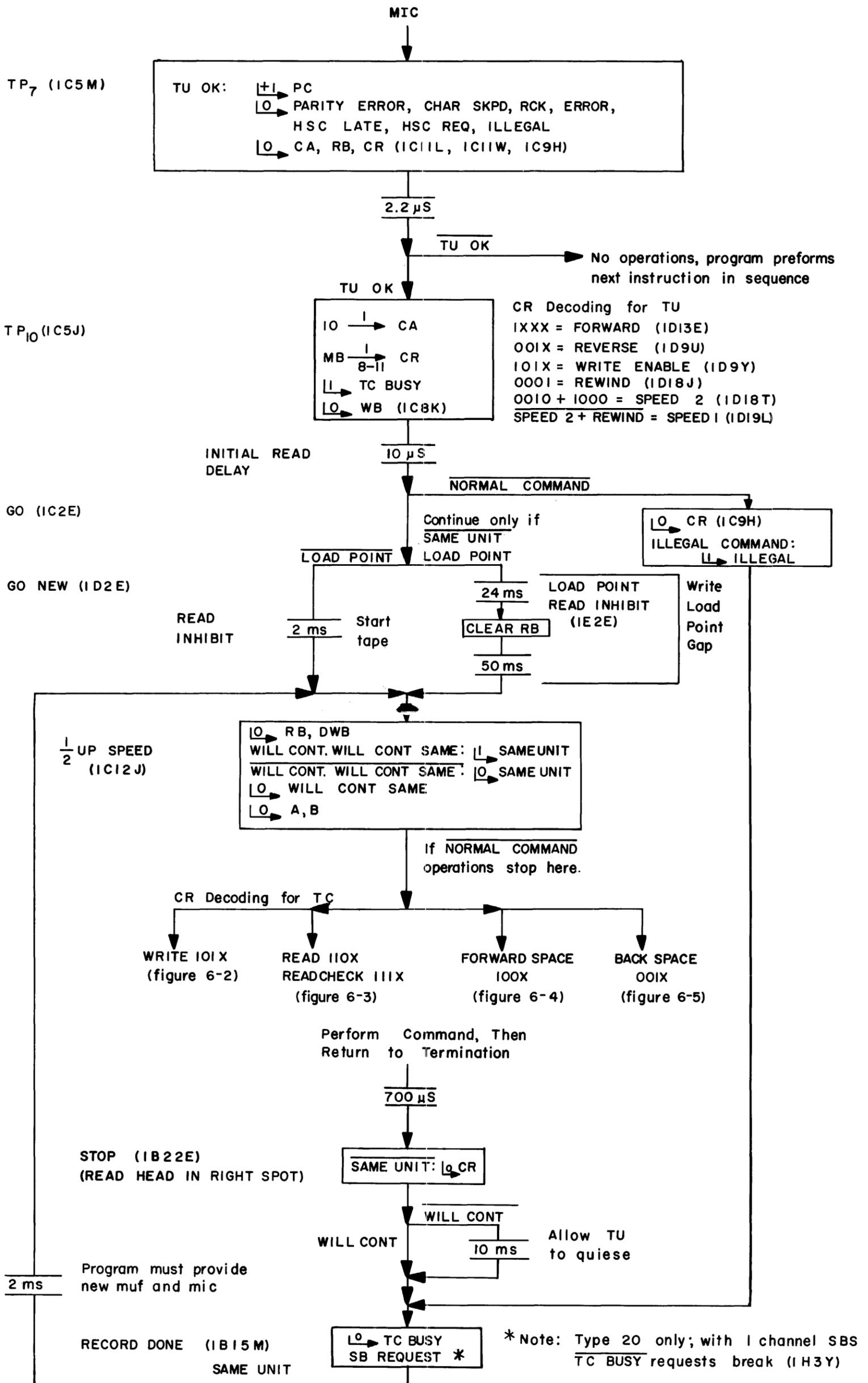
Figure 6-1 Flow Chart: Initiation and Termination of Tape Commands
