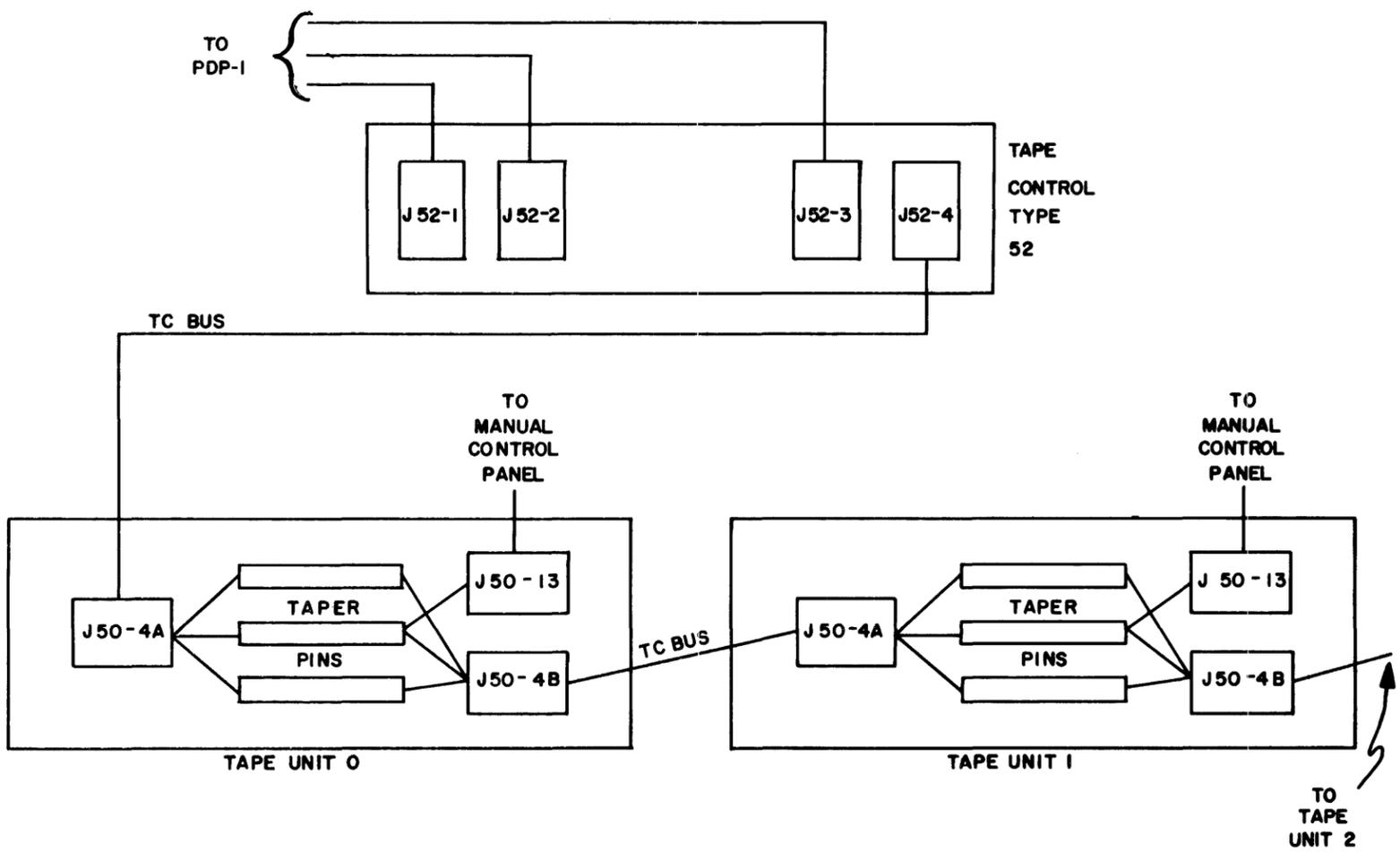
Figure 3-2 Type 52 System Bus Connections
