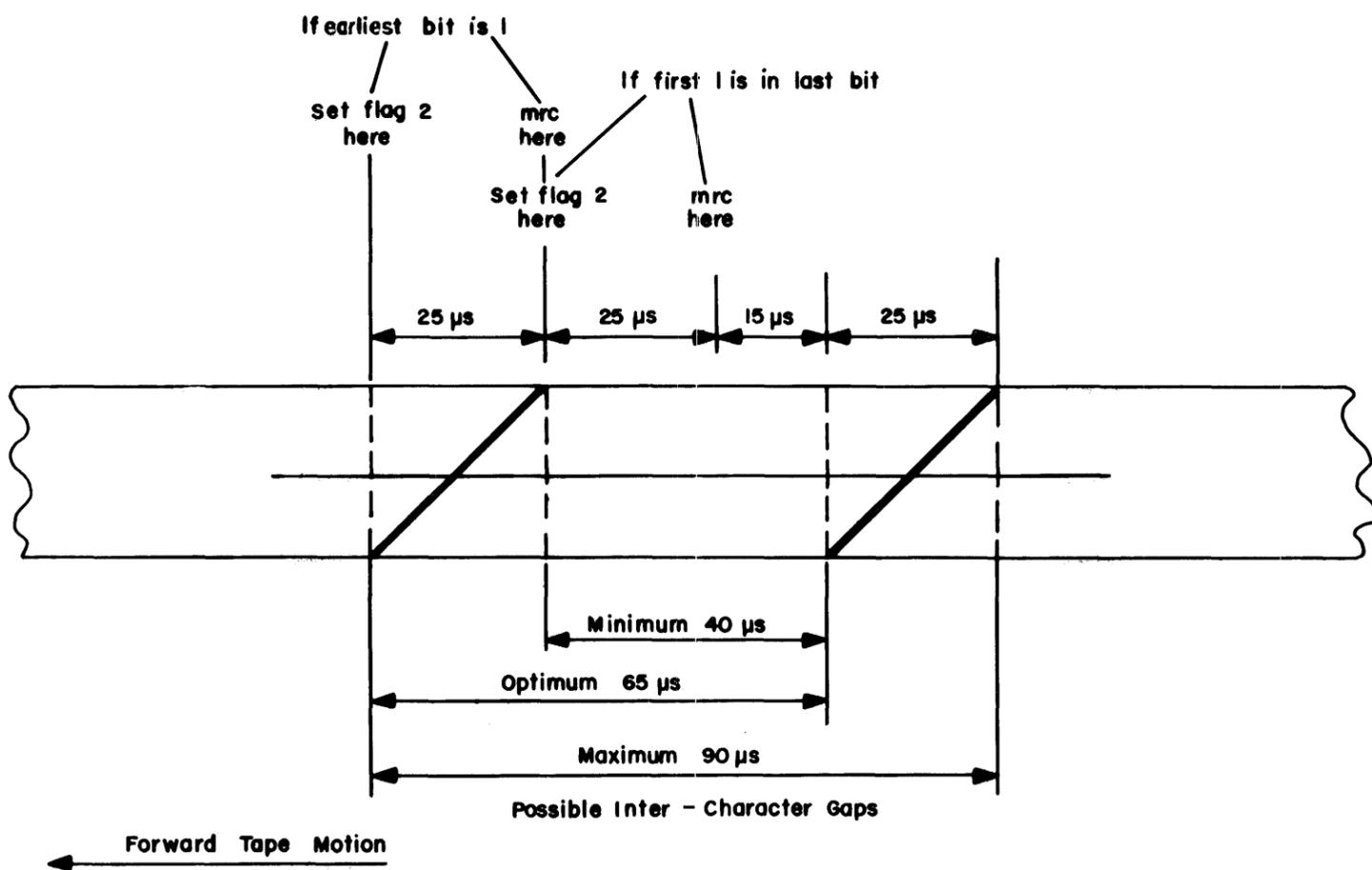
Figure 4-6 Read Timing for Type 51 Programmed Tape System
