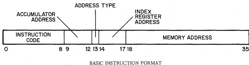
An input/output instruction is designated by three 1s in bits 0-2. Bits 3-9 address the in-out device to be used in executing the instruction, and bits 10-12 specify the operation. The rest of the word is the same as in other instructions.
