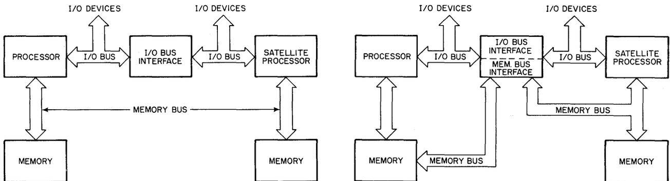
Input/Output Bus Links Between the DECsystem-10 and a Satellite Processor
