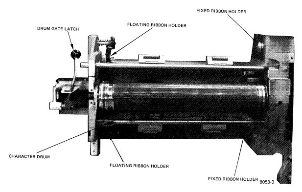
Figure 1-16: LP10 Ribbon Installation
