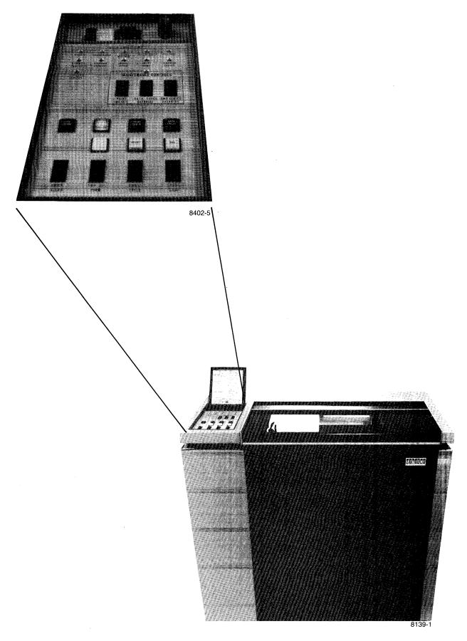
Figure 1-10: LP07 Line Printer
