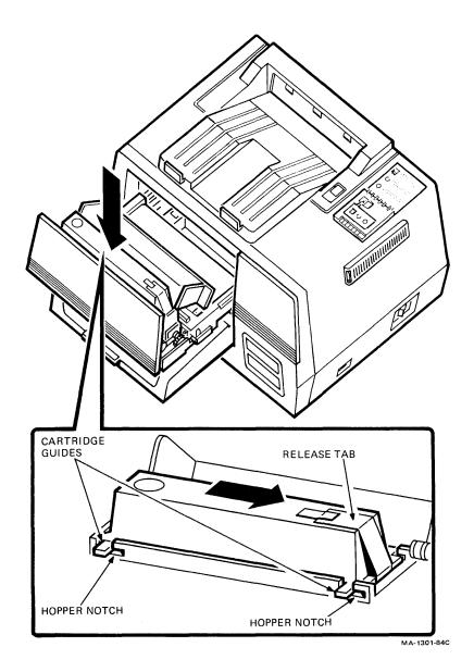
Figure 1-25: LN03 Toner Cartridge Hopper Notches
