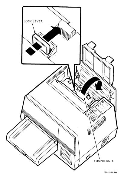
Figure 1-28: LN03 Paper Exit Cover Lock Lever
