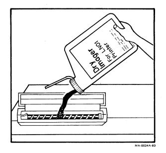
Figure 1-20: Adding Dry Imager to the Hopper
