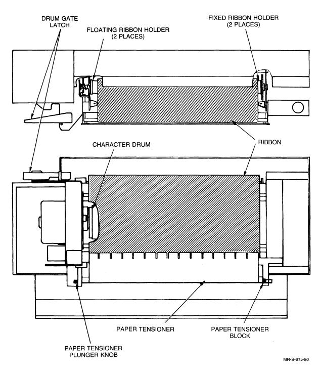
Figure 1-9: LP05, LP14, LP26 or LP27 Ribbon Installation
