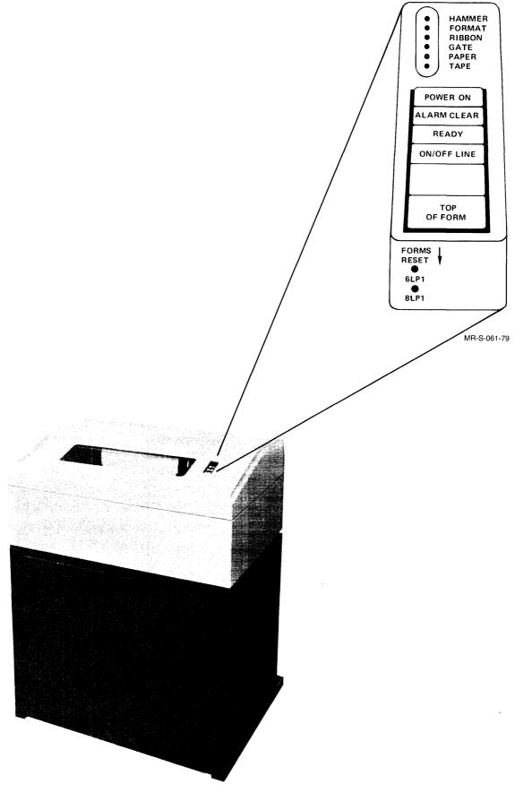
Figure 1-2: LP14 Line Printer
