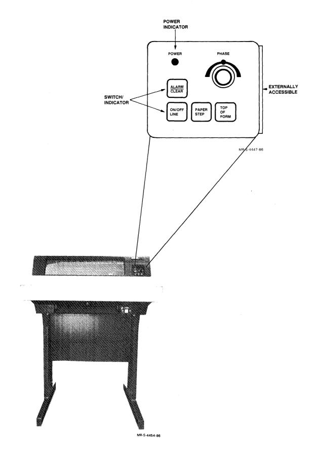
Figure 1-3: LP26 Line Printer
