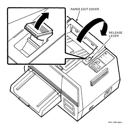
Figure 1-27: LN03 Paper Exit Cover Release Lever
