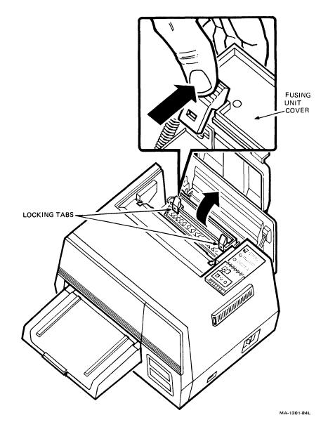
Figure 1-29: LN03 Fusing Unit Cover Locking Tabs
