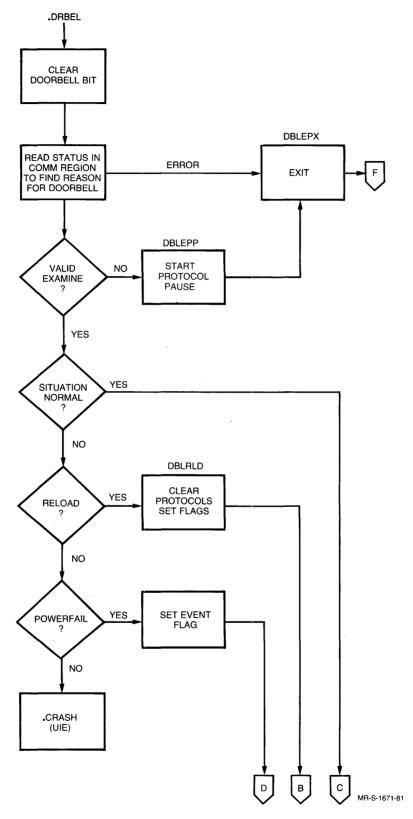
Figure 8-5 DTE Interrupt Handler (part 4 of 5)
