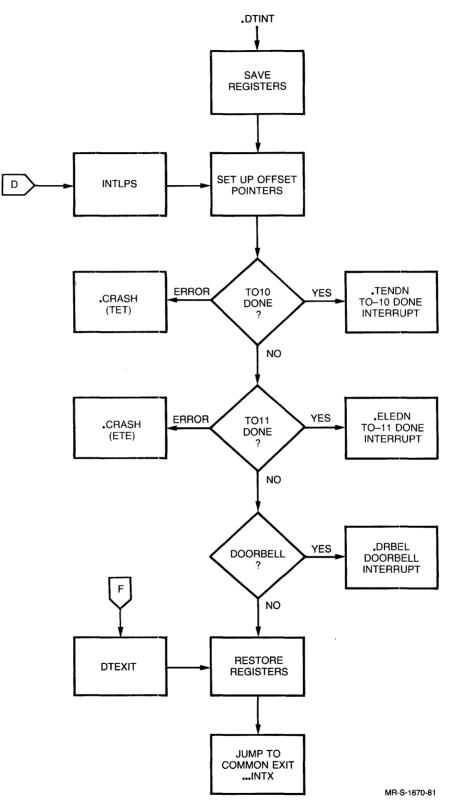
Figure 8-5 DTE Interrupt Handler (part 1 of 5)
