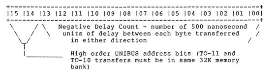
DLYCNT Since the DTE-20 is clocked from the EBUS clock module, which runs at a different rate from the PDP-11 clock, a compromise in timing must be effected in order to transfer data over the DTE-20. Therefore, the PDP-11 sets this register to notify the DTE-20 of the speed at which to carry out byte transfer operations. The register contains the number of 500 nanosecond units of delay that should come between two consecutive byte transfers.
