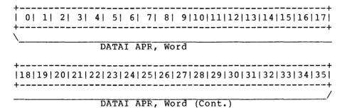
The CMDAPR word is the storage area provided for reading the current break conditions from the Arithmetic Processor. The DATAI APR, instruction puts the information here. (For more information on break conditions and the Arithmetic Processor, refer to the DECsystem-10/DECSYSTEM-20 Processor Reference Manual.)
