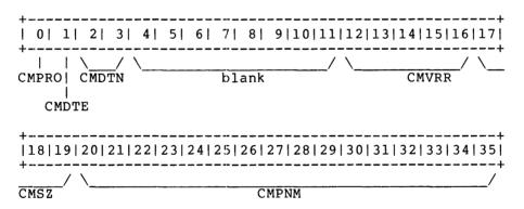
The TOPID word is the first location in each "To" processor area. This word contains information on the connections between the owning processor and the "To" processor.
