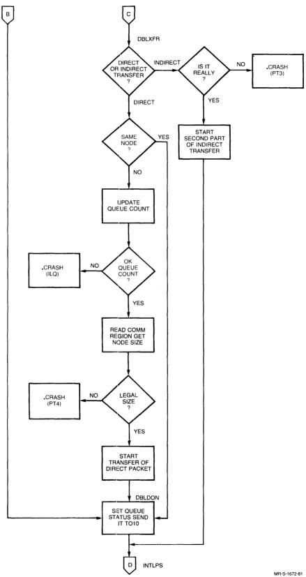
Figure 8-5 DTE Interrupt Handler (part 5 of 5)
