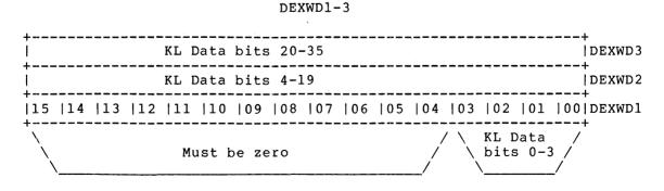
DEXWD1-3 During a deposit or examine operation, the data being deposited or examined appear in these three registers. However, DEXWD1 must always contain zeros in the high-order bits.
