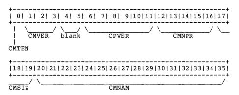
The PIDENT word provides information about the owning processor and its area. The separate fields in PIDENT are described below.
