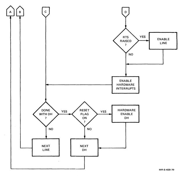
Figure 7-9 Terminal Timeout Algorithm (Cont.)
