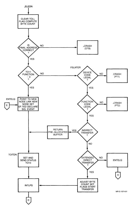
Figure 8-5 DTE Interrupt Handler (part 3 of 5)
