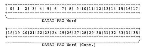
The CMPDWD word is the storage area provided for reading the process status of the Pager. The DATAI PAG, instruction puts the status information here. (For more information on the Pager refer to the DECsystem-10/DECSYSTEM-20 Processor Reference Manual.)
