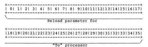
This word contains a copy of the "To" processor's reload word. The copy is saved by the owning processor in case the "To" processor crashes.
