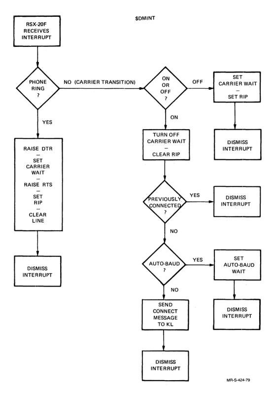
Figure 7-6 Modem Control Algorithm
