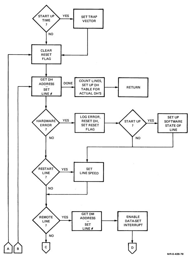
Figure 7-9 Terminal Timeout Algorithm
