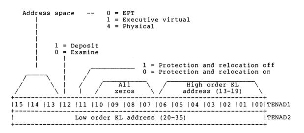
TENAD1-2 The PDP-11 uses these two registers in examine and deposit operations to specify the KL address. When the PDP-11 writes TENAD2 the deposit/examine operation ' is initiated; thus, all necessary data must be written to DEXWD1-3 before TENAD2 is written.
