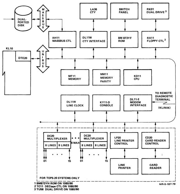
Figure 1-1 The Front End for a KL-based Computer System
