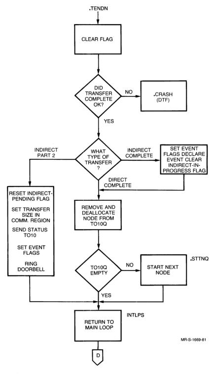
Figure 8-5 DTE Interrupt Handler (part 2 of 5)
