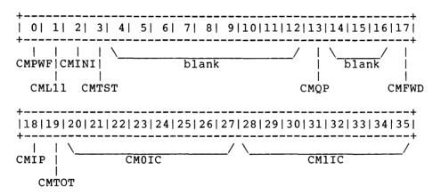
The STATUS word is intended to be the only word a processor has to examine when it receives a doorbell interrupt. The STATUS word contains the following status bits and counters:
