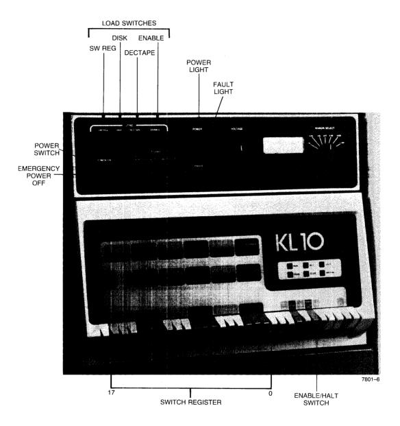
Figure 5-2 Load Switches and Switch Register for KL with DECtapes
