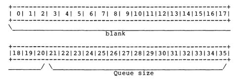
This word contains the number of eight-bit bytes written into the current packet by the transmitting processor. The packet can contain more than one message; this word does not contain a count of the number of messages, only of the number of bytes.
