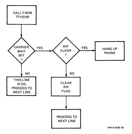
Figure 7-7 Modem Timeout Algorithm
