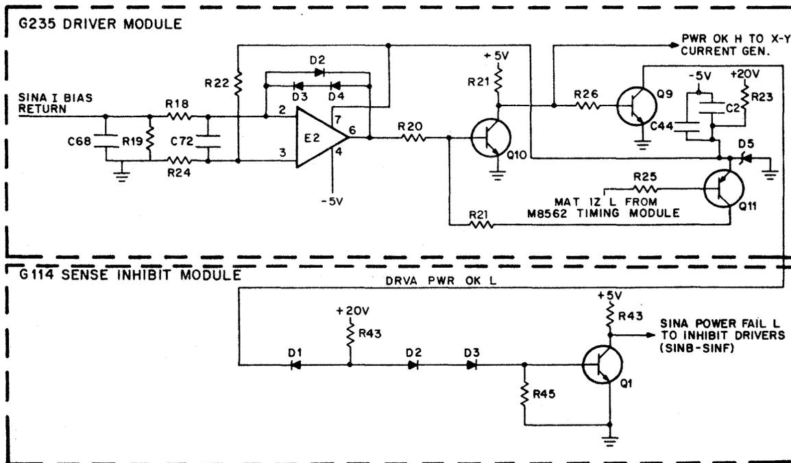
Figure 4-23 DC LO and Bias Current Detection Circuit
