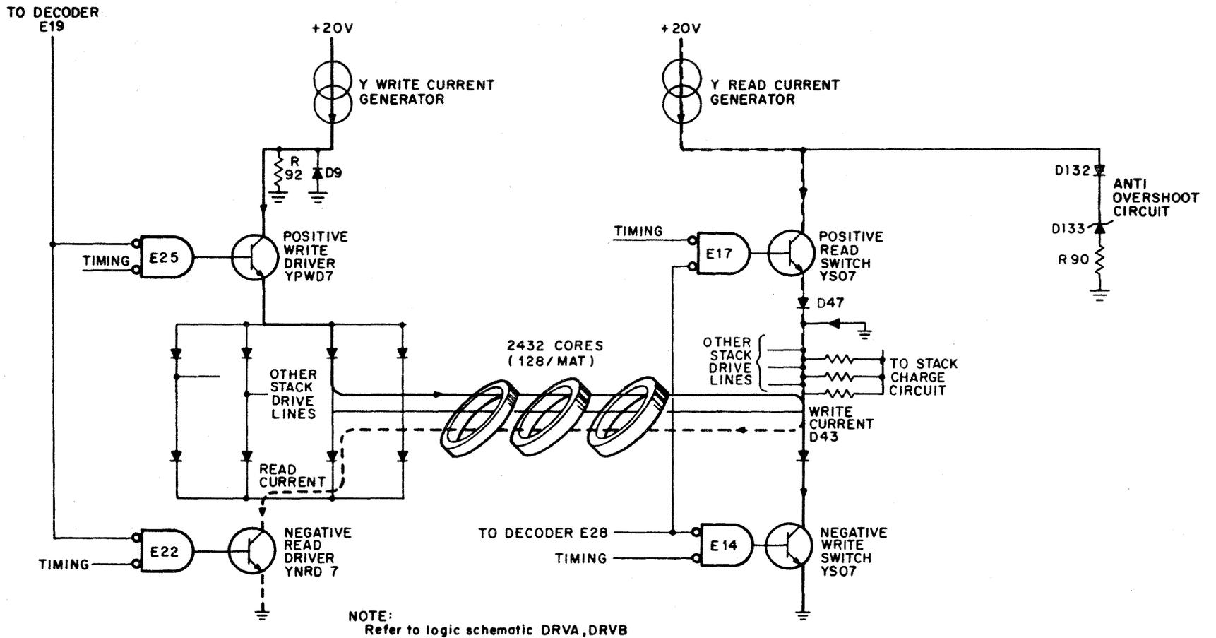
Figure 4-16 Typical Y Line Read Write Switches and Drivers
