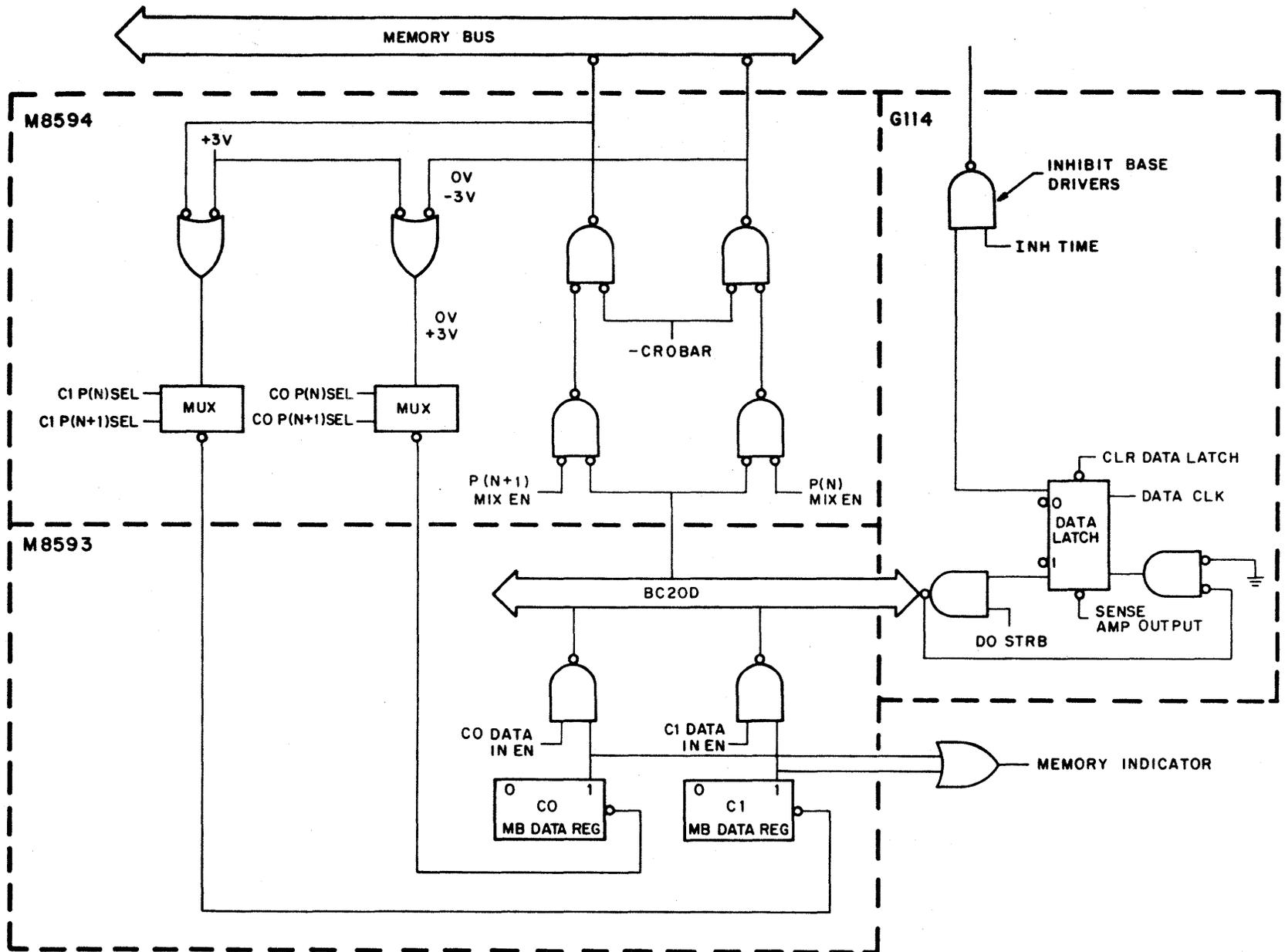
Figure 4-5 Data Path Diagram
