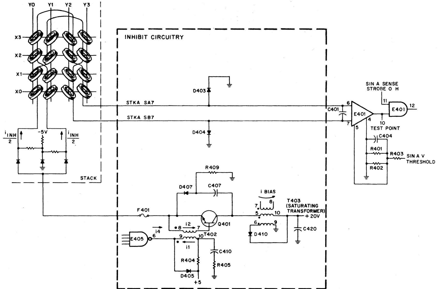
Figure 4-20 Sense Amplifier and Inhibit Driver
