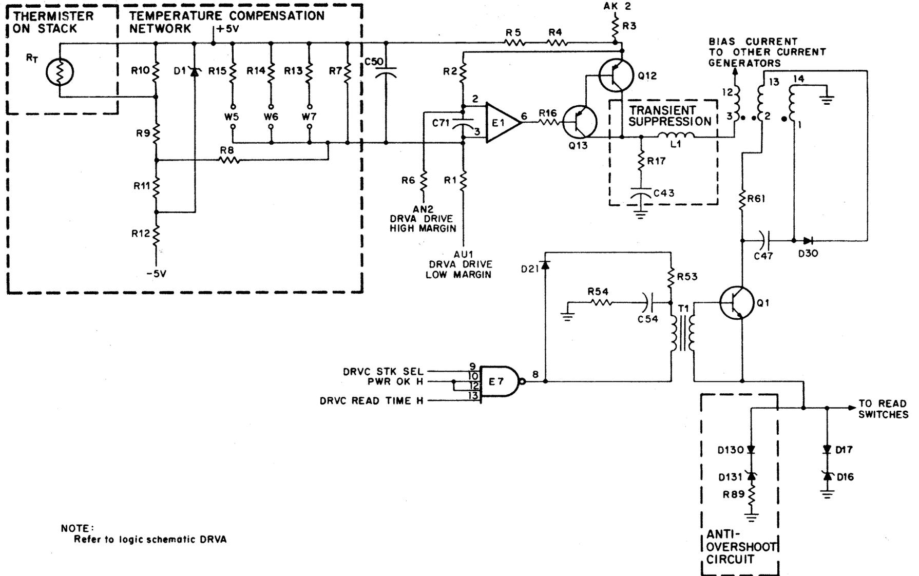
Figure 4-19 Bias Current Supply and Read X Current Generator
