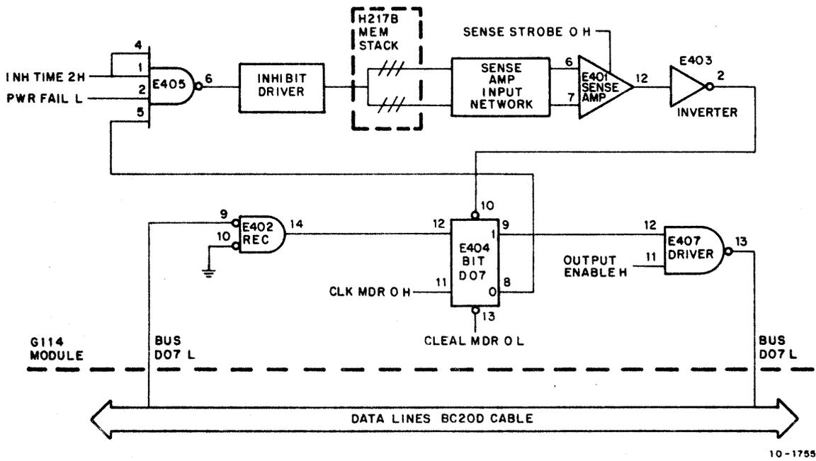
Figure 4-17 Read and Write Data Path
