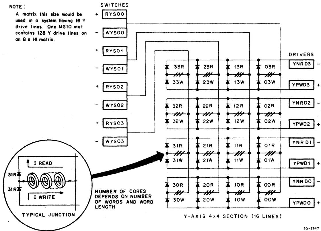
Figure 4-15 Simplified Y Line Selection Stack Diode Matrix
