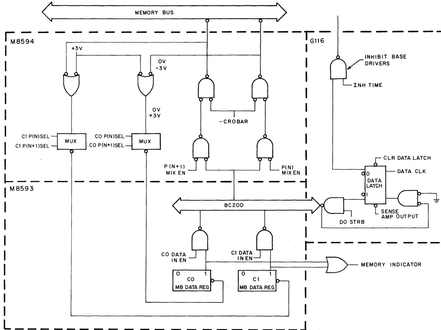
Figure 4-5 Data Path Diagram
