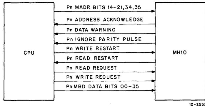
Figure 4-1 Memory Processor Interface
