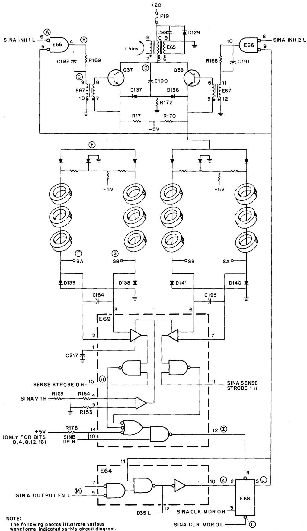
Figure 5-3 Typical Sense/Inhibit Circuit
