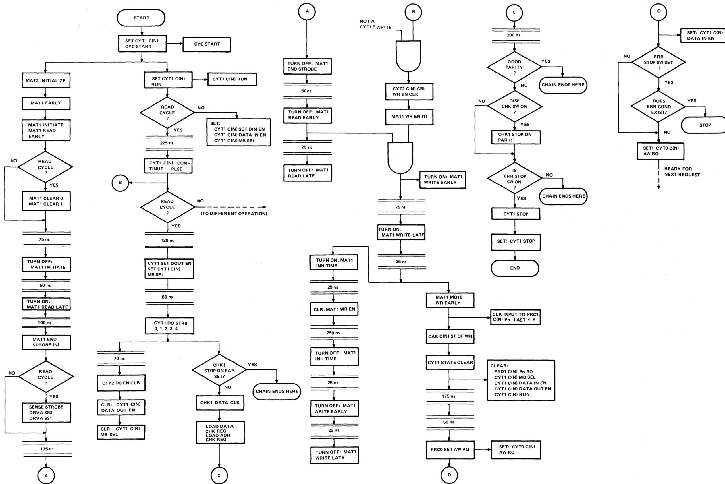
Figure 4-7 Read Restore Timing Flow Diagram
