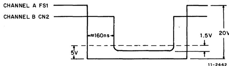
Figure 5-1 Sense Strobe Delay Waveform
