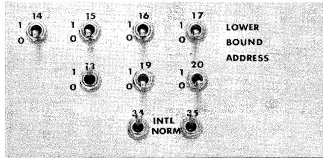
**Figure 3-3 Memory Address Switches**
