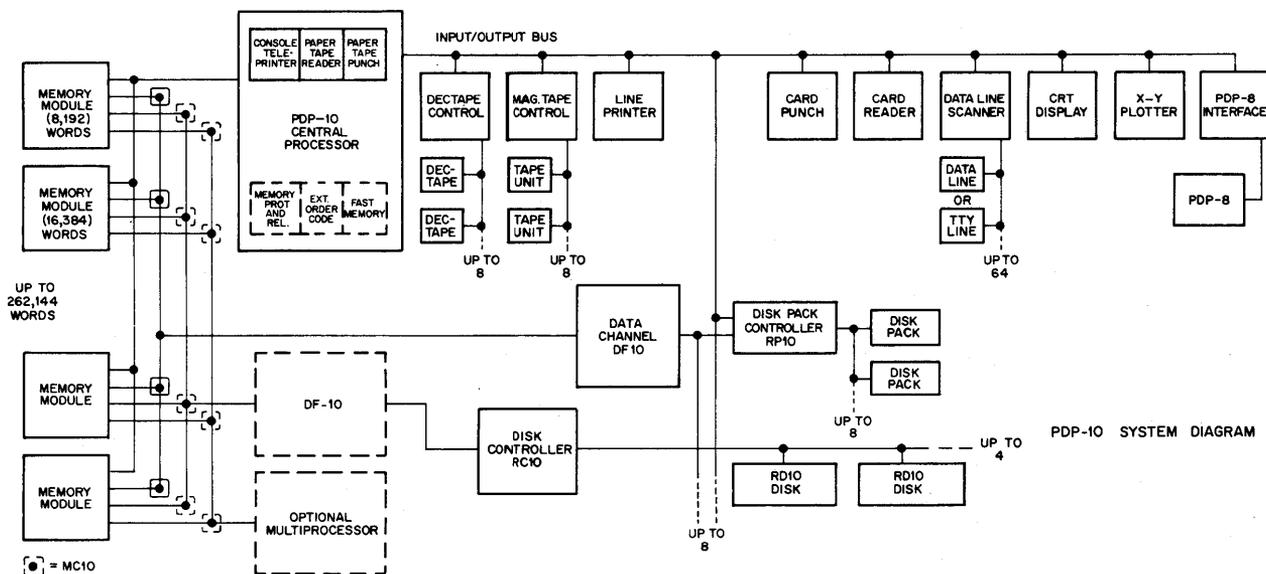
Figure 1 PDP-10 System With Up to 8 Disk Packs
