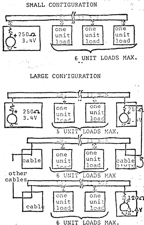
Figure 5. Small and Large BUS Configurations
