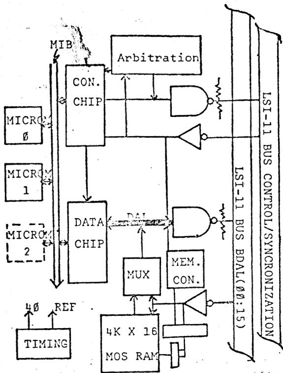
Figure 3. Processor Module Configuration
