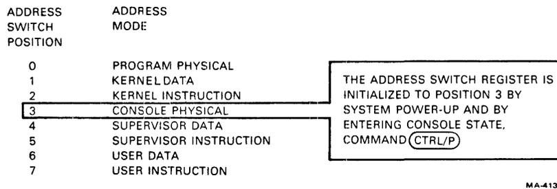
Figure 4-3 Address Display Multiplexer
