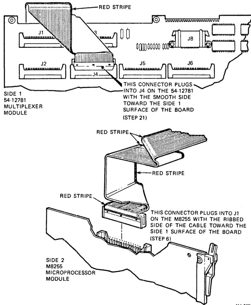
Figure 6-6 BC06R-3 Cable Configuration
