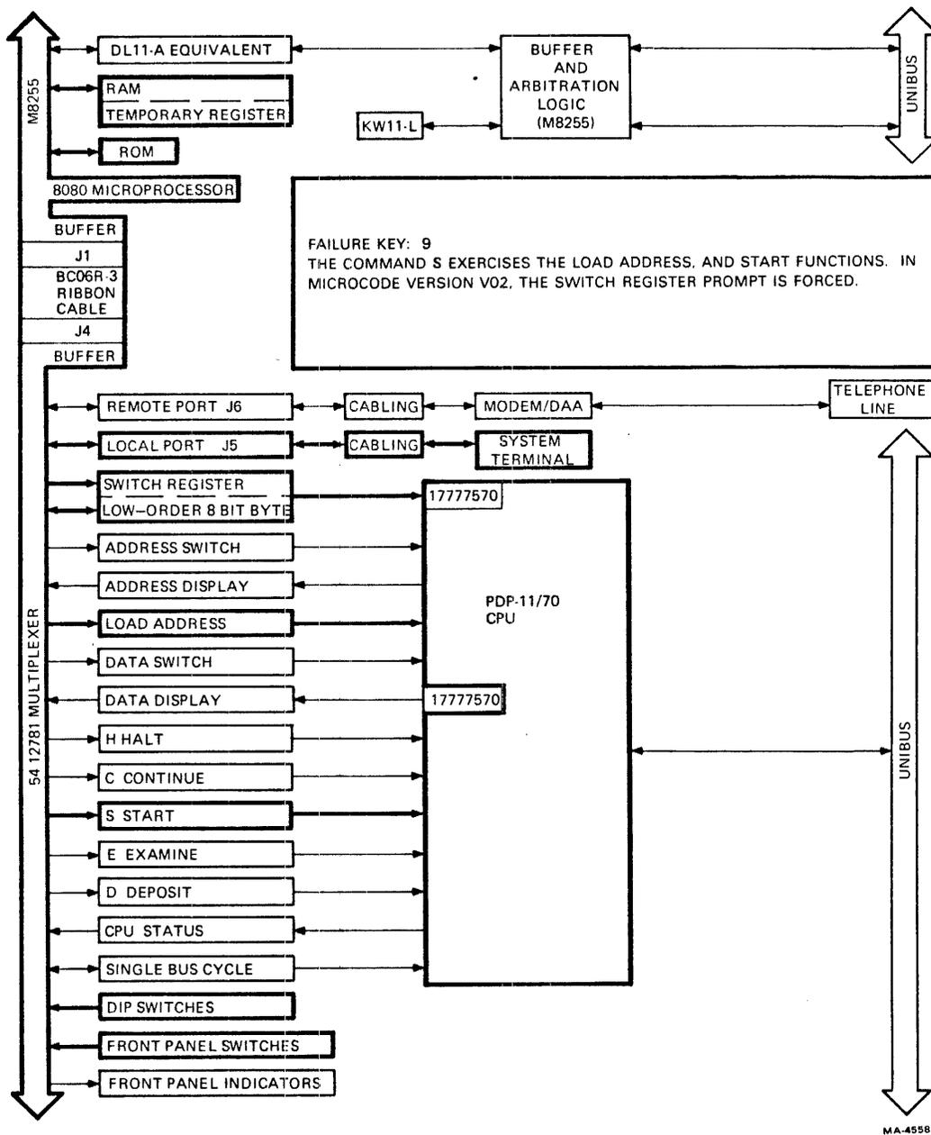
Figure 7-9 Failure Key 9
