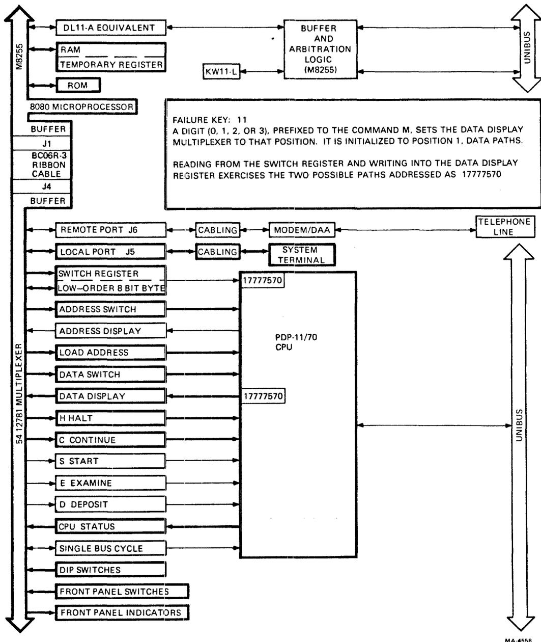
Figure 7-11 Failure Key 11
