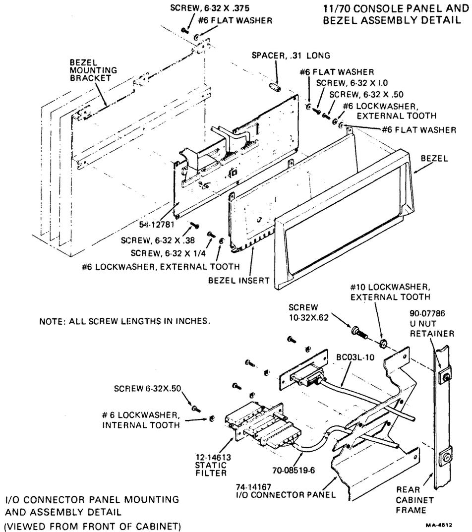
Figure 6-9 KY11-RB/KY11-RE Mechanical Assembly
