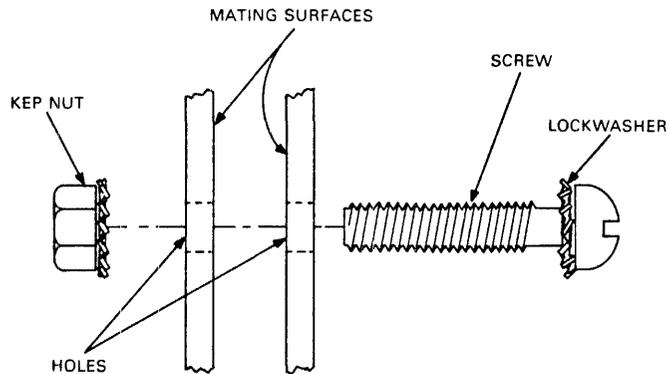
SCREW, LOCKWASHER, AND KEP NUT MOUNTING
