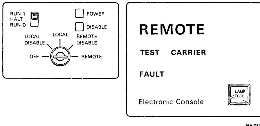
Figure 2-1 Electronic Console Panel Controls and Indicators
