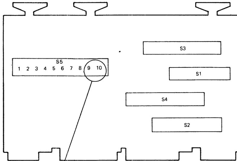
REAL TIME CLOCK OPTION IS ENABLED IF S5 SWITCH 9 IS OFF AND SWITCH 10 IS ON.
