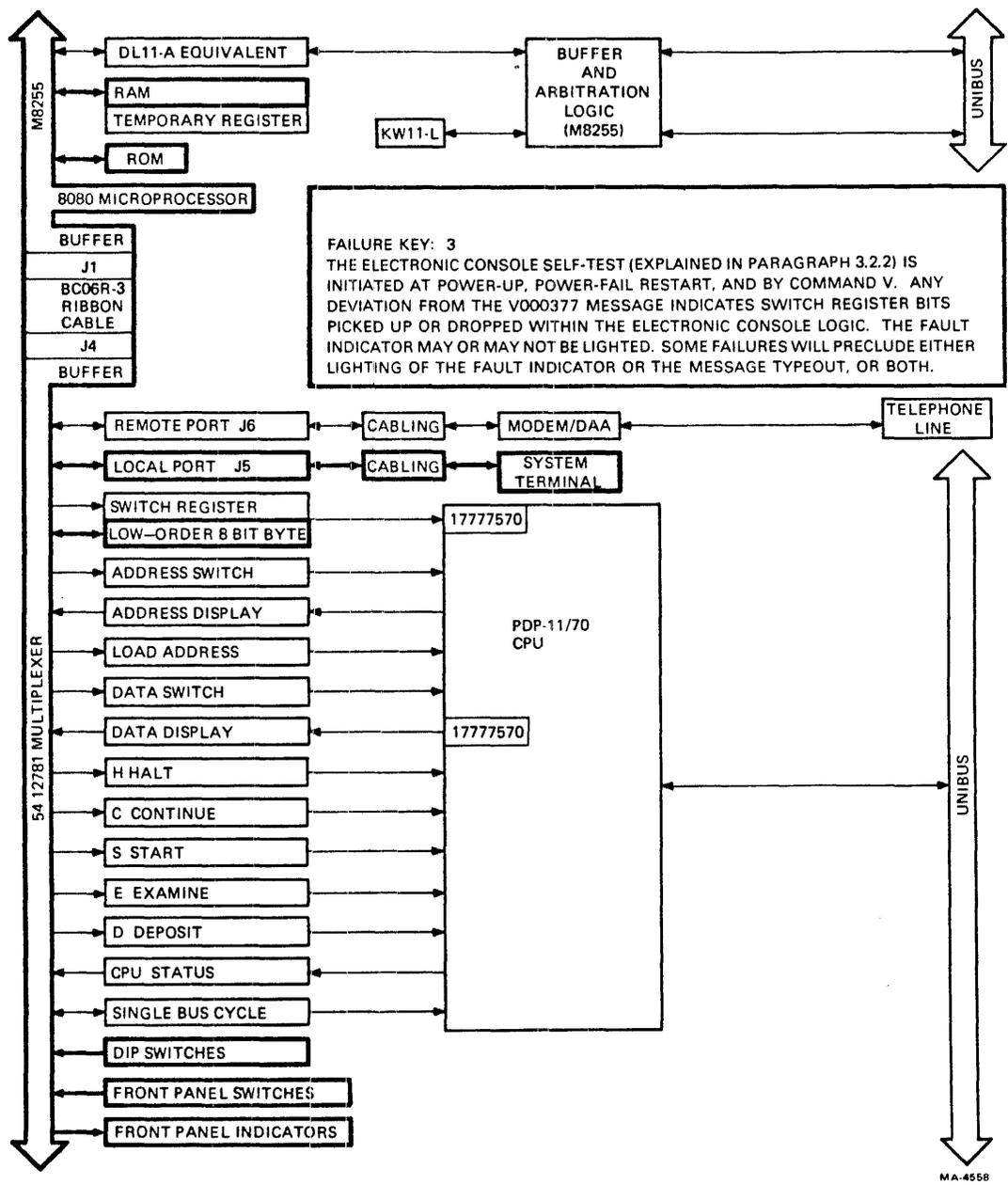
Figure 7-3 Failure Key 3
