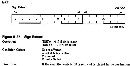
operand; if the N-bit is clear, a 0 is placed in the destination This instruction is particularly useful in multiple-precision arithmetic because it permits the sign to be extended through multiple words.
