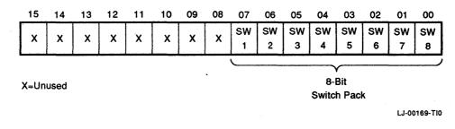
Figure 1–31 Boot and Diagnostic Configuration Register Format (17777524 - Read-Only) • Write-only boot and diagnostic display register.
