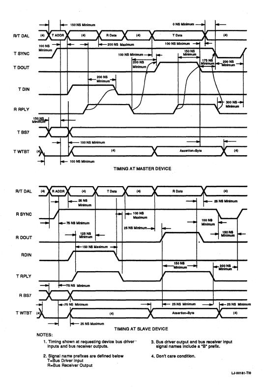
Figure 5–6 DATIO or DATIO(B) Bus Cycle Timing
