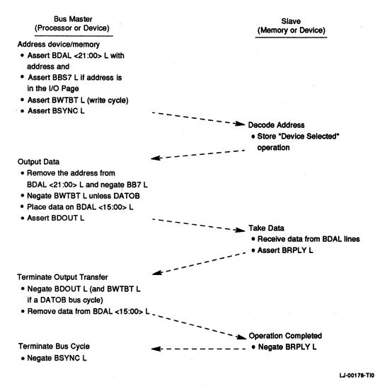
Figure 5–3 DATO or DATO(B) Bus Cycle
