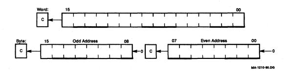
Figure 8–28 Example: Arithmetic Shift Left
