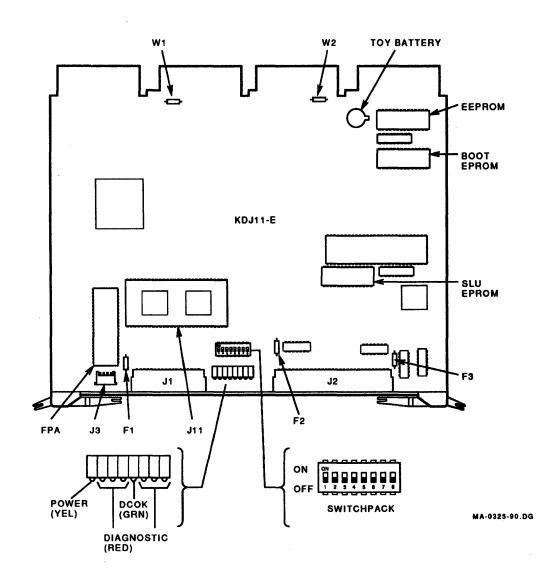
Figure 1–24 KDJ11-E Jumper and DIP Switch Locations
