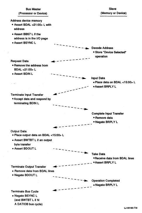
Figure 5–5 DATIO or DATIO(B) Bus Cycle
