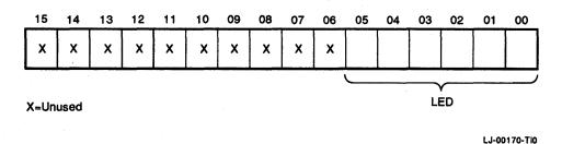
Figure 1–32 Boot and Diagnostic Display Register Format (17777524 - Write-Only)
