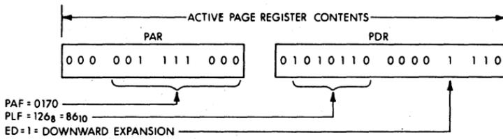
To specify page length for a downward expandable page, write complement of blocks required into high byte of PDR.
