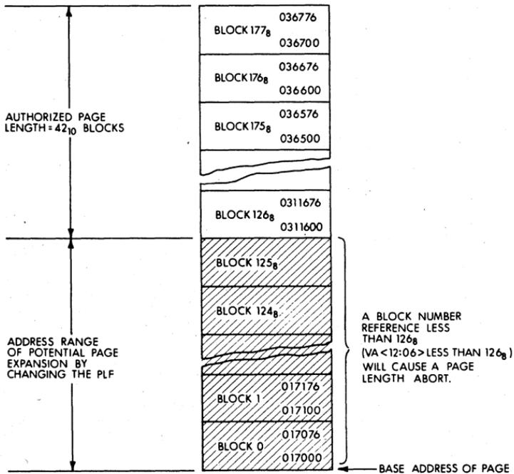
Figure 7-7 Example of a Downward Expandable Page
