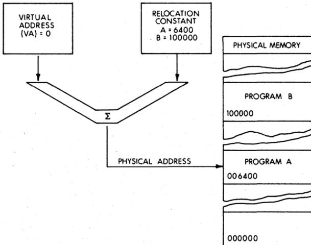
Figure 7-2 Simplified Memory Relocation Example
