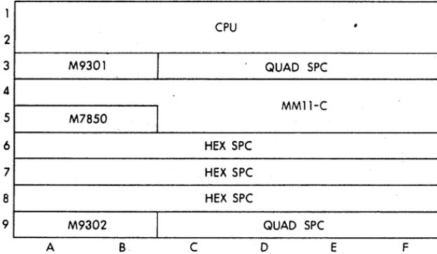
Figure 6-2 8K Core using MM11-C
