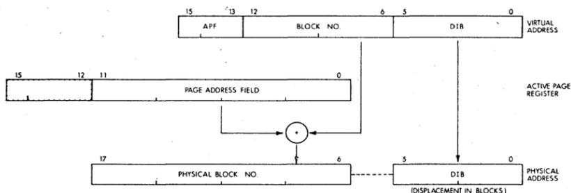
Figure 7-10 Construction of a Physical Address
