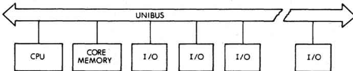
Figure 2-1 PDP-11 System Simplified Block Diagram
