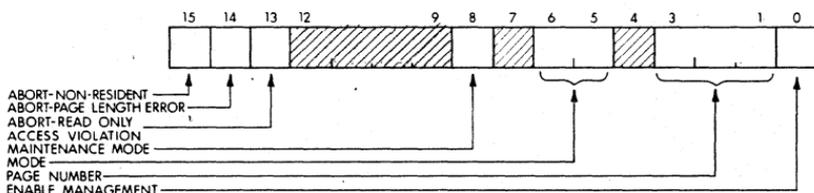
**Figure 7-11 Format of Status Register #0 (SR0)**
