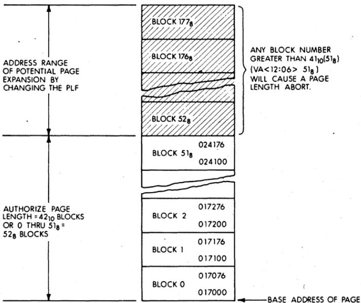
Figure 7-6 Example of an Upward Expandable Page
