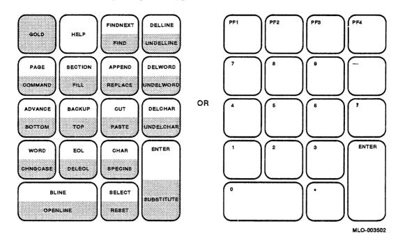
Most of the function keys specify two functions: a standard function and an alternate function.
