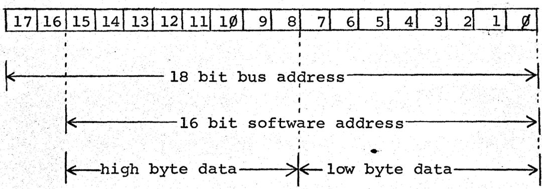
The processor converts the software address to a full 18-bit bus address. On word bus commands (DATI, DATO, DATM), the slave ignores D0; on byte bus commands (DATOB, DATMB), slave receives byte data on D  $\langle 15:8 \rangle$  if D0=1 or D  $\langle 7:\emptyset \rangle$  if D0= $\emptyset$ .
