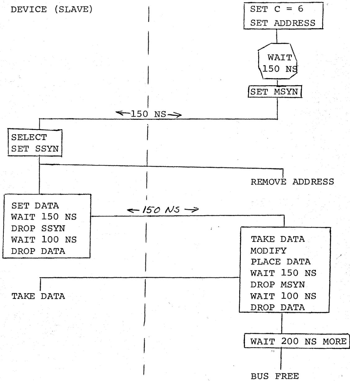
$$\text{DATM} = 5 \times 150 \text{ NS} + 300 \text{ NS} = 1050 \text{ NS}$$
