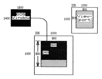
Figure 1-3: Isotropic Mapping: Window to Viewport
