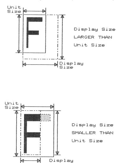
Figure 1-13: Character Unit Cell and Display Cell
