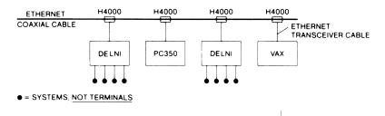
Although the DELNI is limited to a range of 100 meters, a DELNI local area network can be expanded by connecting to a second DELNI or to a larger Ethernet network.
