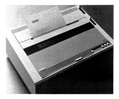
Operating the LQP03 is simple, with ease-of-use features unavailable on other daisywheel printers. You load or adjust paper by pressing the soft-touch pushbutton controls on the top front of the printer; rolling platen knobs and lining up paper are things of the past. In addition, you'll appreciate no-mess cartridge ribbons that snap in and out for quick, clean ribbon changes.
