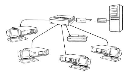
Digital's Mini-Exchange provides local communications, common access to shared devices, and common access to remote computers via a modem.
