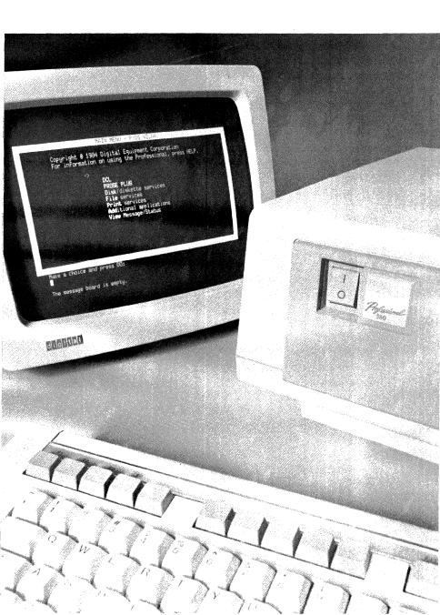
The Professional Series consists of three models: the Professional 325, the Professional 350, and the Professional 380. All feature Digital's highly acclaimed keyboard, a high-resolution monochrome or color monitor, a PDP-11-based CPU with floating-point processor, bit-mapped graphics, 512 Kbytes of main memory, an 800-Kbyte dual-diskette drive, and communications, printer, and network interconnect ports.
