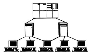
The Professional is designed to be part of a fully distributed data processing system.
