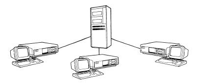
PRO/Communications provides many communications capabilities, including file transfer between Professionals and VAXes. the Professional to either a PDP-11 or VAX-11 host system running Professional Host Communications software. Both of the above file transfer operations take advantage of Digital's error-correcting protocol.
