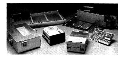
The Professional's modular design makes it easy to upgrade and service. In fact, the entire system unit can be disassembled in minutes, using nothing more than a ball-point pen. Any subassembly can be removed for inspection, repair, or replacement, and all system options are user-installable.
