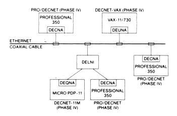
The DECNA Ethernet Controller allows the Professional to connect directly to Ethernet coaxial cable (via an H4000 Transceiver) or to a Local Network Interconnect (DELNI) device.
