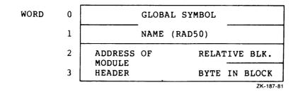
Figure 10-4 Format of Entry Point Table Element
