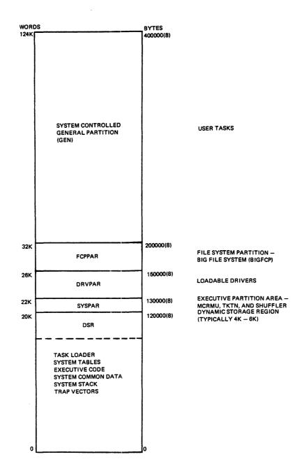
Figure 1-2 Example of a Mapped 124K RSX-11M System
