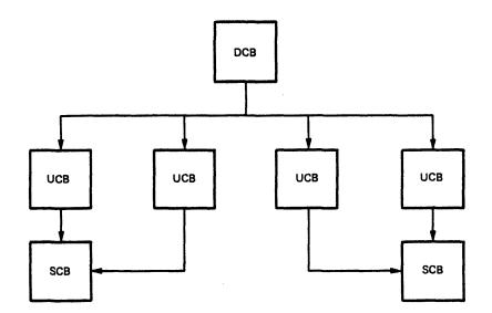
Figure 8-23 I/O Data Structure for Two RK11 Disk Controllers
