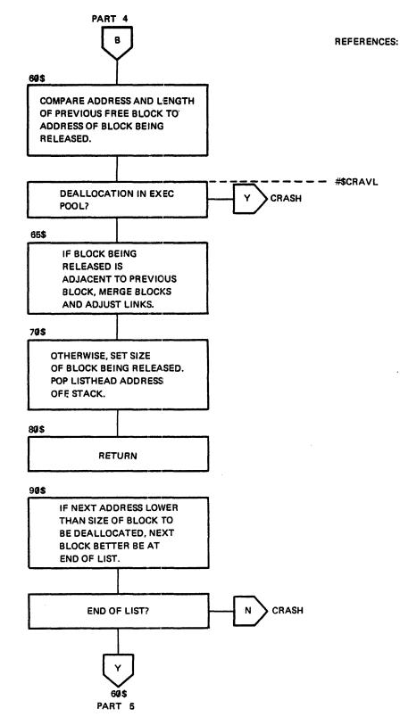
Figure 2-6 \$DECLK-\$DEPKT-\$DEACB Logical Flow Diagram (Part 5 of 5)
