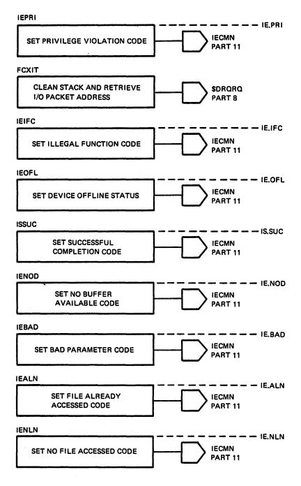
Figure 6-2 QIO Directive Processing (Part 12 of 24)
