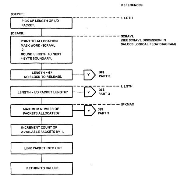
Figure 2-6 \$DECLK-\$DEPKT-\$DEACB Logical Flow Diagram (Part 2 of 5)
