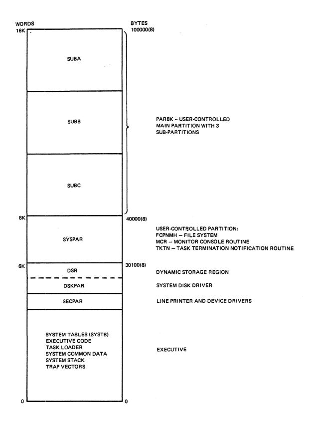
Figure 1-1 Sample Unmapped 16K System Memory Layout
