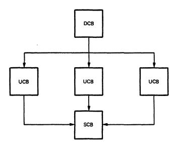
Figure 8-22 RKll Disk I/O Data Structure
