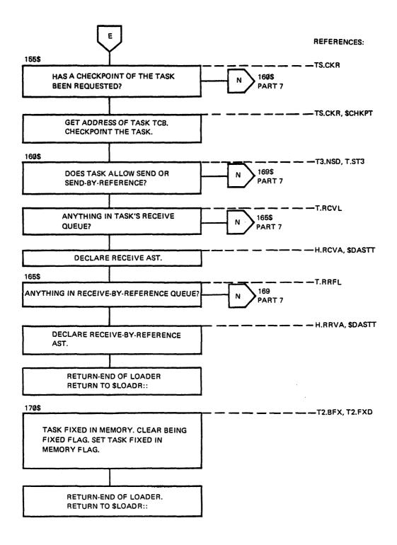
Figure 2-11 Loader Logical Flow Diagram (Part 7 of 8)
