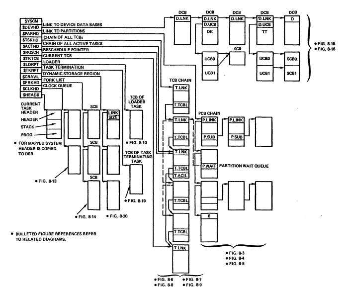
Figure 8-2 Overview of RSX-11M System Control Blocks
