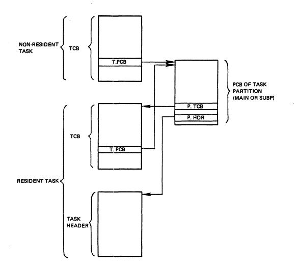
Figure 8-7 Simplified User-Controlled Partition TCB, Task Header, and PCB Relationship
