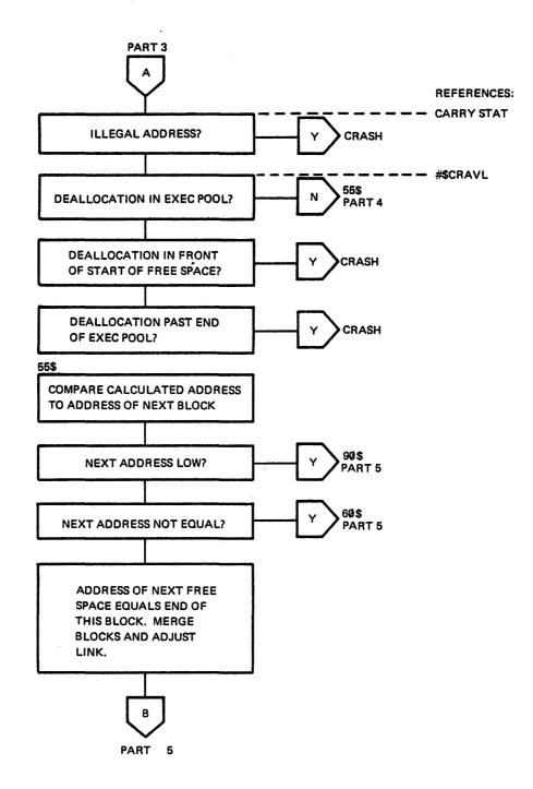
Figure 2-6 \$DECLK-\$DEPKT-\$DEACB Logical Flow Diagram (Part 4 of 5)
