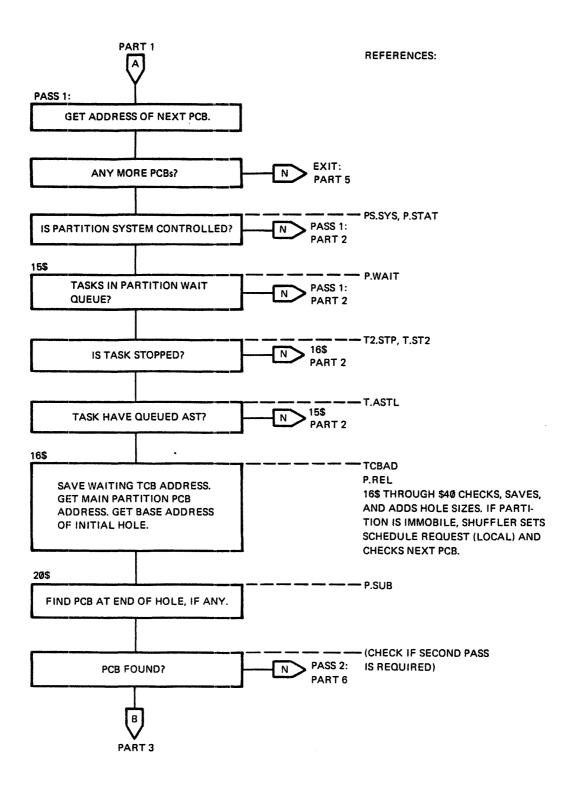
Figure 2-12 Shufller Logical Flow Diagram (Part 2 of 11)
