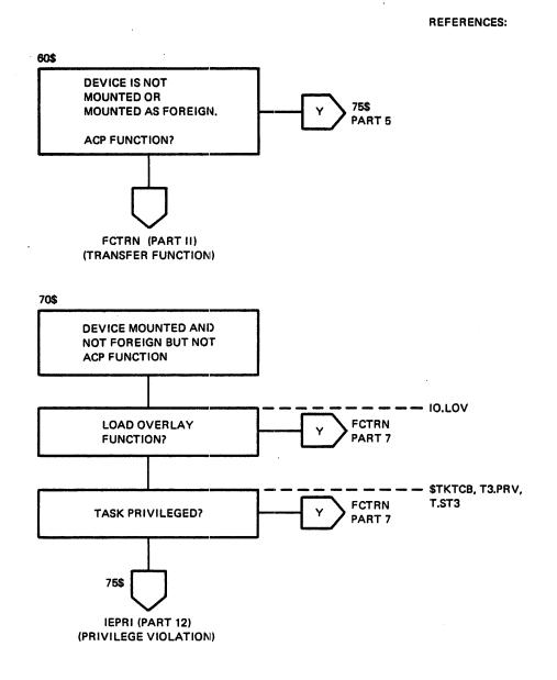
Figure 6-2 QIO Directive Processing (Part 5 of 24)
