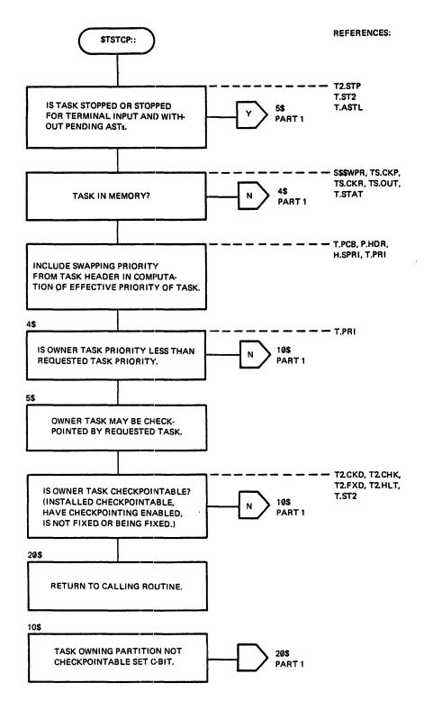
Figure 2-10 \$TSTCP Logical Flow Diagram (Part 1 of 1)
