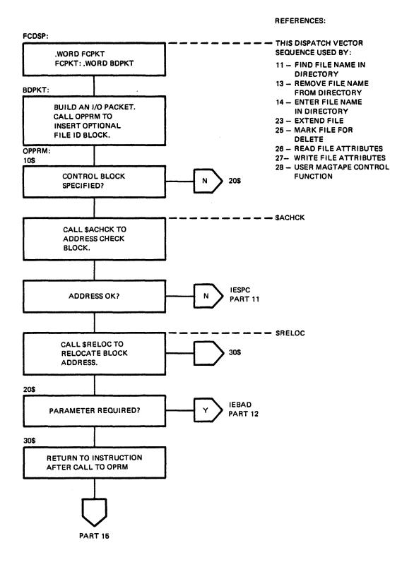
Figure 6-2 QIO Directive Processing (Part 14 of 24)
