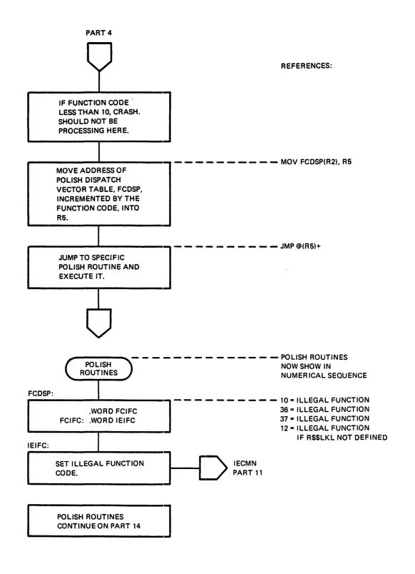
Figure 6-2 QIO Directive Processing (Part 13 of 24)
