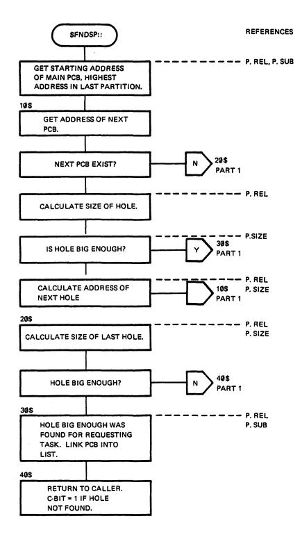
Figure 2-7 \$FNDSP Logical Flow Diagram (Part 1 of 1)
