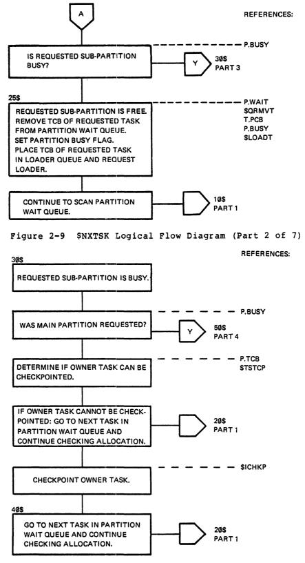
Figure 2-9 \$NXTSK Logical Flow Diagram (Part 3 of 7)
