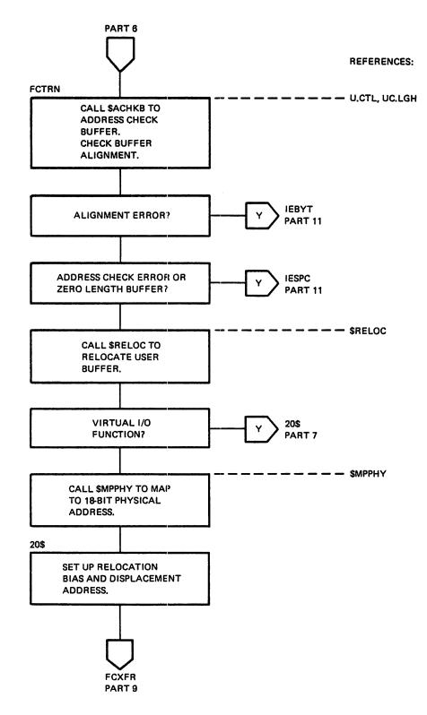
Figure 6-2 QIO Directive Processing (Part 7 of 24)
