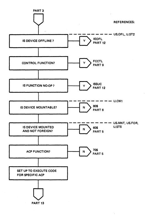
Figure 6-2 QIO Directive Processing (Part 4 of 24)
