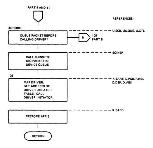
Figure 6-2 QIO Directive Processing (Part 8 of 24)
