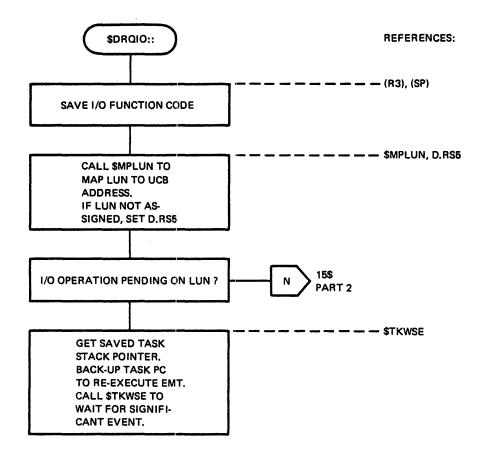
Figure 6-2 QIO Directive Processing (Part 1 of 24)
