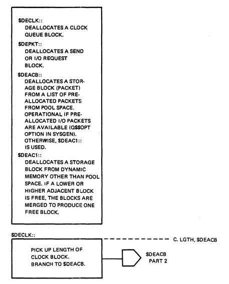
Figure 2-6 \$DECLK-\$DEPKT-\$DEACB Logical Flow Diagram (Part 1 of 5)
