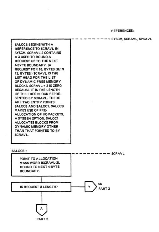
Figure 2-4 \$ALOCB Logical Flow Diagram (Part 1 of 2)
