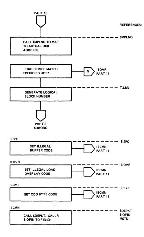
Figure 6-2 QIO Directive Processing (Part 11 of 24)
