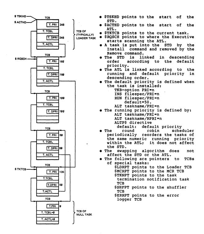
Figure 8-6 Example of a System Task Directory (STD) and Active Task List
