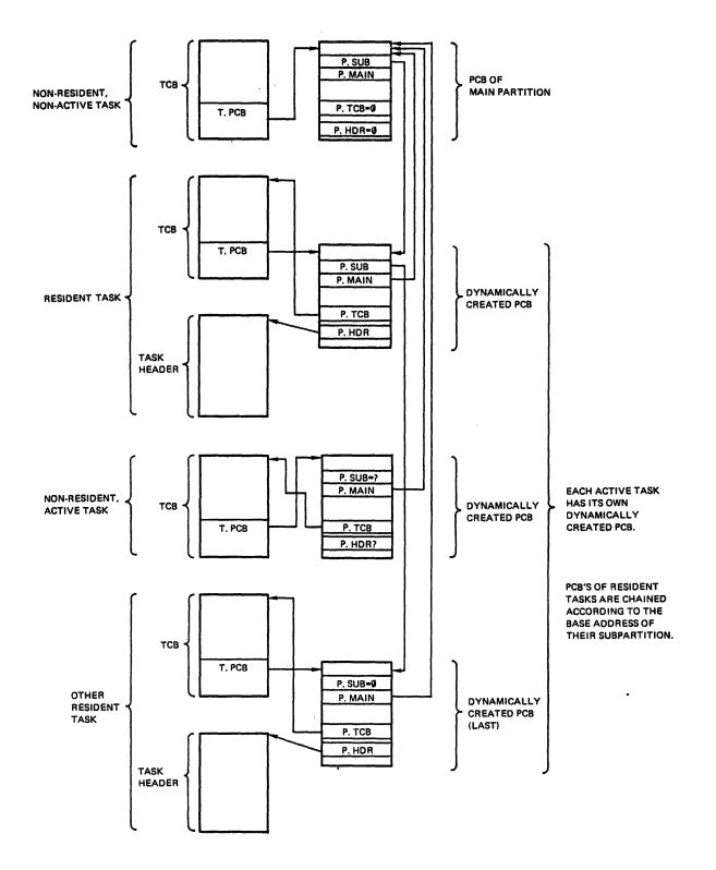
Figure 8-8 TCB, Task Header, and PCB Relationships in a System-Controlled Partition
