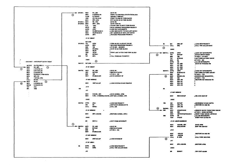
Figure 3-6 Interrupt Flow of Control
