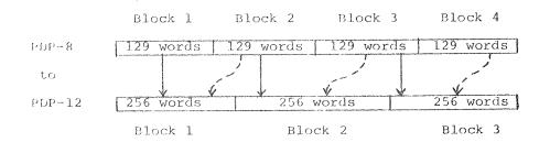
For a PDP-12 to PDP-8 transfer, one 256 word LINCtape block is written on two PDP-8 128 word blocks. 7777 is written for the 129th (link) word in this case.
