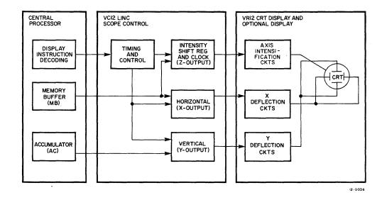
Figure 5-6 Display Control General Block Diagram
