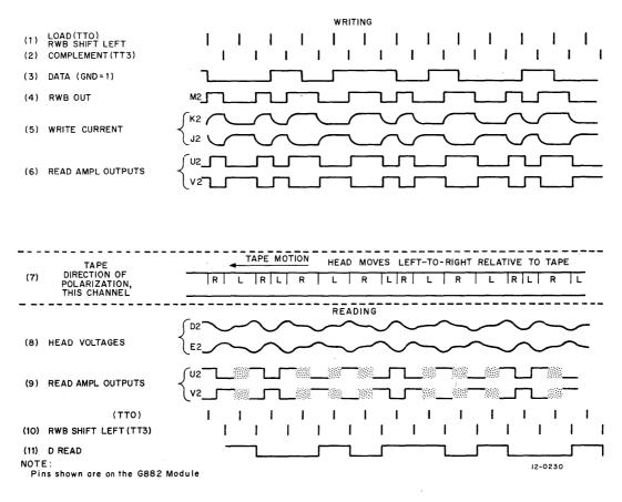
Figure 6-13 Read/Write Logic and Waveforms
