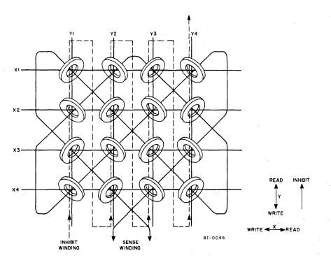
Figure 2-3 Simple Core Memory Plane
