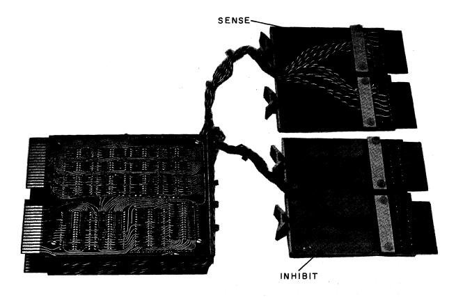
Figure 2-2 PDP-12 Core Memory Stack
