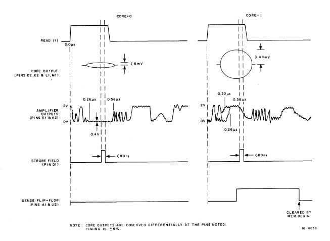
Figure 2-9 Representative Sense Amplifier Waveforms
