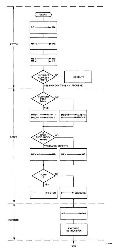
Figure 1-8 8-Mode Address Modification
