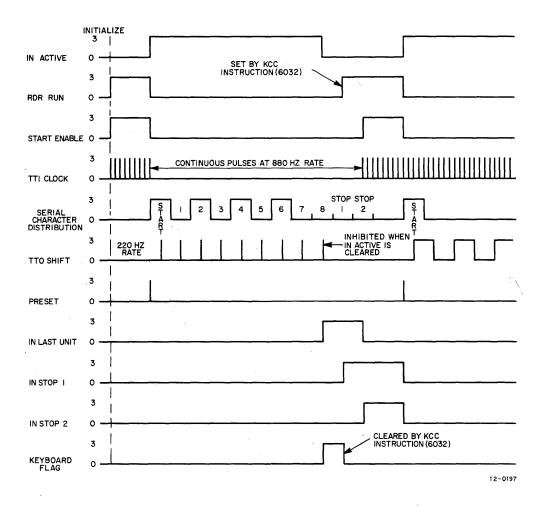
Figure 4-2 Teletype Read Cycle Timing Diagram
