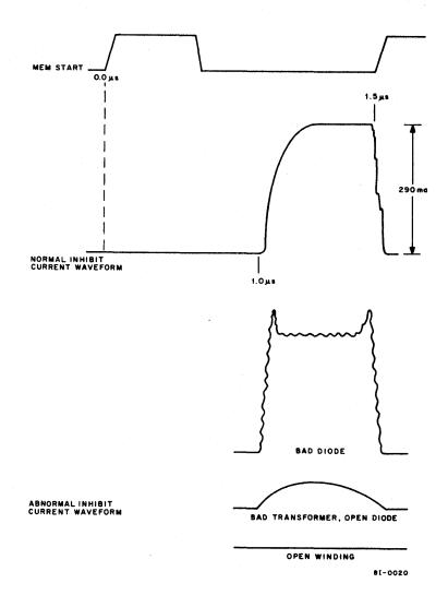
Figure 2-8 Representative Inhibit Current Waveforms
