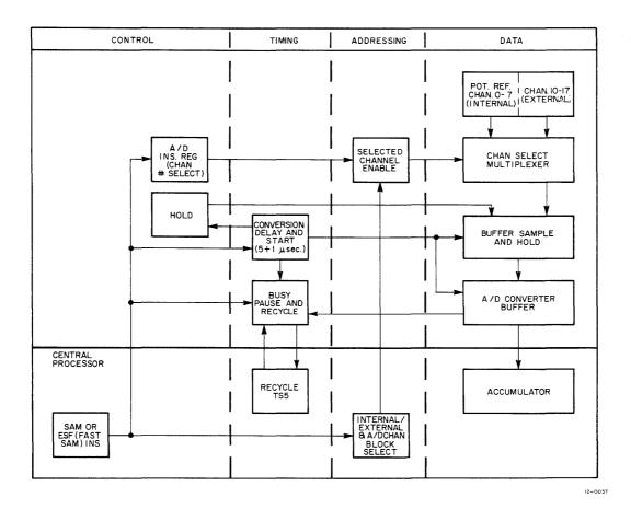
Figure 5-2 A/D Control Block Diagram
