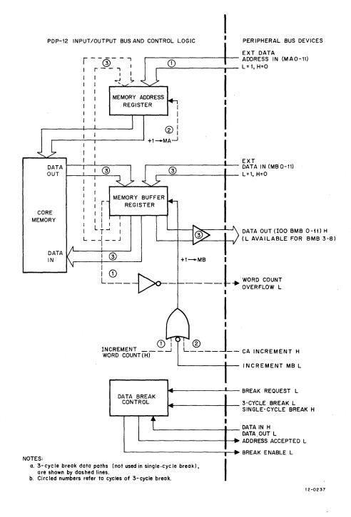
Figure 3-2 Data Break I/O Bus Block Diagram
