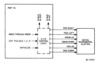
Figure 7-15 XY12 Block Diagram
