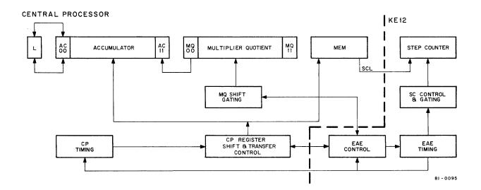
Figure 7-2 Simplified Block Diagram, KE12 EAE
