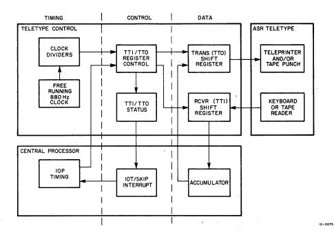
Figure 4-1 Teletype Control Block Diagram
