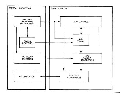
Figure 5-1 A/D Control General Block Diagram
