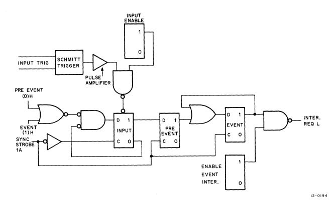
Figure 7-12 Simplified Input Synchronizer Logic Diagram
