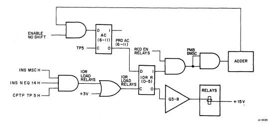
Figure 5-5 Relay Control Functional Block Diagram
