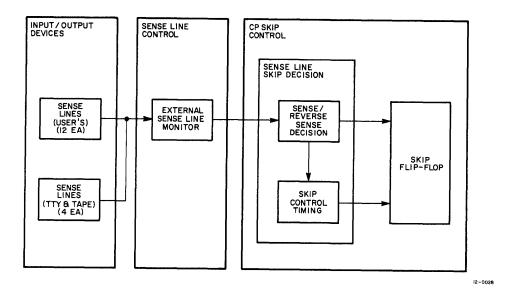
Figure 5-3 Sense Line Control Clock Program
