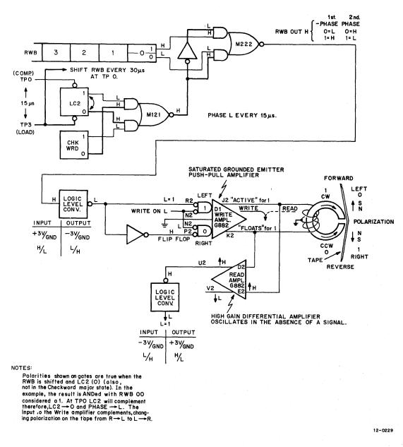
Figure 6-12 Read/Write Simplified Logic
