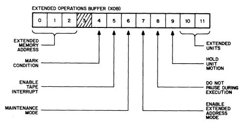
Figure 6-11 Extended Operations Buffer Bit Assignments
