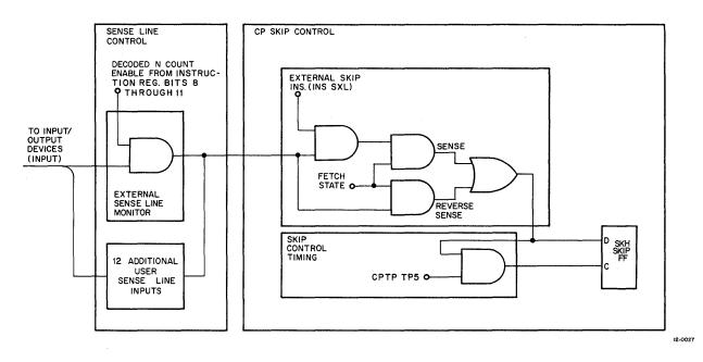
Figure 5-4 Sense Line Control Functional Block Diagram
