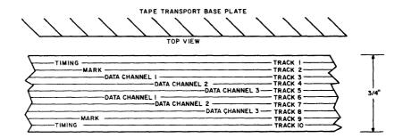
Figure 6-4 Track Allocation Showing Redundantly Paired Tracks
