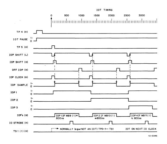
Figure 1-10 IOT Timing
