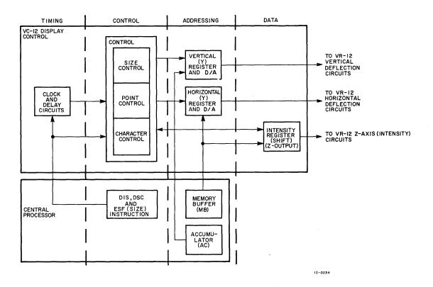
Figure 5-10 Display Addressing Block Diagram
