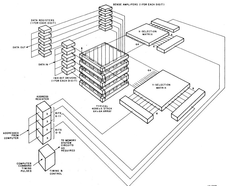
Figure 2-1 Elements of PDP-12 Core Memory
