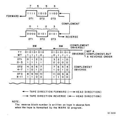
Figure 6-14 Reading A Block Mark
