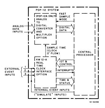
Figure 7-10 KW12-A Real Time Interface Functional Relationship
