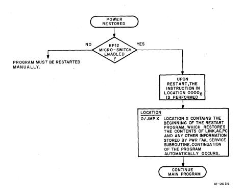
Figure 7-7 Typical Power Failure Program Service Routine
