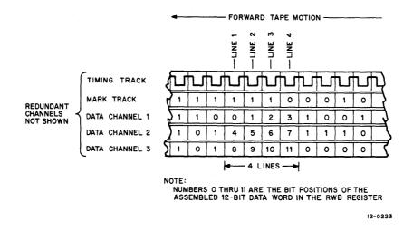
Figure 6-5 Structure of 12-Bit Data Word (4 Tape Lines)
