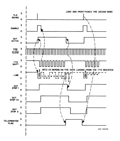
Figure 4-3 Print/Punch Cycle Timing Diagram
