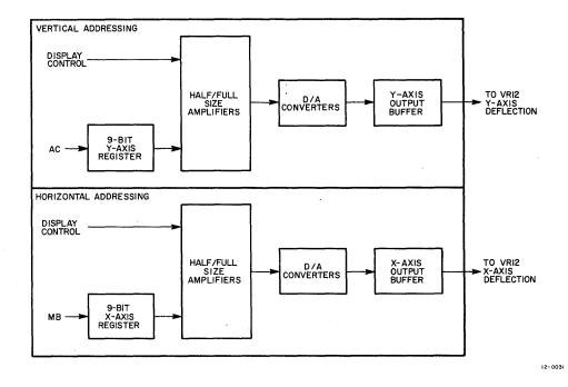
Figure 5-7 Display Control Block Diagram
