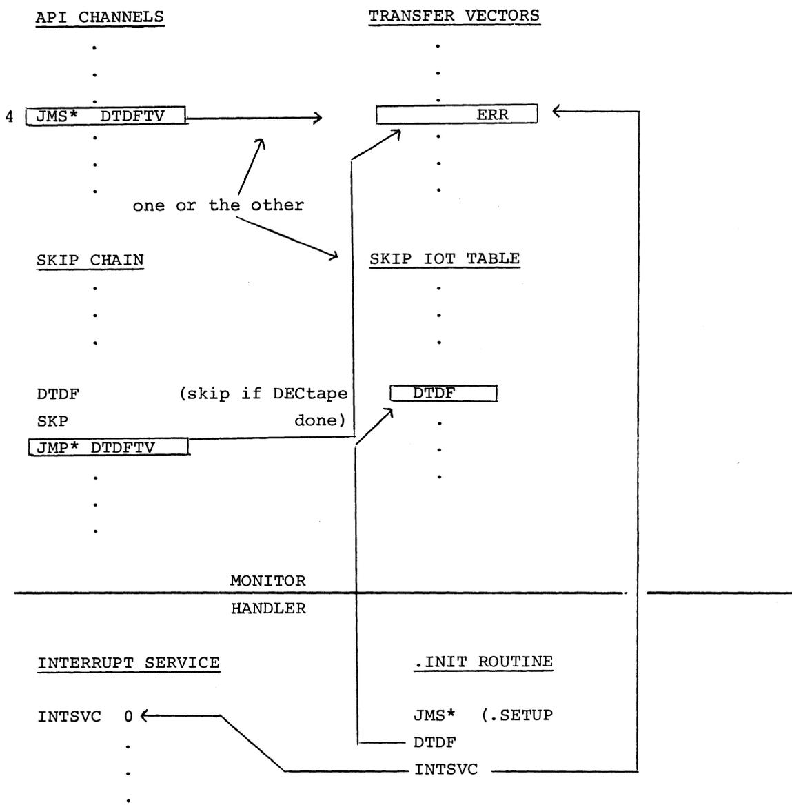
FIGURE 8-1 INTERRUPT LINKAGES FOR I/O DEVICES
