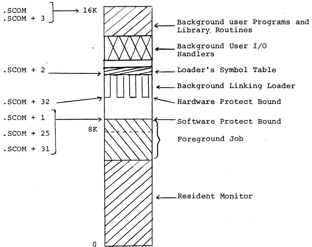
The BACKGROUND Linking Loader overlays the System Loader by loading user programs down from the top of core. User I/O handlers, presuming that they cannot fit in core between the FOREGROUND job and the bottom of the Loader, are loaded into upper core but relocated to run just above the FOREGROUND job so that the memory protect bound can be set above them. Common blocks and I/O buffers are not shown in this memory map.
