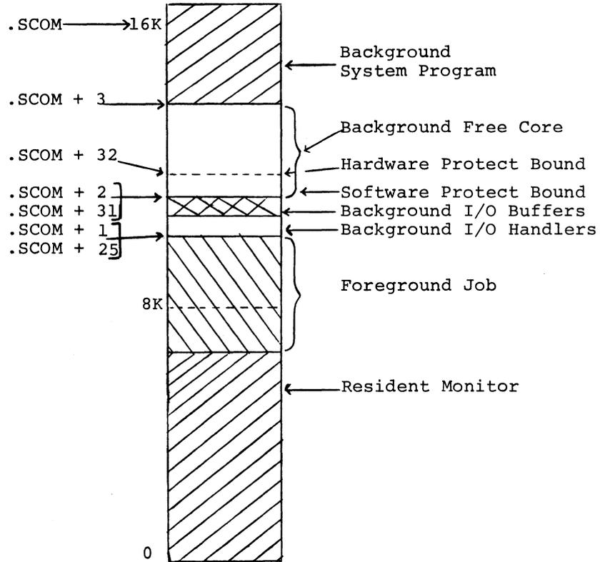
If the BACKGROUND request is for a system program, the System Loader loads the system program I/O handlers up from the top of the FOREGROUND job, allocates I/O buffer space, and loads the system program at the top of core (overlying the System Loader). Control is returned to the Resident Monitor, which sets the memory protect bound above the buffer space and gives control to the system program.
