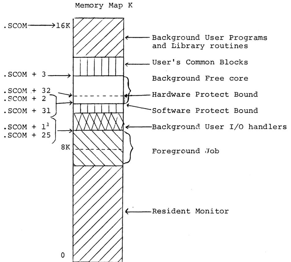
The .EXIT from the Linking Loader causes the user program I/O handlers to be block transferred to their running position, the memory protect bound to be set just above the I/O buffer space, and control given to the user program. If DDT was also loaded, it resides at the top of core, above the user programs. Its symbol table, built by the Loader, is block transferred by the Monitor to start at the software protect bound.
