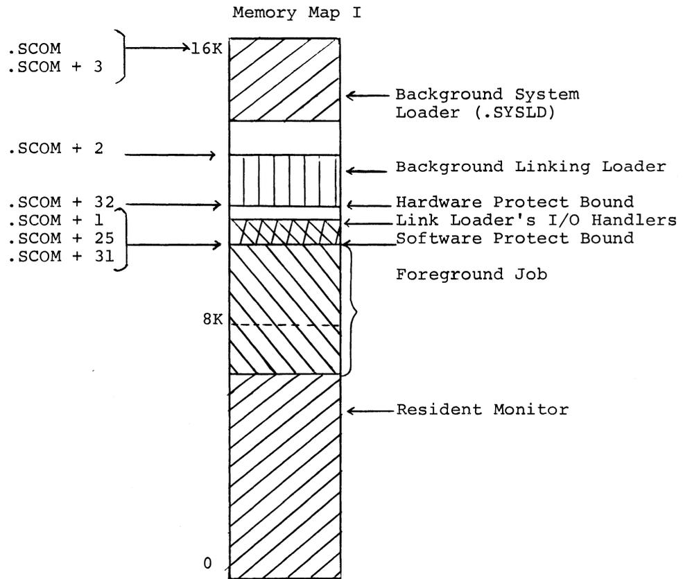
If the BACKGROUND program is a user program<sup>1</sup>, the System Loader loads the Linking Loader I/O handlers up from the top of the FOREGROUND job and loads the Linking Loader such that the memory protect bound can be set just below it.
