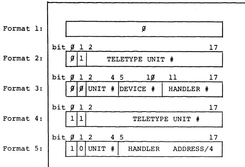
Formats 1 through 3 are the pre-setup stage (I/O handler linkage not established); Formats 4 and 5 are setup (I/O handler linkage established, handler is in core and I/O calls to such .DAT slots will be honored by the Monitor). Bit 0 distinguishes Formats 1 through 3 from 4 and 5.
