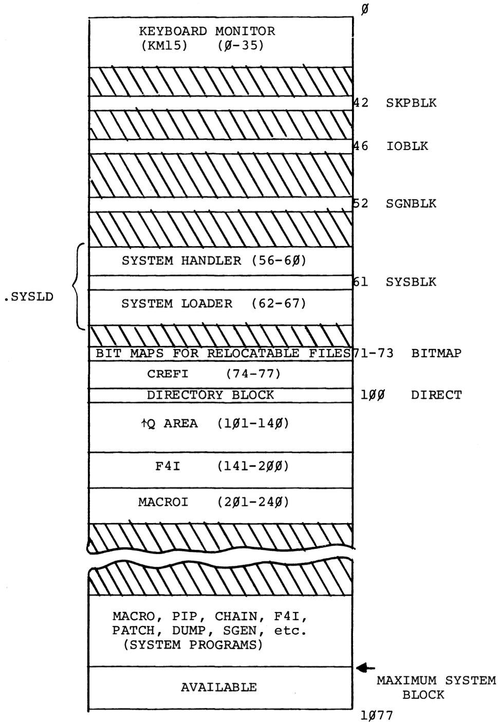
Figure 3-1. 8K System Tape Allocations
