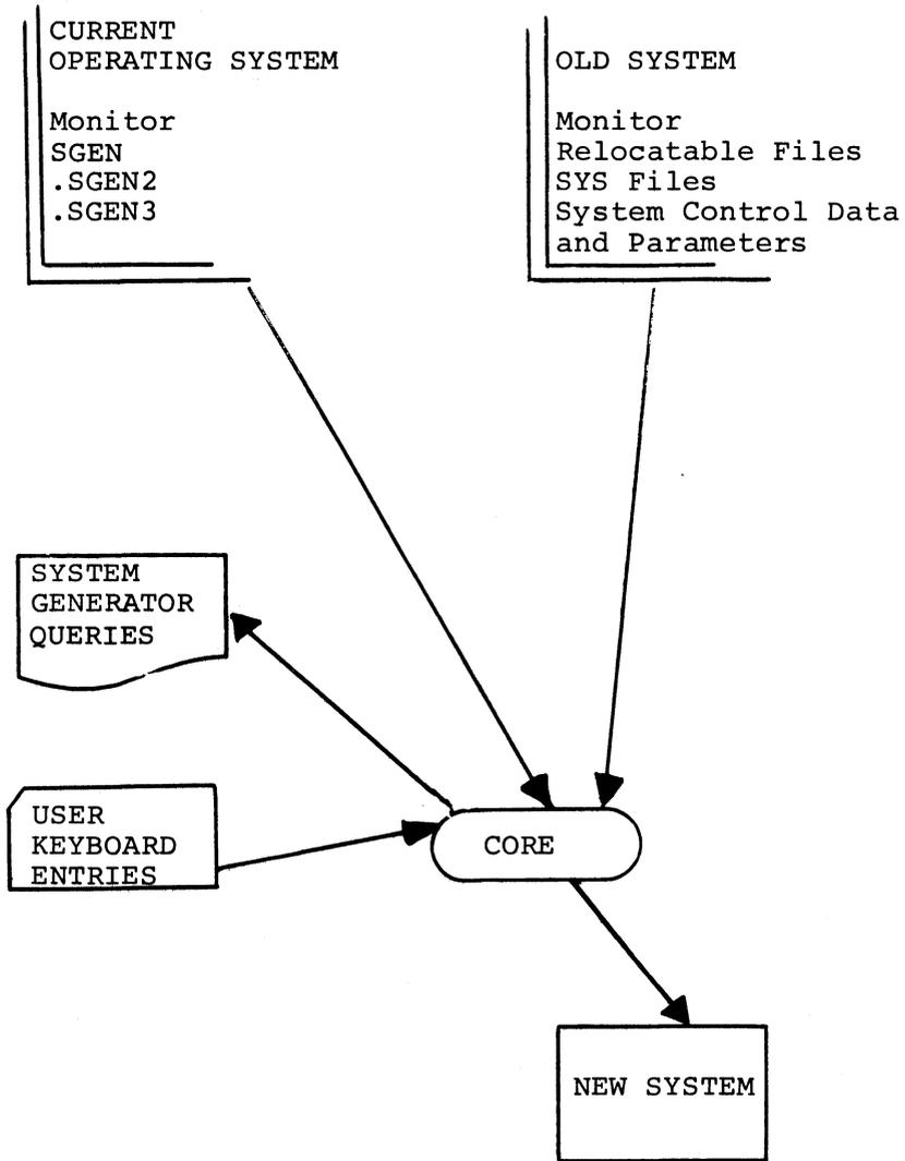
Figure 1-1. SGEN Operations, Information Flow Diagram
