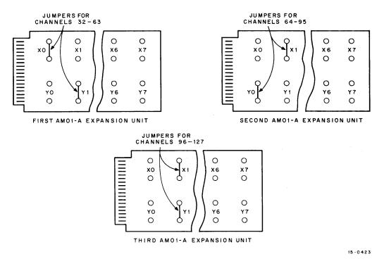
Figure 4-1 Jumper Connections for G729 Card
