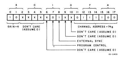
Figure 3-5 Example of Program Control Input Status Word
