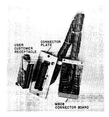
Figure 1-4 BC01P-4 Cable Assembly
