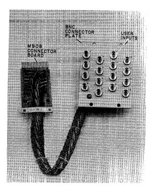
Figure 1-5 BC01N-4 Cable Assembly
