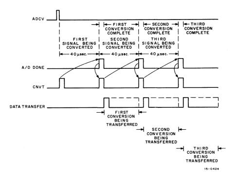
Figure 2-4 Sequential Mode Timing Relationships
