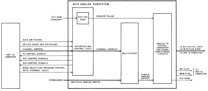
Figure 1–2 AD15 System Block Diagram
