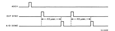
Figure 2-3 External Sync Timing Diagram
