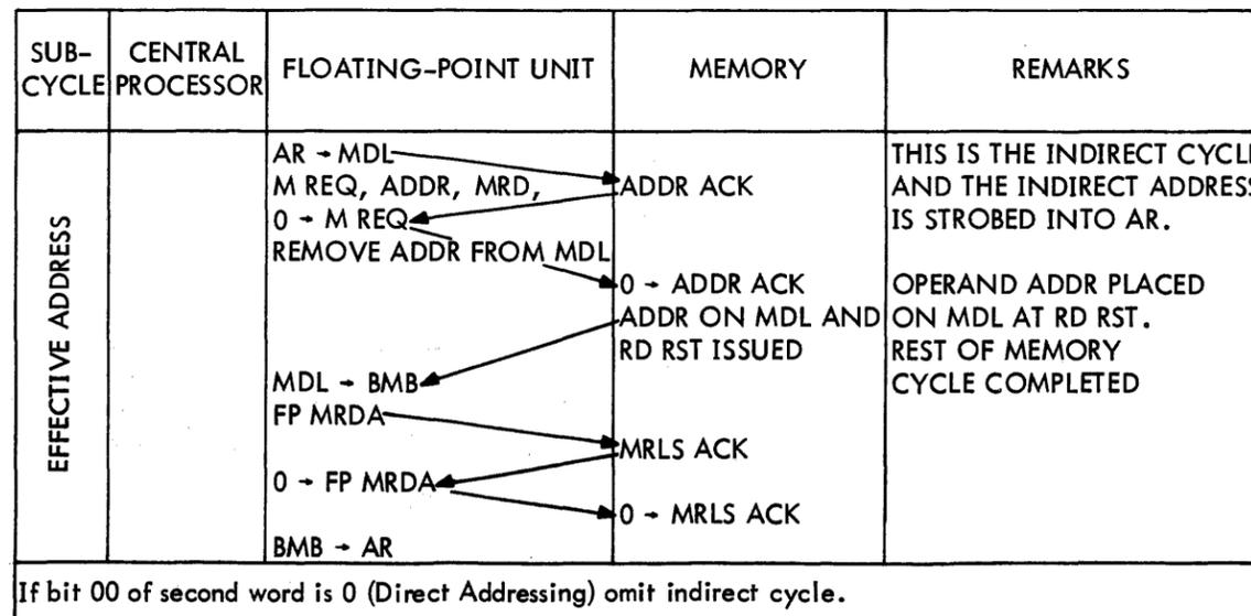
Figure 3-3 Memory Interface--FETCH Cycle (Indirect)
