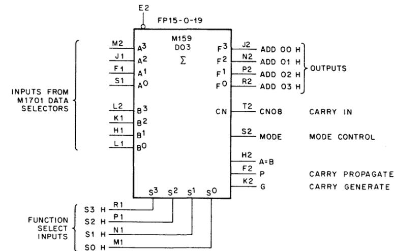
Figure 2-2 M159 Arithmetic Logic Unit
