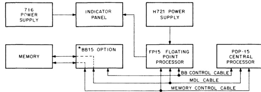
\*If BB option is not installed, cables are directly routed to memory.
