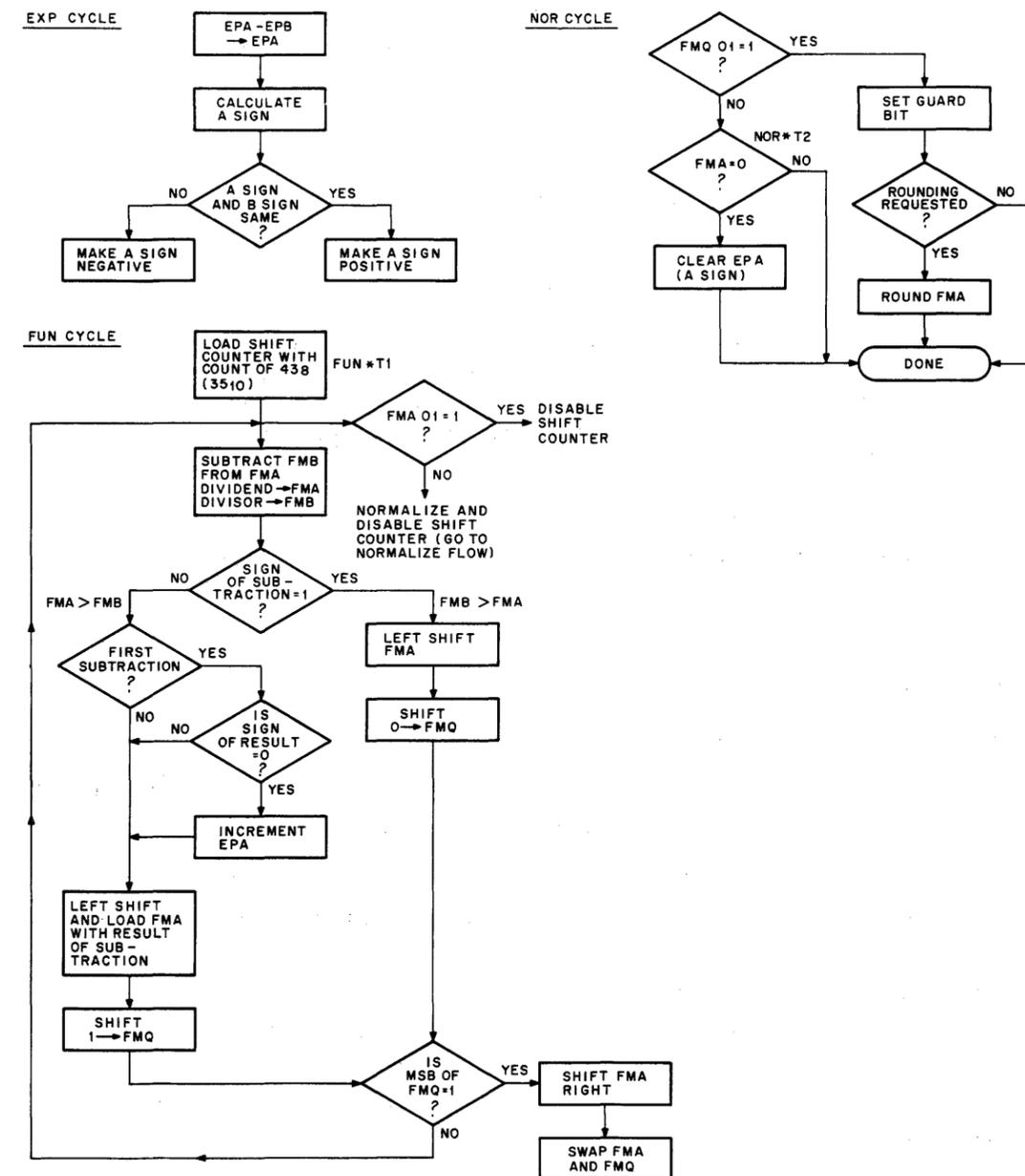
Figure 4-6 Floating-Point Divide Simplified Flow Diagram
