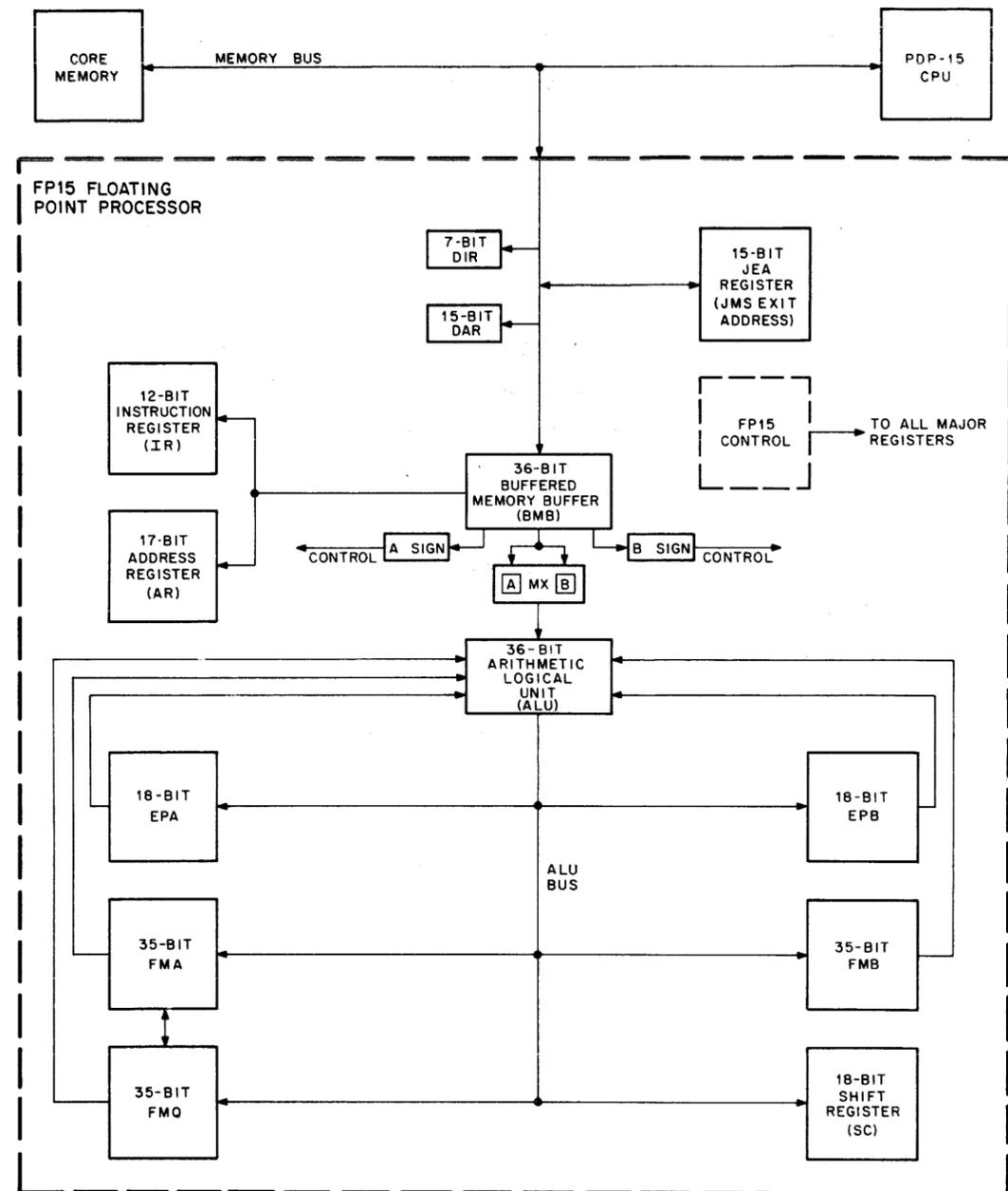
Figure 1-3 FP15 Functional Block Diagram
