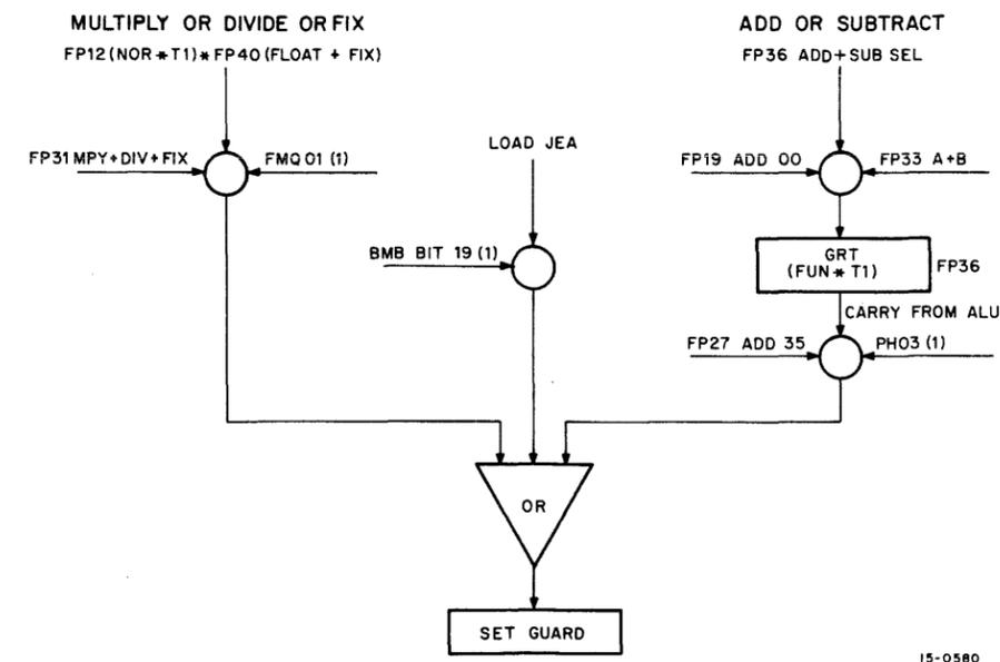
Figure 4-3 Flow Diagram for Setting Guard
