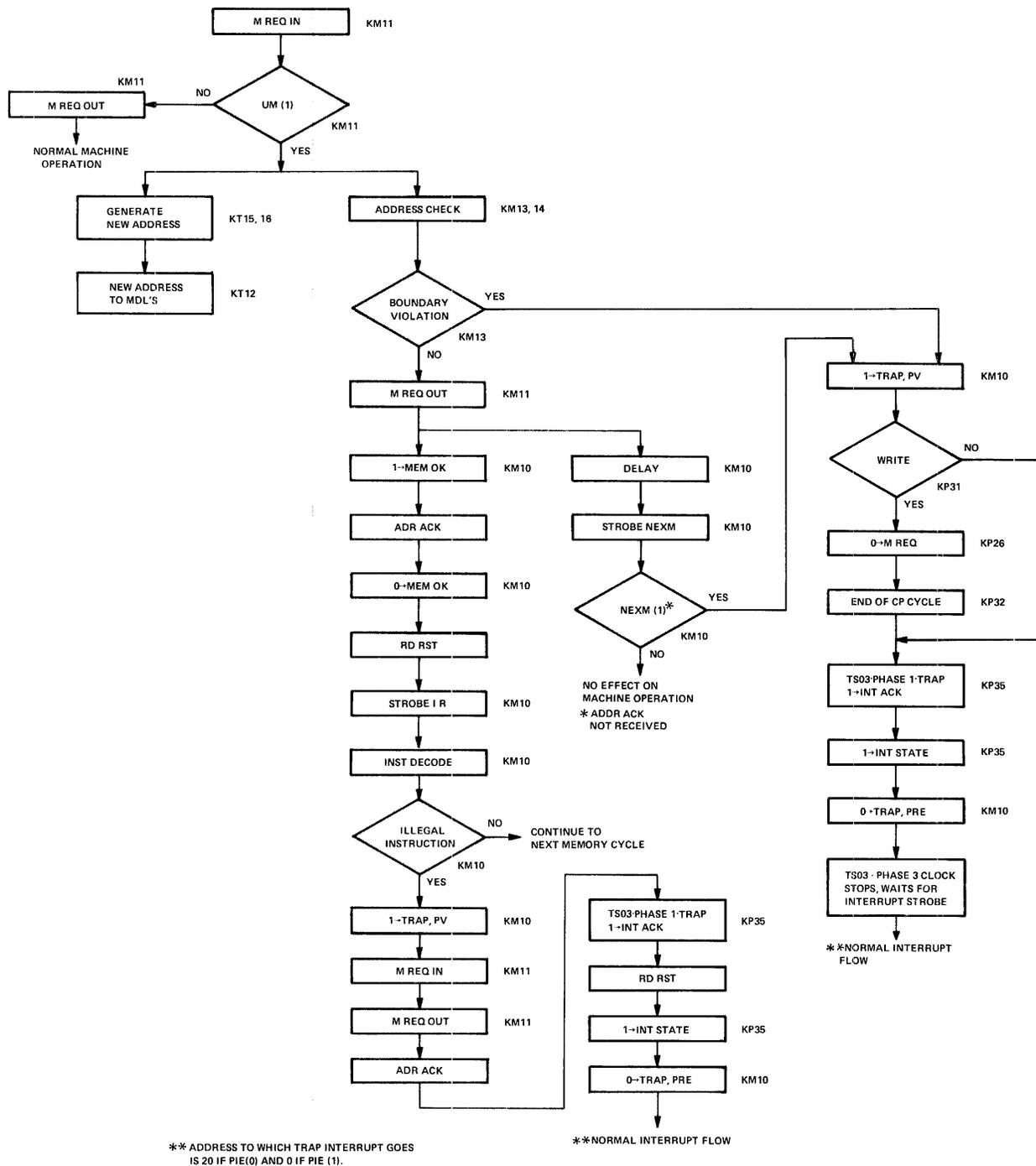
Figure 6-13 KT15 Memory Protect/Relocate Flow Diagram
