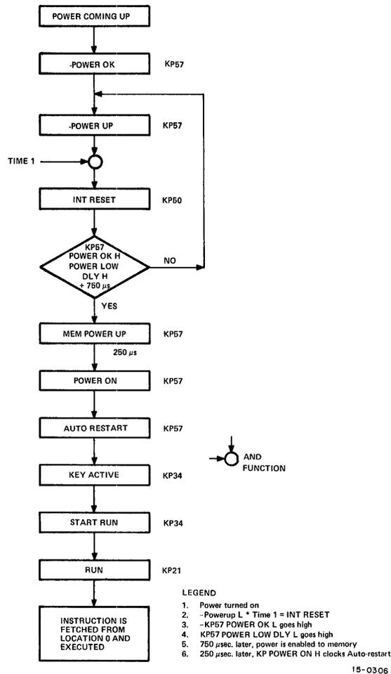
Figure 6-8 Power Restore Sequence With Power Fail Option Enabled, Flow Diagram
