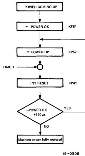
Figure 6-6 Power Restore Sequence With Power Fail Option Disabled, Flow Diagram
