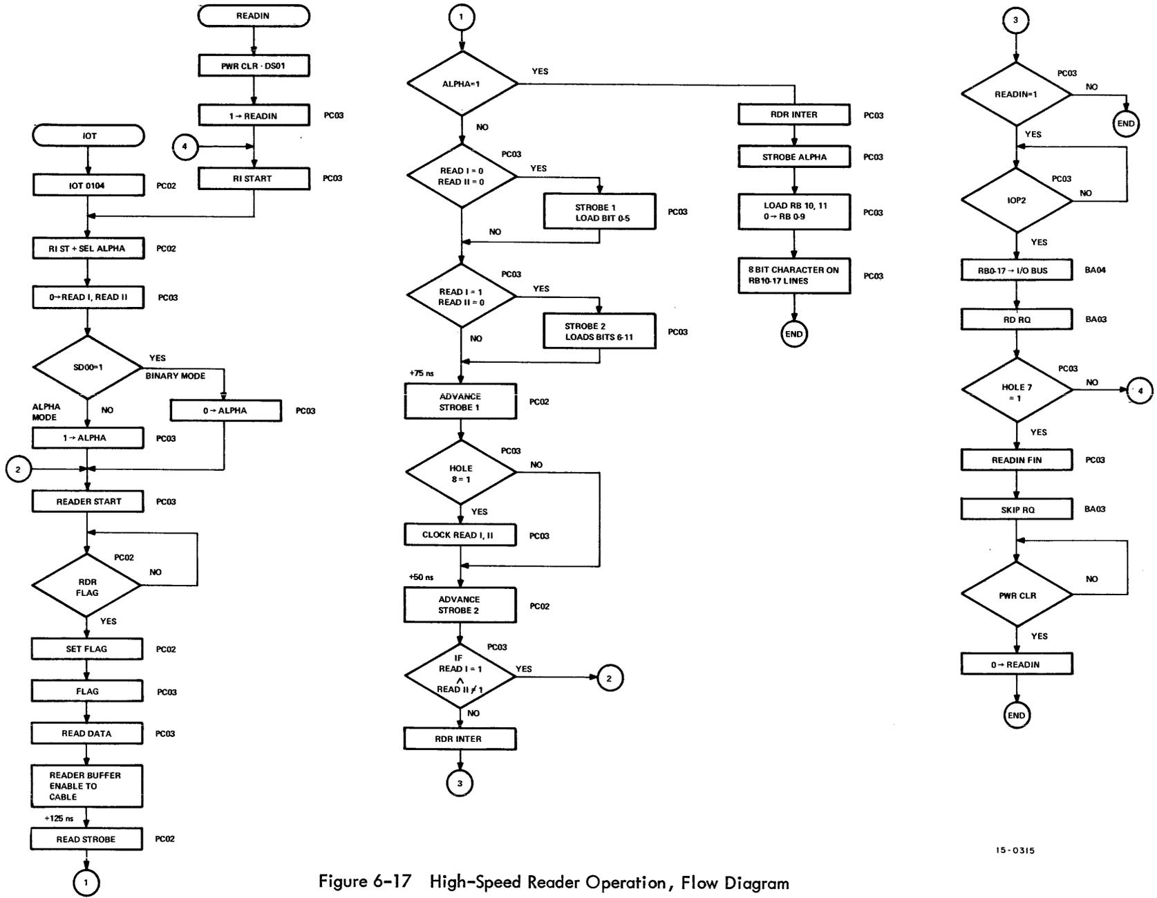
Figure 6-17 High-Speed Reader Operation, Flow Diagram
