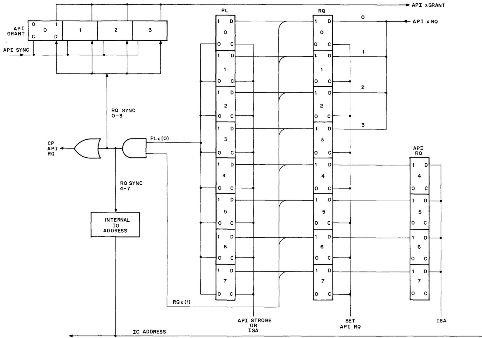
Figure 6-10 API Block Diagram
