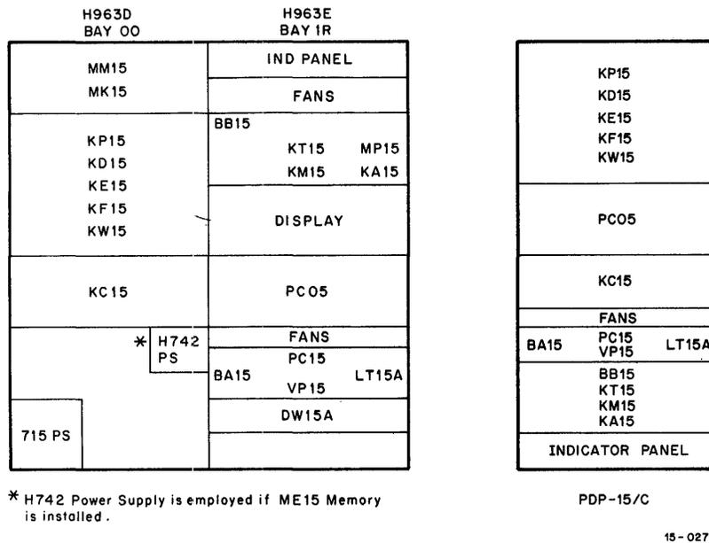
Figure 1-1 PDP-15 Configuration
