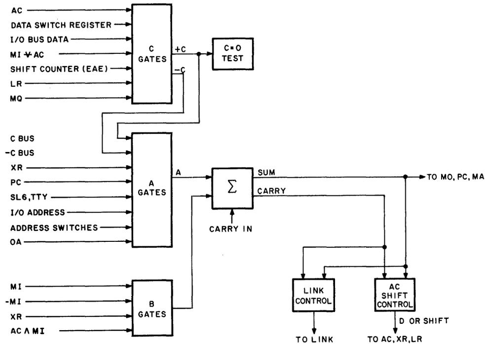
Figure 3-1 CPU Bus Structure
