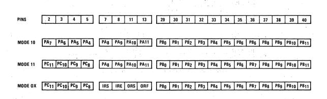
FIGURE 7: IM6103 PIO port pin assignments.
