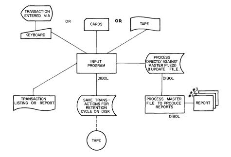
This figure illustrates of the input data (transaction file) from terminal, card reader of DECtape; the processing against the master file by a user created DIBOL program and the output (depending on the DIBOL program being run) of reports and files.
