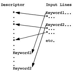
There is a current asterisk record pointer in BUILD which keeps track of the next asterisk record to be filled. After inputting the last \* record, BUILD goes back to the first one.
