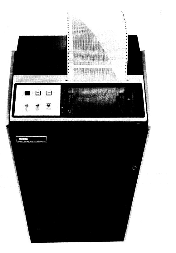
Figure F-6. LP08 80-Column Line Printer
