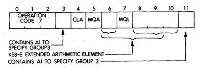
Figure 3-4 Group 3 Operate Microinstruction Bit Assignments
