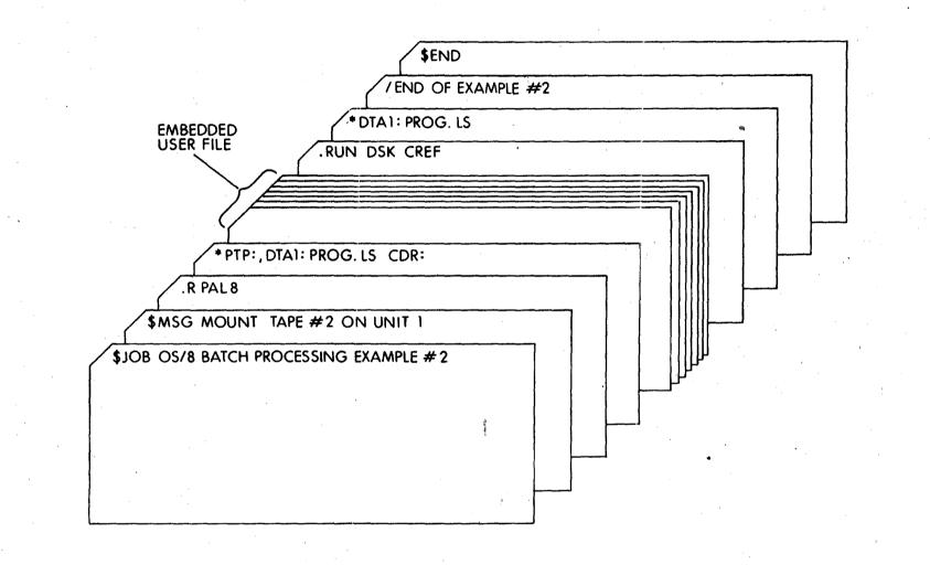
Figure 2-2 Punched Card Input File
