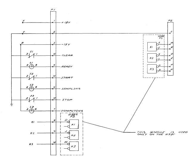
Figure 6–30 D–BS–H300–0–2 H301 Cable Connector Diagram
