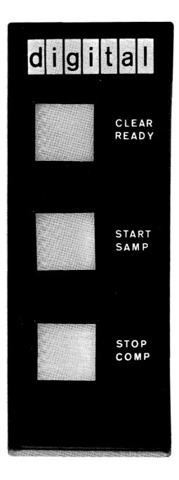
Figure 2-1 H300 and H301 Local Operator Console
