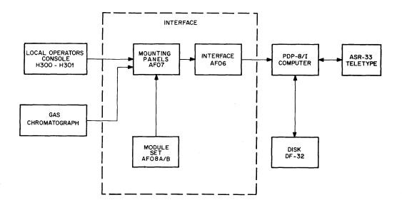
Figure 1–2 GLC–8 System Simplified Block Diagram
