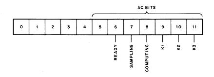
Figure 2–3 Digital Output Register Bit Assignment Diagram
