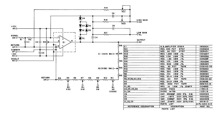
Figure 6-34 B-CS-A212-0-1 A212 Variable Gain Amplifier Circuit Schematic
