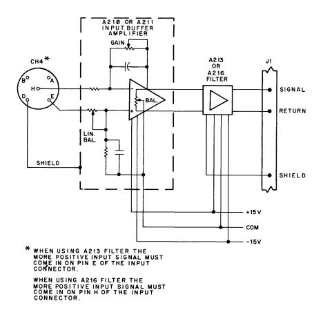
Figure 3-12 Input Buffer Amplifier, Simplified Diagram
