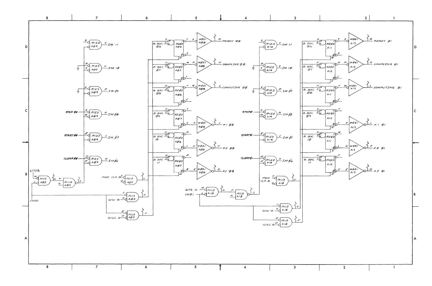
Figure 6–8 D–BS–AF17–0–3 LOC Control Logic (Ch. 00 to 07) Block Schematic Diagram (Sheet 1)
