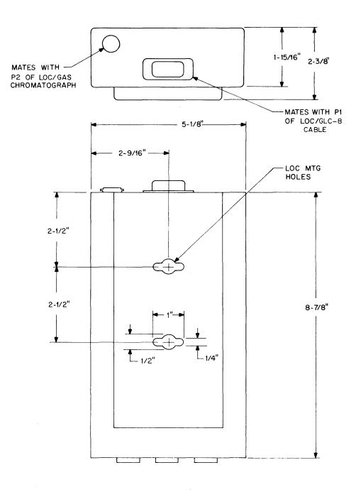
Figure 4-2 Local Operator Console, Outline Drawing
