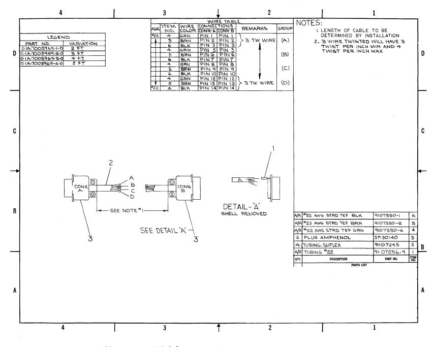
Figure 6-14 C-IA-7005969-0-0 H303 Amplifier Mounting Panel Cable Assembly Diagram
