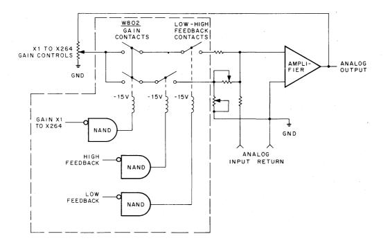
Figure 3-8 AG04 Variable Gain Amplifier, Simplified Diagram
