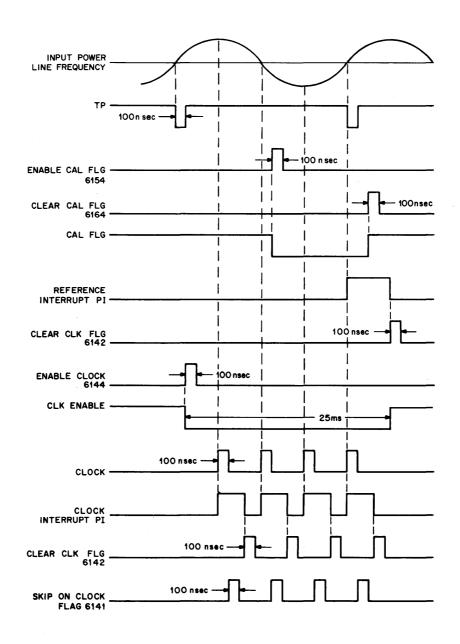
Figure 3-9 DK01A Timing Diagram
