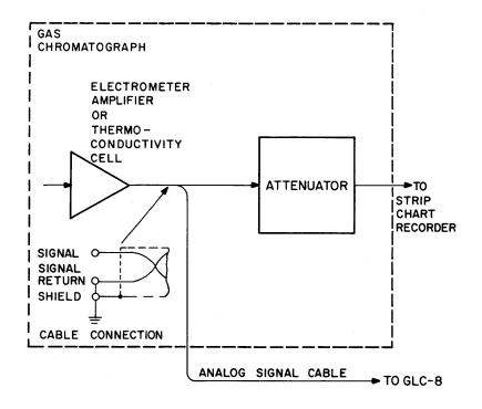
Figure 4-6 Installation of Analog Cable Assembly
