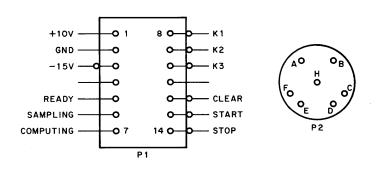
Figure 5–1 H300 and H301 LOC Cable Connectors
