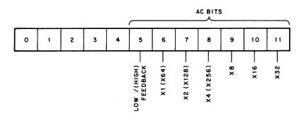
Figure 2–2 AG04 Variable Gain Amplifier Control Bit Assignment
