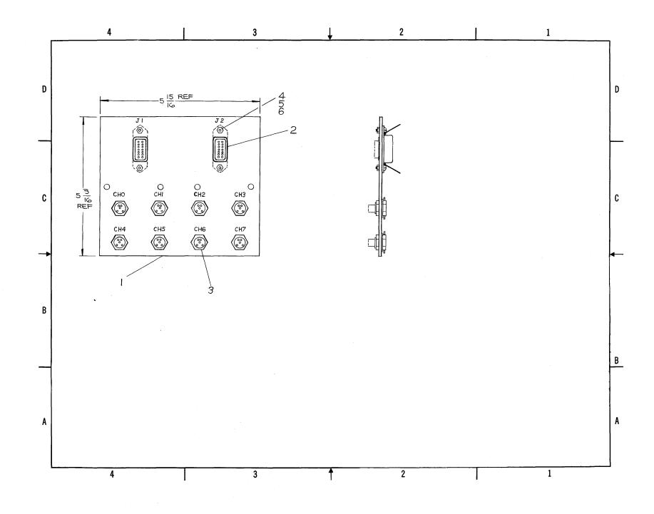
Figure 6-13 C-AD-7005925-0-0 H303 Amplifier Mounting Panel Connector Location Diagram
