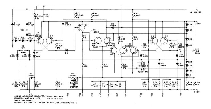
Figure 6-48 B-CS-R303-0-1 R303 Integrating One-Shot Multivibrator Block Schematic Diagram
