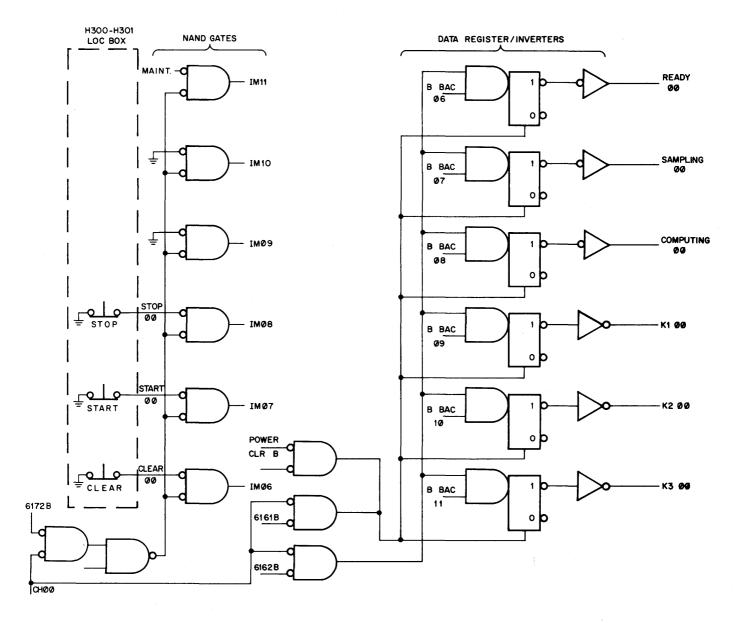
Figure 3–7 AF17 LOC Control Logic, Simplified Diagram
