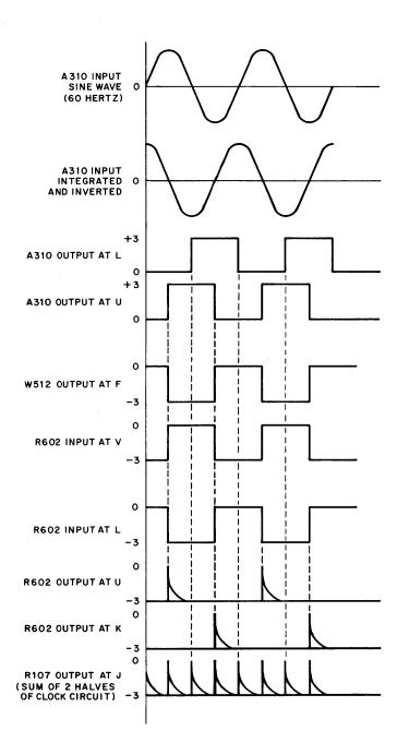
Figure 3–10 Four Times Line Frequency Clock Pulsetrain
