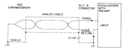
Figure 4-7 Common Mode Noise Analysis Test Setup
