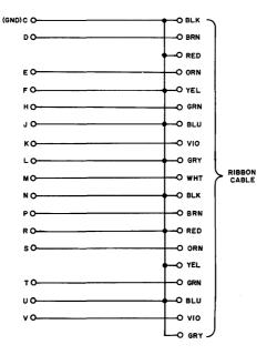
Figure 6–26 B–CS–W021–1–0 W021 Signal Cable Connector Block Schematic Diagram
