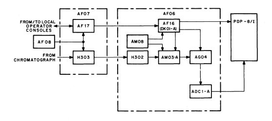
Figure 3-2 AF06, AF07, and AF08 Interconnection Diagram
