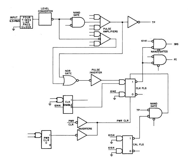
Figure 3-11 Four Times Line Frequency Clock, Simplified Diagram
