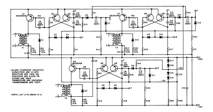
Figure 6-54 B-CS-W640-0-1 W640 Pulse Amplifier Block Schematic Diagram
