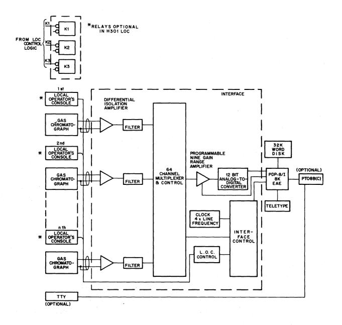
Figure 3-1 System Configuration
