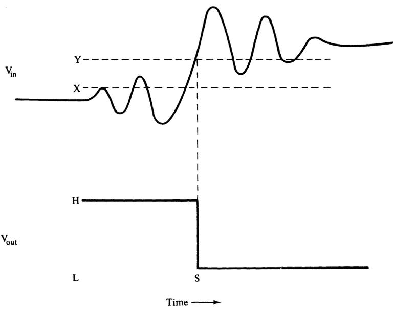
**Figure 12-8.** How the Schmitt trigger removes noise.
