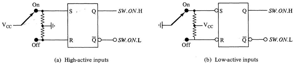
**Figure 4–8.** Mechanical switch debouncing circuits using asynchronous RS flip-flops.
