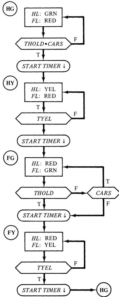
**Figure 6-17** The ASM for the traffic-light controller.
