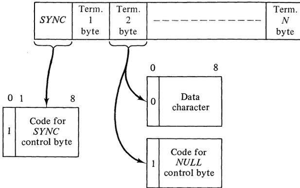
**Figure 11-12.** The frame structure for the terminal multiplexer's high-speed transmissions.
