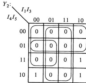
$$\overline{Y}_2 = \overline{I}_4 + I_3 + \overline{I}_1 \cdot I_5$$
