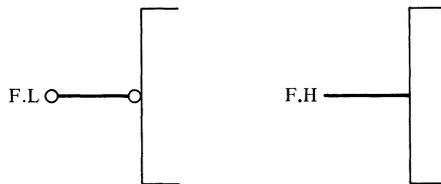
In this unchanging operation, the voltage on the wire never varies. For convenience, we sometimes show only the voltage level (H or L) on the diagram:
