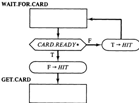
Figure 6-30 A segment of an ASM with an output race.
