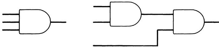
Figure 2-14. Realizing a 3-input AND.
