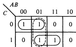
The theory is that a circuit based on the two solid loops may or may not contain a hazard; however, if we build a circuit that includes the dashed loop, we can be sure that the circuit will have no hazards. Using the dashed loop requires extra hardware (additional AND and OR gates), a necessary penalty when we cannot tolerate hazards.
