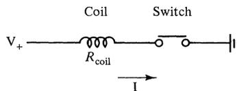
With the switch closed, the current is given by Ohm's Law:
