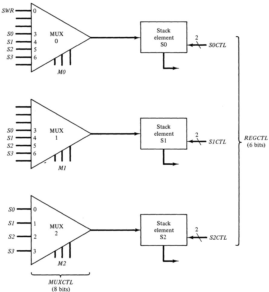
Figure 10–15 The architecture of a microprogrammed design.
