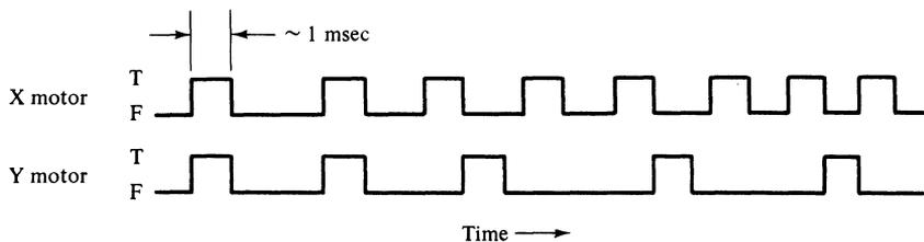
**Figure 11-9.** Typical signal patterns for the independent X and Y stepping motors.
