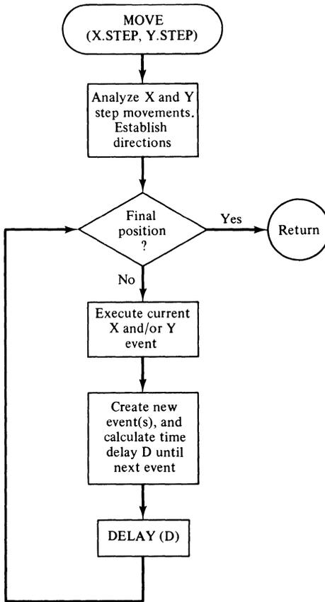
**Figure 11–10.** Flowchart of the sub-program MOVE for controlling the simultaneous movement of the X and Y stepping motors.
