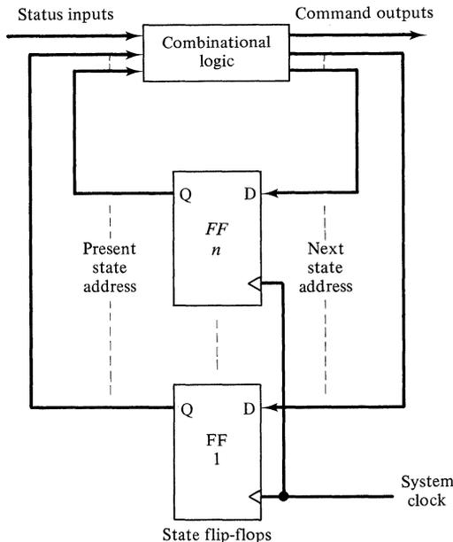
**Figure 5-10.** A model of an encoded ASM state generator.
