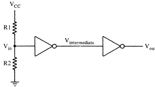
By proper choice of the resistors  $R1$  and  $R2$ , we can set the input voltage  $V_{in}$  such that  $V_{out} = V_{in}$  and  $V_{intermediate} \approx V_{in}$ . Both inverters are in their transition region. Now, if we carefully connect the output to the input and remove the source of  $V_{in}$ , we will have constructed a crosscoupled flip-flop circuit that is metastable:
