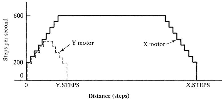
**Figure 11-8.** Acceleration and deceleration patterns of stepping motors.
