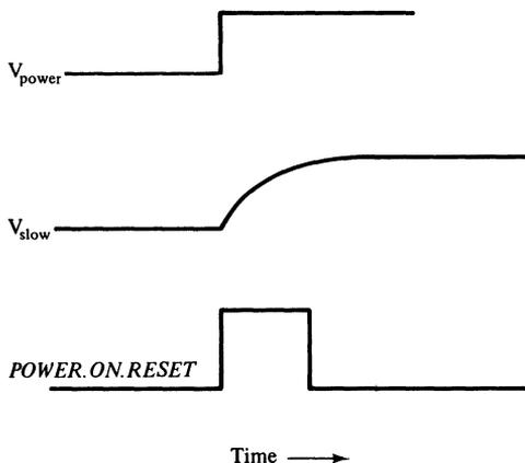
**Figure 12-9.** A power-on reset circuit.
