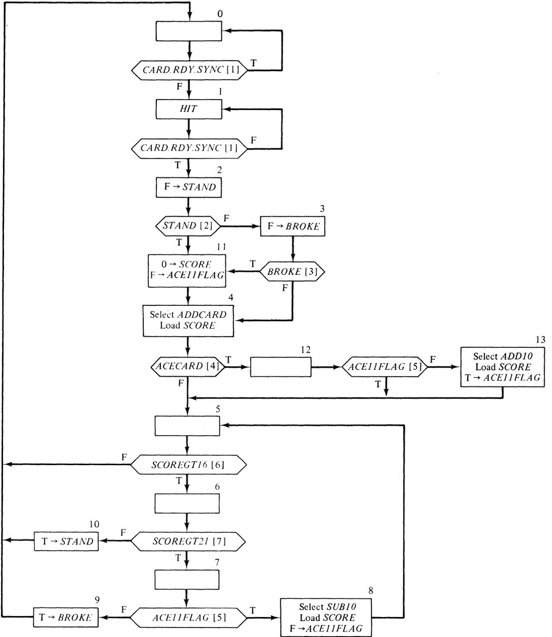
Figure 10-9 The Black Jack Dealer ASM revised for microprogrammed implementation.
