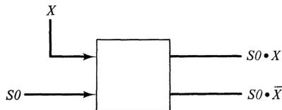
One such operation in each branching state will produce all the product terms required by the logic equations. If a state has no test input, we omit the square symbol, sending the raw state signal on to the right.
