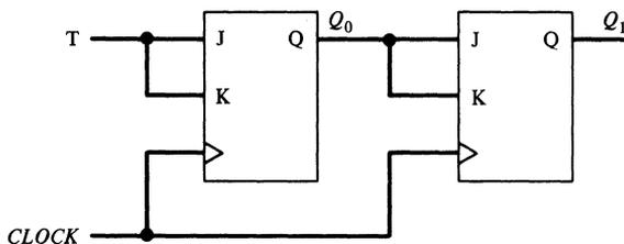
**Figure 4-13.** A two-bit binary counter. The least significant bit is on the left.
