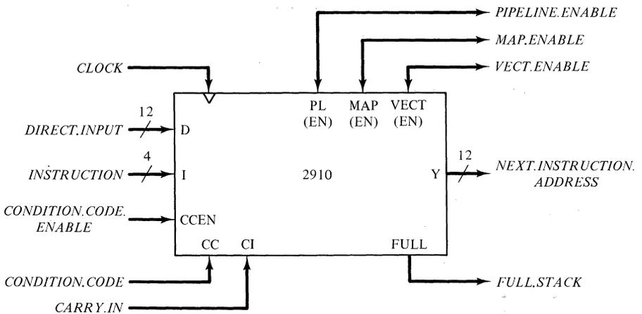
Figure 10-11 The 2910 microprogram sequencer.
