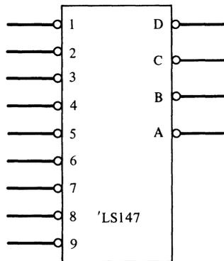
Figure 3–15. The 74LS147 Ten-Line-to-Four Line Priority Encoder.
