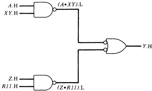
**Figure 2-6.** Schematic of  $Y = A \cdot XY + Z \cdot R11$ .
