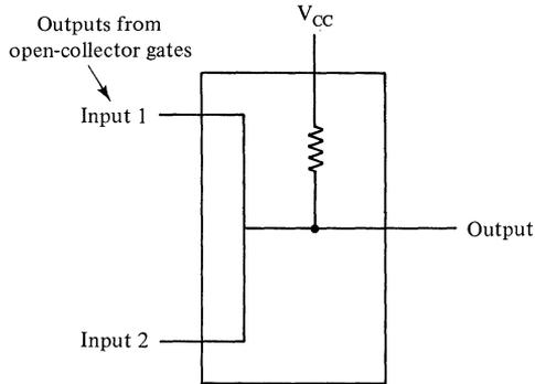
When two open-collector outputs serve as inputs to the box, the voltage table is:
