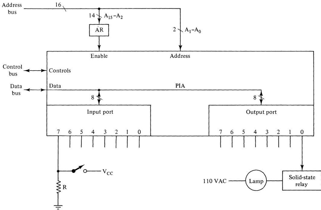
**Figure 11-3.** A switch operating a lamp, controlled by programmed input-output through a PIA.
