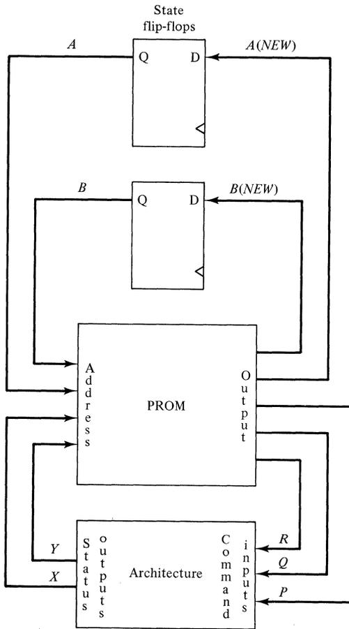
**Figure 10-4** A PROM-based micro-programmed implementation of Fig. 10-2.
