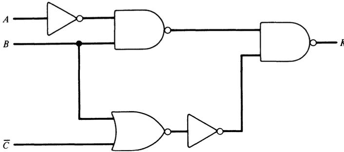
**Figure 2-21.** A circuit in the positive-logic convention. The circles represent logic inversions.
