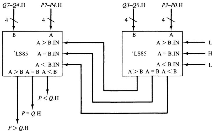
Figure 3-17. An 8-bit magnitude comparison using the 74LS85.
