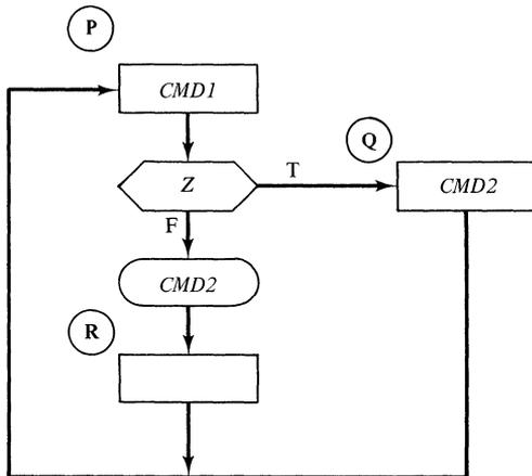
**Figure 5–8.** An ASM with a conditional output.
