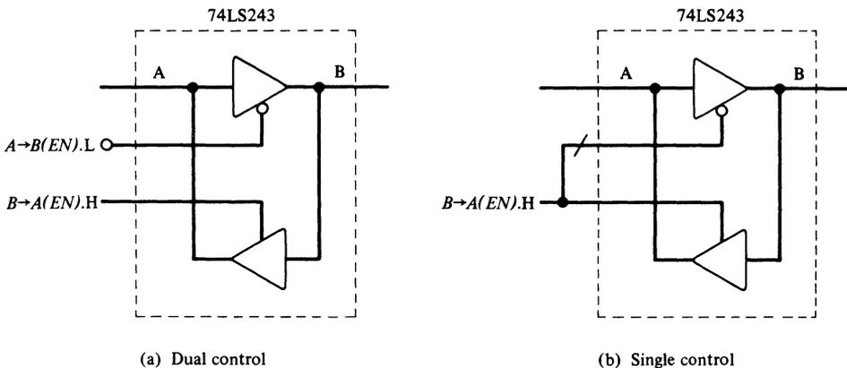
Figure 11–2. A bus transceiver in two configurations.
