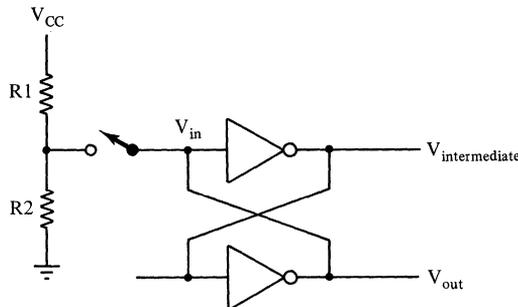
Eventually, electronic noise or the random thermal fluctuations of the atoms in the gates will upset the metastability and drive the outputs to a stable condition. The duration of the metastable interval is unpredictable. Real flip-flops always have feedback and can always be balanced at this metastable point. *There is no way to avoid this phenomenon!*
