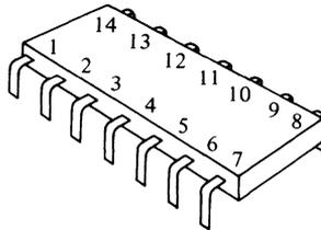
Operating power enters the chip through two pins,  $V_{CC}$  and GND (ground), usually at opposite corners. In the drawing, pin 7 is GND and pin 14 is  $V_{CC}$ . A chip may contain one or more independent logic elements.
