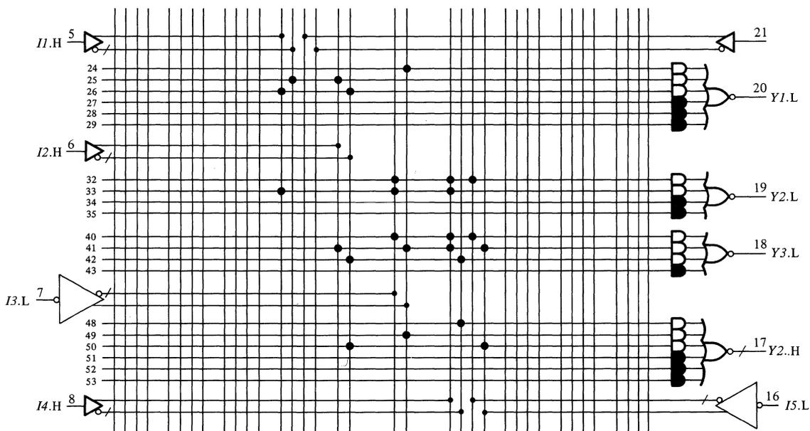
**Figure 4-26.** An implementation of Eqs. (4-1) through (4-3), using the PAL18L4. Note the mixed-logic changes to the diagram.
