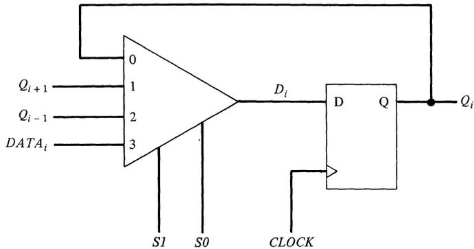
Figure 4–20. A typical bit  $Q_i$  of a general shift register.
