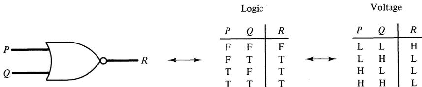
The name *Nor* derives historically from conventional positive logic, in which this chip performs the logical NOR (NOT OR) function.
