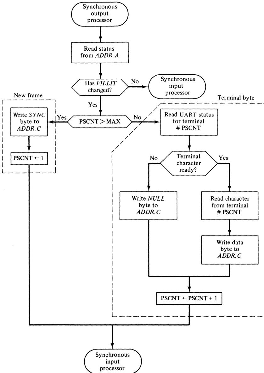
Figure 11-15. Algorithm for the terminal multiplexer: synchronous output (P → S) processing.
