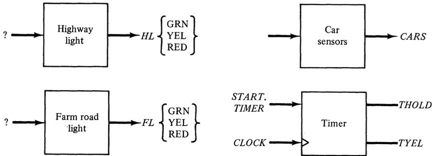
**Figure 6-16** The preliminary architecture of the traffic-light controller.
