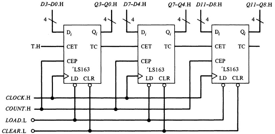
Figure 4-18. A 12-bit binary counter constructed with 74LS163 chips.
