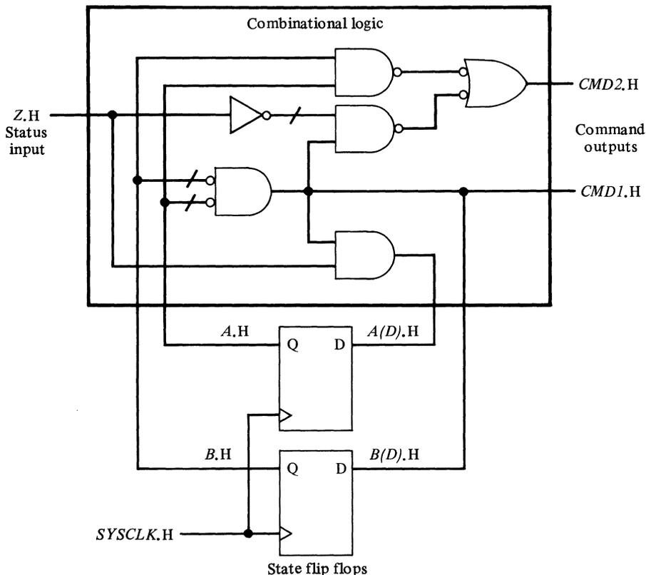
Figure 5-11. Traditional synthesis of the ASM in Fig. 5-9.
