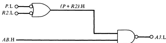
**Figure 2-7.** Schematic of  $A3 = (P + R2) \cdot AB$ .
