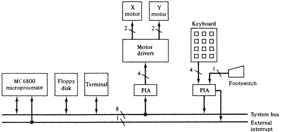
Figure 11-5. Signal paths for the wire-wrap controller.
