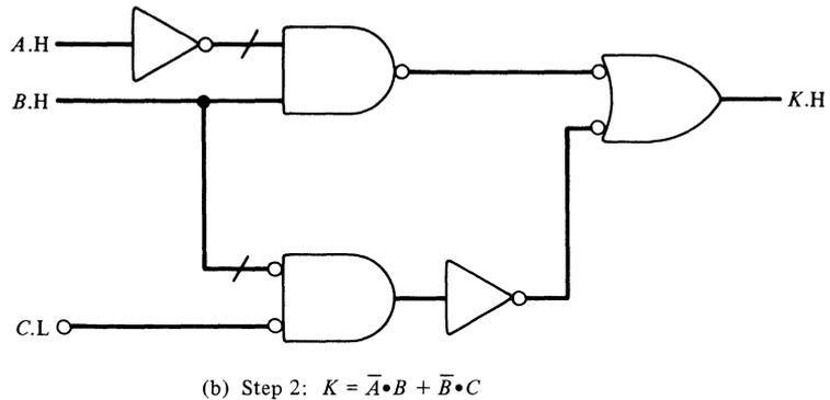
**Figure 2-23.** Converting Fig. 2-21 to mixed logic.
