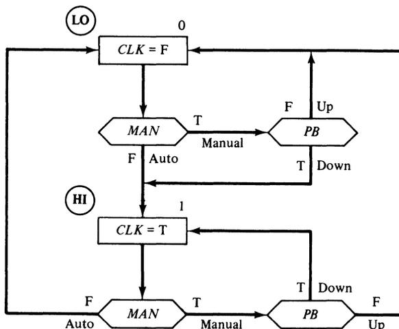
**Figure 6–5** An ASM of a system clock.
