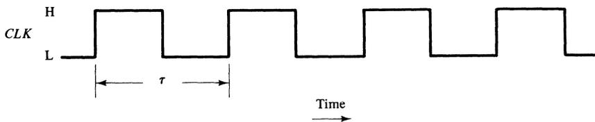
The clock event that triggers the transition from one state to another and other actions of the system is called the *active edge*, and in synchronous systems is usually the rising (L → H) edge of the clock. In a synchronous system, the clock will thus have  $T = H$ . Commonly, the clock period  $\tau$  ranges from 20 nanoseconds to several microseconds. The frequency  $f$  of the clock is its number of oscillations per second. Frequency and period are related by the expression
