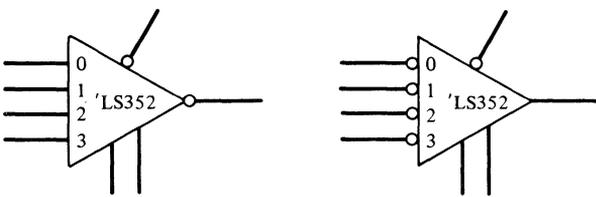
Figure 3-10. Mixed-logic symbols for the 74LS352 4-input multiplexer.
