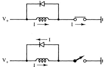
When the switch is closed, the diode is back-biased and no current flows through the diode. When the switch opens and the inductance tries to maintain the current, the voltage rises at the switch terminal, and the diode becomes forward-biased. Current can flow in a circular path through the diode until the inductive effect has dissipated. Therefore, no large voltage surge is developed across the switch.
