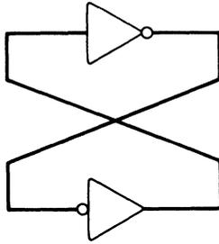
**Figure 4-3.** Memory displayed by a circuit with feedback.
