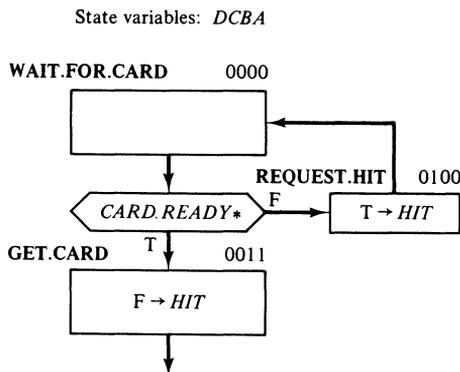
**Figure 6–29** A segment of an ASM with a transition race.
