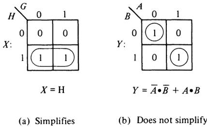
Figure 1-11. Simplifiable and unsimplifiable functions of two variables.
