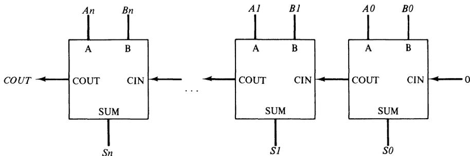
Figure 3-19. Addition with cascaded full adders.
