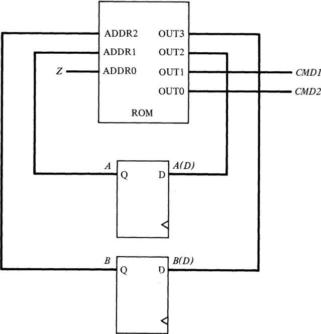
**Figure 5-16.** Implementation of the ASM in Fig. 5-9, using a ROM.
