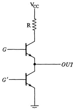
**Figure 12–4.** The TTL totem pole output configuration. The internal signals  $G$  and  $G'$  are complements of each other.
