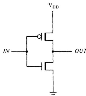
In this arrangement, one transistor is conducting whenever the other is shut off. When *IN* is a high voltage, the n-MOS transistor is on and the p-MOS transistor is off, producing a low voltage level at the output *OUT*. When *IN* is a low voltage, the n-MOS transistor is off and the p-MOS transistor is on, producing a high voltage level at *OUT*. Except during the brief instant of switching, no
