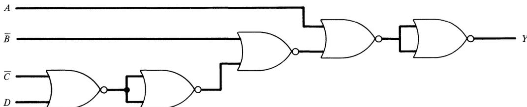
**Figure 2–19.** Positive-logic implementation of  $Y = A + B \cdot \overline{C} + \overline{D}$ , using De Morgan's law and Nor gates.
