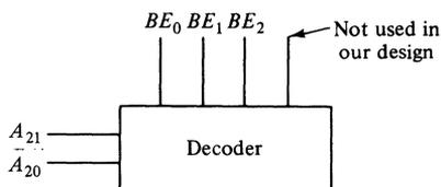
$BE_0$  enables the chips in bank 0,  $BE_1$  enables bank 1, and so on. A bank contains two RAM chips, since there are 2 bits per word. (The row-select and column-select control lines are not shown in the diagram.)
