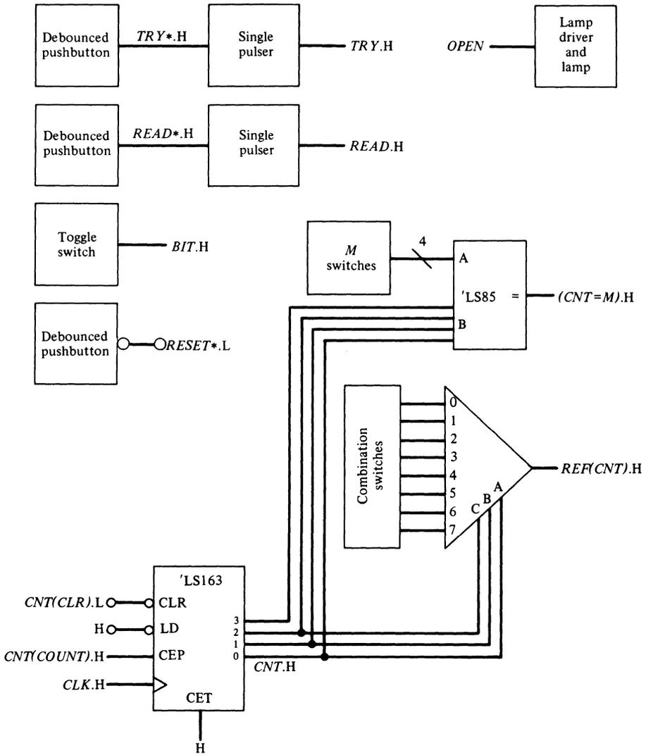
Figure 6-22 The architecture for an elegant combination lock.
