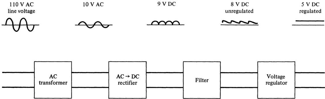
Figure 12–14. Components and waveforms of a dc power supply.
