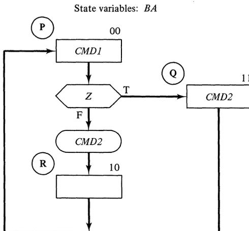
Figure 5-9. A simple ASM with a state assignment.
