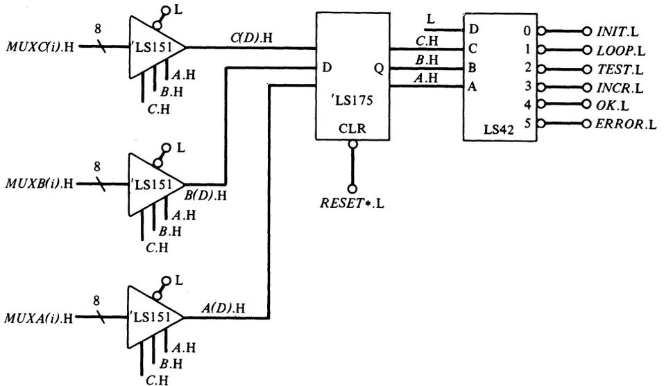
**Figure 6-23** A state generator for an elegant combination lock.
