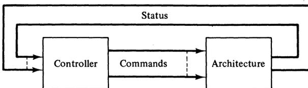
**Figure 5-1.** The structure of a state machine.
