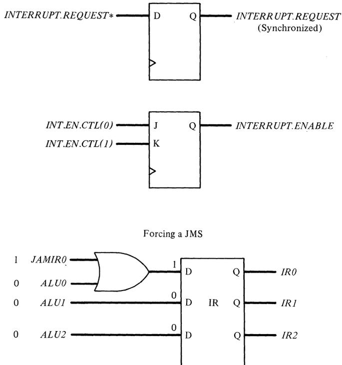
**Figure 10-22** Architecture of the interrupt system in the LD30.
