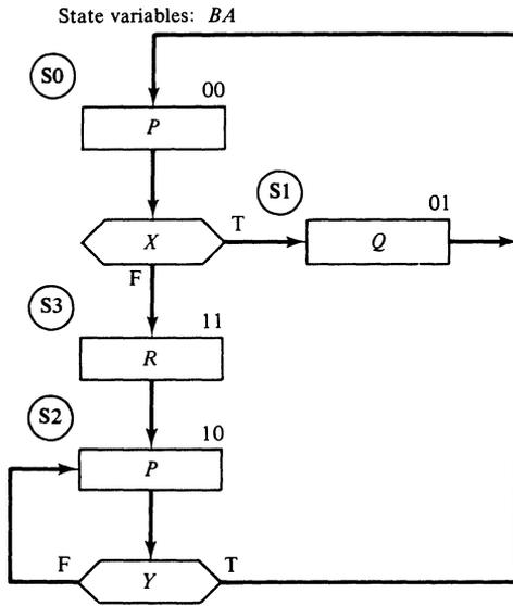
Figure 10-6 Figure 10-2 redesigned to have no conditional outputs.
