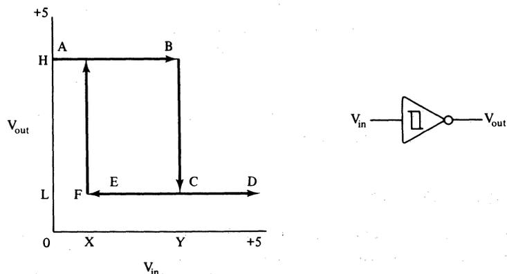
Figure 12-7. Voltage behavior and symbol of the Schmitt trigger.
