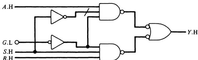
Figure 3-5. An enabled two-position electronic selector switch.
