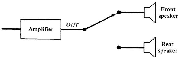
Figure 3-11. A mechanical distributor switch.
