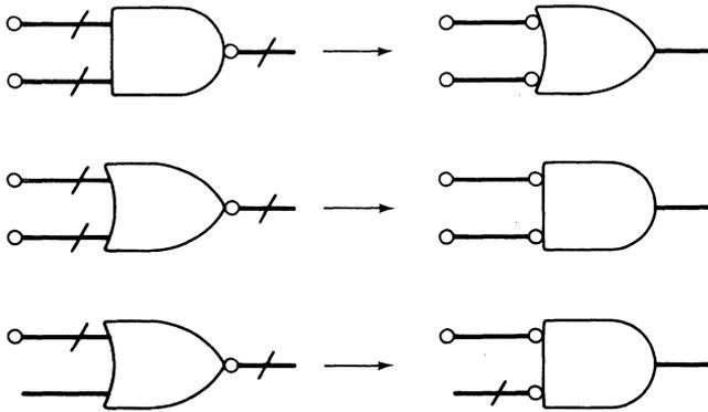
**Figure 2-22.** Some logic transformations on gates.
