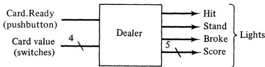
**Figure 6-25** The Black Jack Dealer's interface with the operator.
