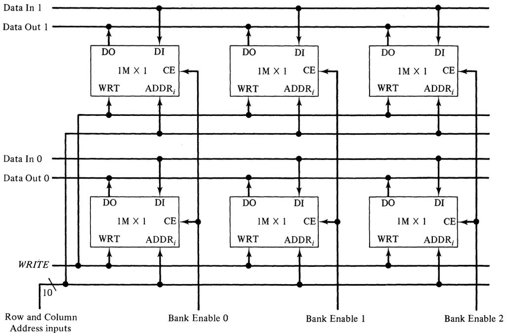
**Figure 4-22.** A  $3M$ -word by 2-bit memory constructed with  $1M \times 1$  RAM chips.
