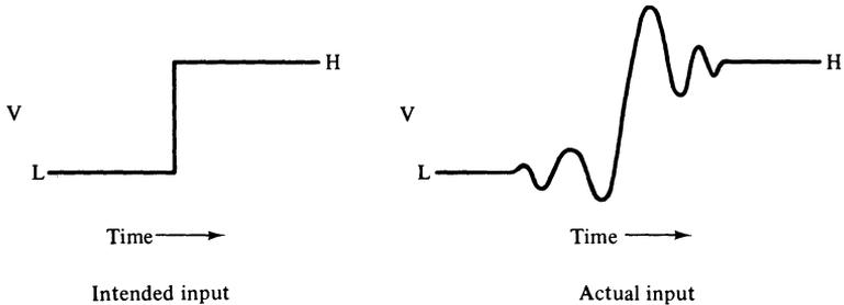
Let us put this waveform into a Schmitt trigger and see what happens. In Fig. 12-8, the sloppy input waveform with the Schmitt trigger switching voltages X and Y is shown. The input must rise to Y before the Schmitt trigger will switch. The hysteresis in the Schmitt trigger rejects all the noise in the lower part of the signal, and a clean switch occurs in the output at point S. Once switched,
