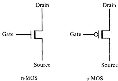
The drain voltage is  $V_{DD}$ ; the source voltage is  $V_{SS}$ . Typical n-MOS supply voltages are 0 volts for  $V_{SS}$  and 5 volts for  $V_{DD}$ . In good mixed-logic style, the circle shows that a low gate-voltage turns on the p-MOS transistor. In circuits that are entirely of one type of transistor, the distinguishing notations are often omitted.
