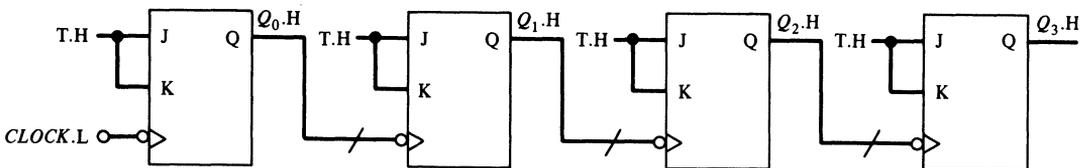
**Figure 4-16.** A 4-bit (modulo-16) ripple counter.
