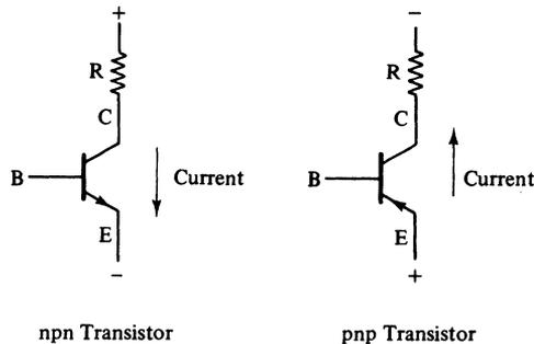
In each case the resistor R limits the current whenever the transistor is conducting; without the resistor, the transistor could be damaged. Most bipolar digital circuits are made with npn transistors. The positive supply voltage in these circuits is called  $V_{CC}$ .
