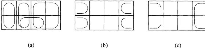
Figure 1-8. Typical circlings of K-maps of three variables.
