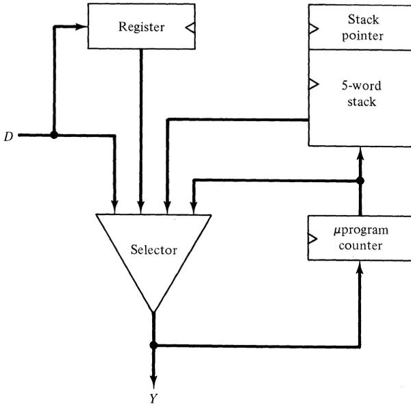
**Figure 10-12** Twelve-bit data paths in the 2910 microprogram sequencer.
