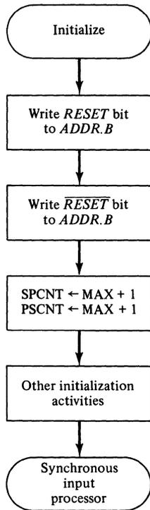
**Figure 11-17.** Algorithm for the terminal multiplexer: initialization.
