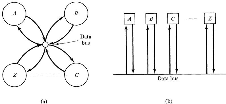
Figure 3–24. Two ways to view a data bus.
