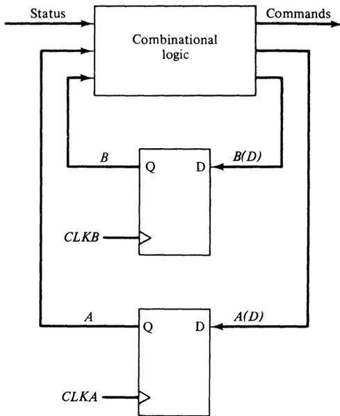
**Figure 5-17.** A model of a digital system for studying clock skew.
