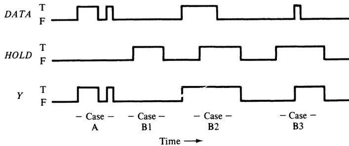
Figure 4-5. A timing diagram for a latch. Note the 1's catching behavior.
