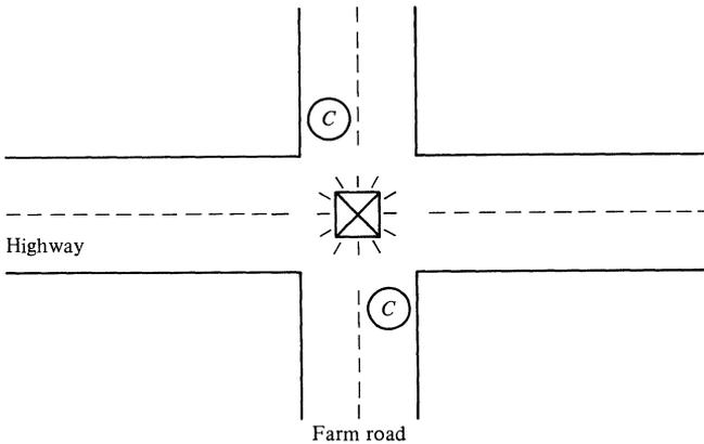
**Figure 6–15** The location of the traffic signal and the sensors in Design Example 5.
