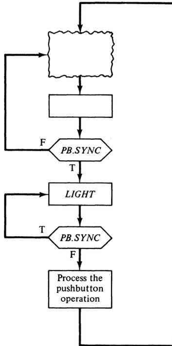
**Figure 6-4** Diagram of an ASM if the operator may press a pushbutton at any time. In this algorithm, the machine waits until the operator releases the button before it responds to the pushbutton.
