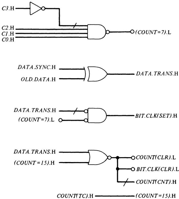
**Figure 6-10** Control signals for a serial bit clock.
