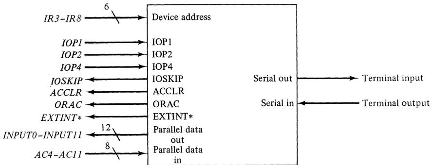
Figure 9-2 Interface signals in the LD20-terminal interface.
