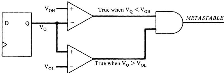
Figure 12-21. A simple metastability detector.
