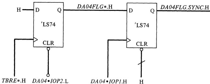
Figure 9-4 A circuit for *DA04FLG\**.
