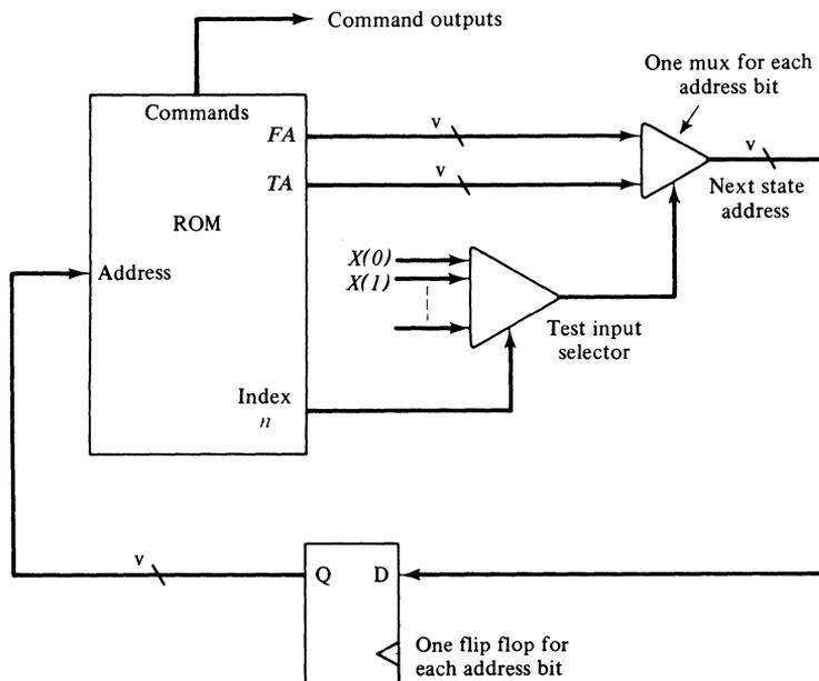
**Figure 10-5** A primitive microprogram controller with an input qualifier index and both true and jump addresses.
