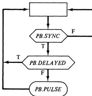
Figure 6-3 A single-pulser ASM in one state.
