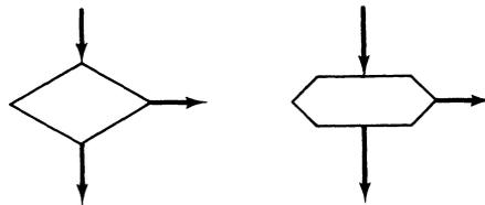
We incorporate this symbol into the ASM chart by appending it to a state rectangle, placing the description of the test input inside the diamond, as in Fig. 5-6. In this case a portrayal of the time line would be
