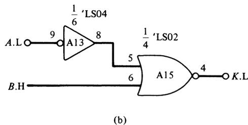
**Figure 2-15.** Two circuits for  $K = A + B$  with signals  $A.L$  and  $B.H$ . The diagrams in this section are fully labeled. The choice of a particular gate within a chip is arbitrary.
