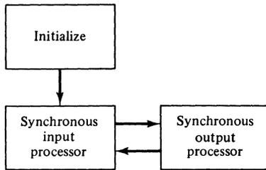
**Figure 11-14.** Algorithm for the terminal multiplexer: basic modules.
