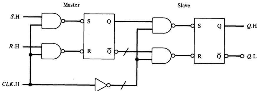
Figure 4-10. A master-slave clocked RS flip-flop.
