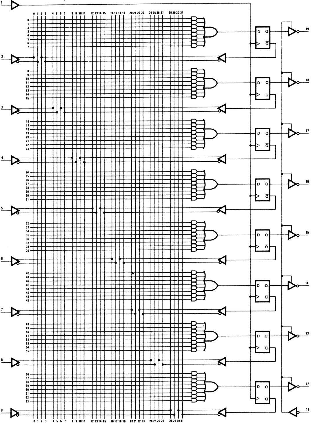
Figure 4-27. A PAL16R8. (Courtesy of Monolithic Memories, Inc.)
