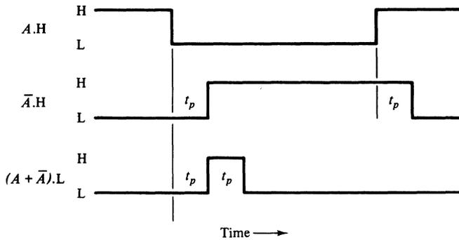
Figure 4-2. A hazard caused by propagation delay in an inverter.
