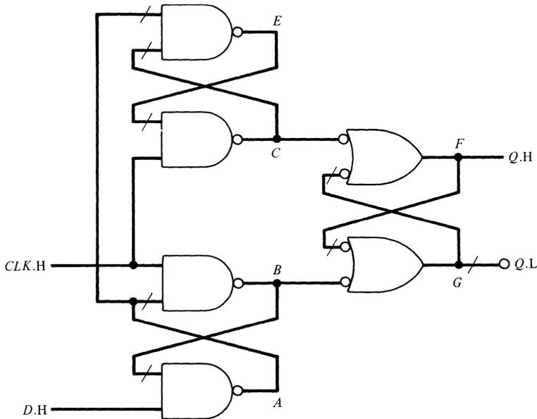
**Figure 4-30.** A 74LS74 D flip-flop without an asynchronous set and clear.
