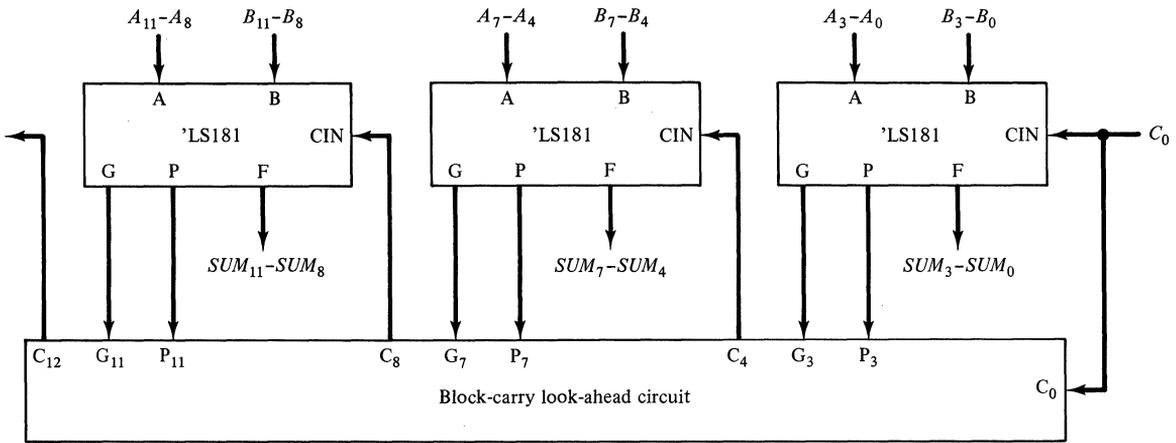
Figure 3-22. A 12-bit ALU containing a block-carry look-ahead circuit.
