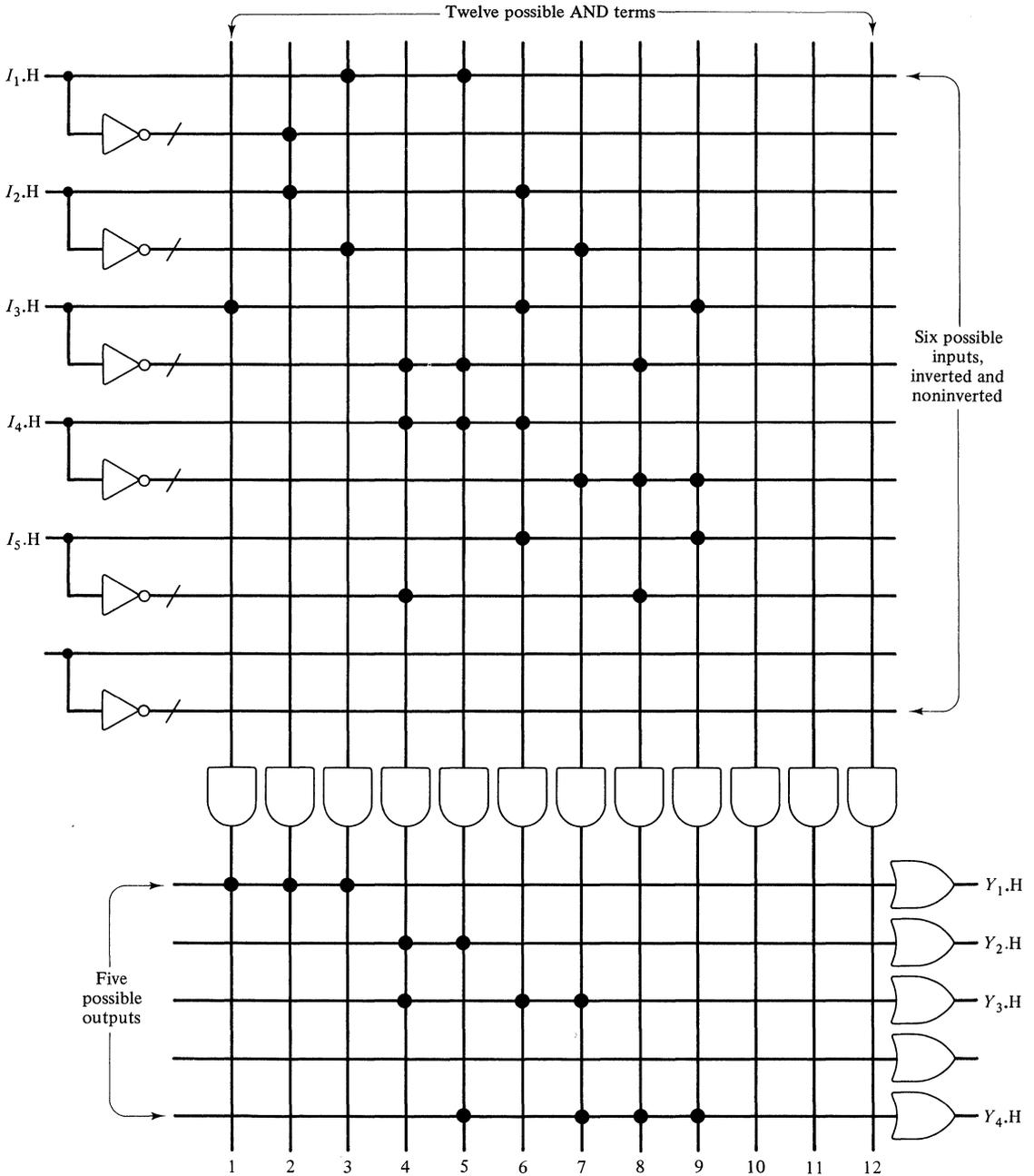
**Figure 4-24.** A PLA realization of Eqs. (4-1) to (4-4). The sixth input, the fourth output, and AND gates 10, 11, and 12 are not used. This PLA is smaller than commercial chips.
