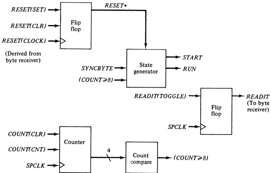
Figure 6-14 The logical structure of a serial-to-parallel converter.
