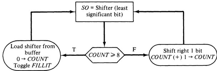
Figure 6-11 An ASM for parallel-to-serial conversion.
