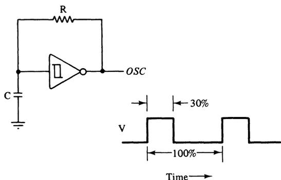
**Figure 12-10.** A simple Schmitt trigger oscillator. R and C control the frequency.
