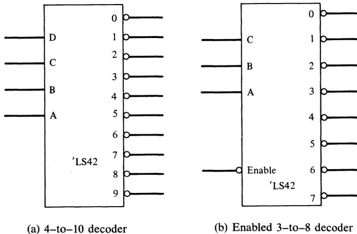
Figure 3-14. Two uses of the 74LS42 decoder.
