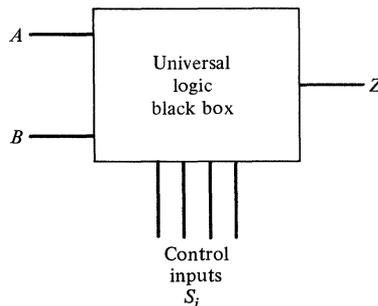
**Figure 3-18.** Inputs and output for the universal logic circuit.
