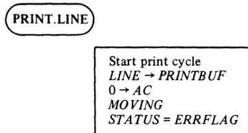
Figure 5-5. ASM output notations.
