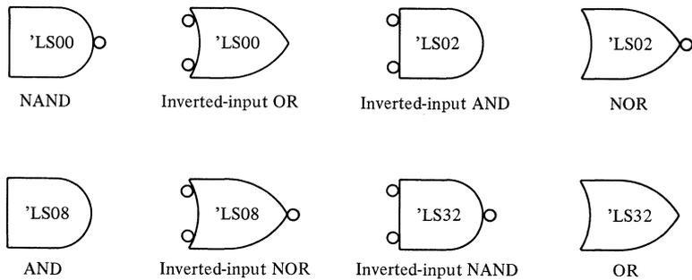
**Figure 2-18.** Interpretation of gates in the positive-logic convention.
