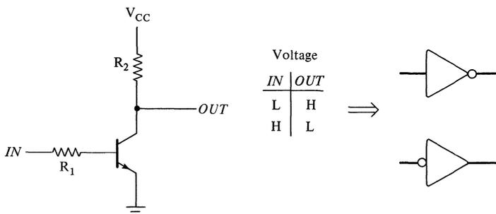
Figure 12–1. An npn transistor used as an inverter.
