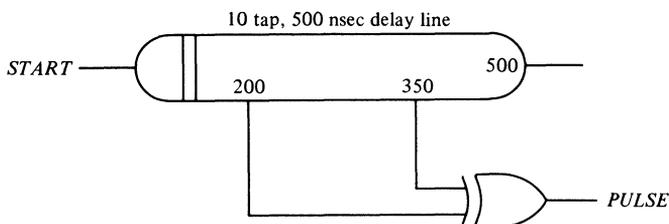
**Figure 4–29.** A circuit for a delay line to produce a 150-nsec pulse delayed by 200 nsec.
