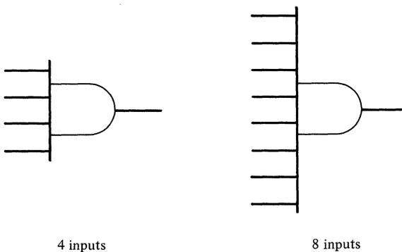
**Figure 2-1.** Symbols for AND with multiple inputs.
