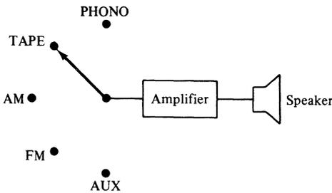
Figure 3-1. A mechanical selector switch.
