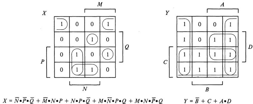
Figure 1-13. Simplification of two functions of four variables.
