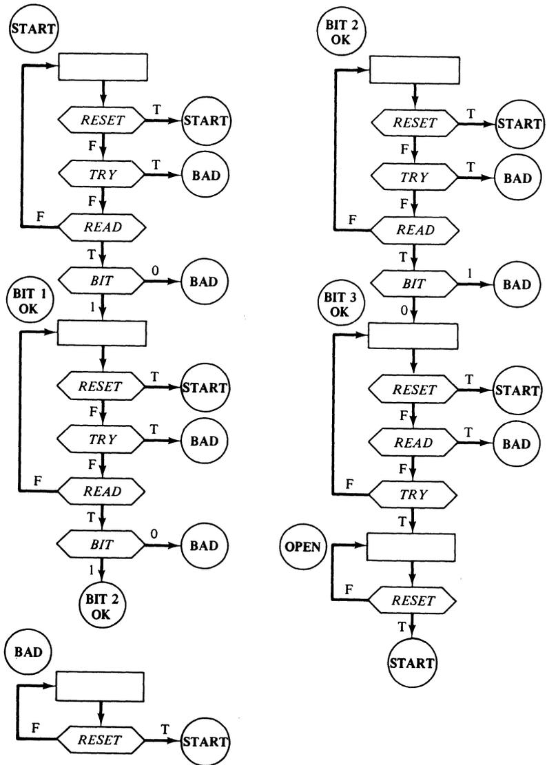
Figure 6-20 An ASM for a primitive combination lock.
