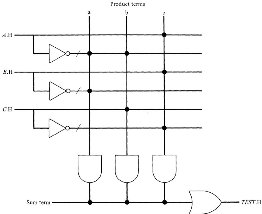
**Figure 4-23.** A PLA realization of  $TEST = \bar{A}\bar{B} + \bar{A}C + A\bar{B}\bar{C}$ .
