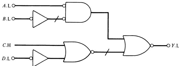
Figure 2-13. Implementation of  $Y = A \cdot \overline{B} + (\overline{C} + \overline{D})$ .
