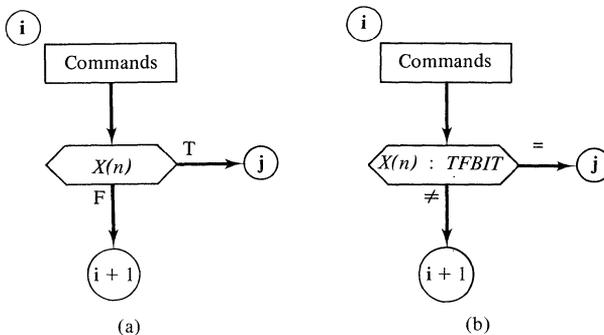
**Figure 10-7** ASMs for single-qualifier, single-jump address microinstructions. (a) Microinstruction branches on a true qualifier. (b) Microinstruction allows selection of the jump condition.
