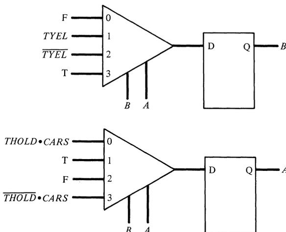
**Figure 6-18** A multiplexer state generator for the traffic-light controller.
