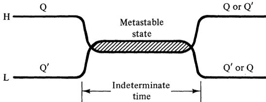
**Figure 12–19.** Metastability in the 7474 D flip-flop. The final stable state is unpredictable, but  $Q$  and  $Q'$  are inverses.
