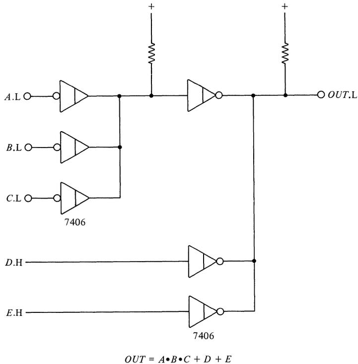
Figure 2-27. A logic realization with open-collector gates.
