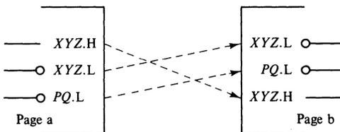
**Figure 2-4.** Illustrating the need for a convention for naming signals.
