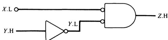
We inserted a voltage inverter to change signal  $Y.H$  into  $Y.L$ , the input required for our AND gate. You will find that adding voltage inverters where necessary requires no active thought; the little mixed-logic voltage-polarity circles direct you to do the right thing.
