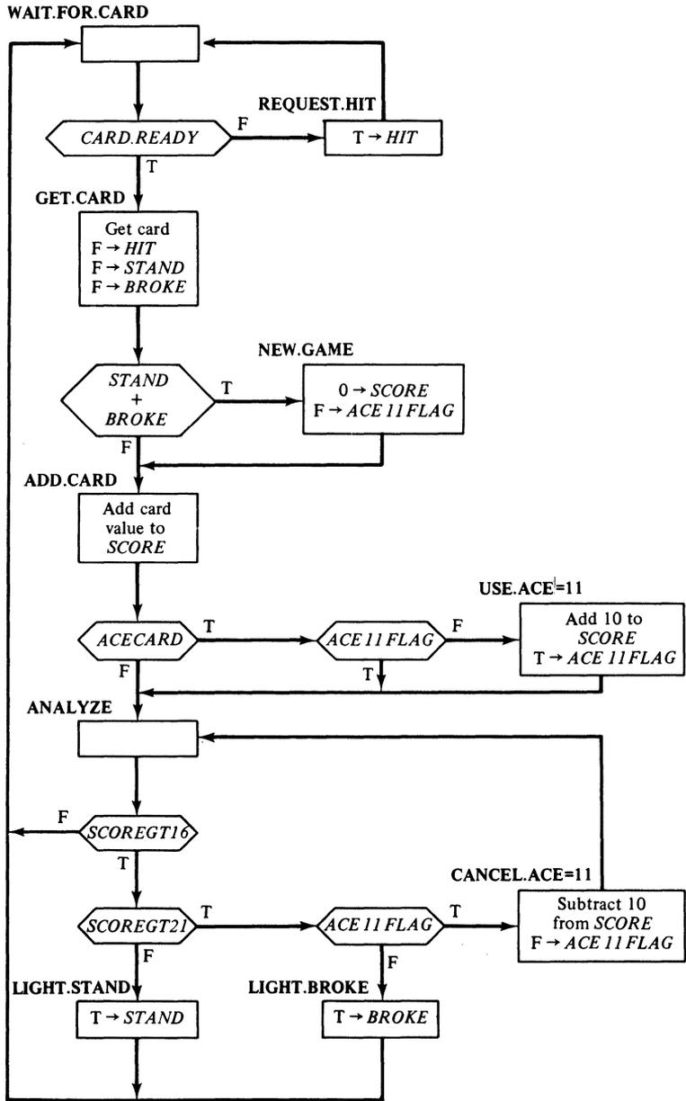
Figure 6-26 A primitive ASM for a Black Jack Dealer, with too many states and an error.
