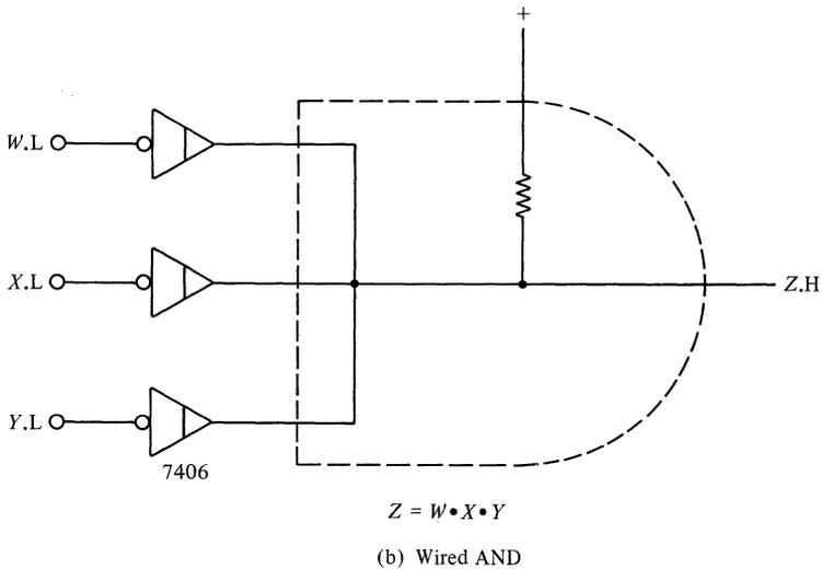
**Figure 2–26.** Wired logic with a 7406 open-collector inverter.
