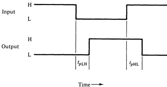
**Figure 4-1.** Timing diagram showing propagation delays in a logic circuit.
