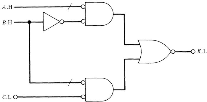
Figure 2-24. A mixed-logic circuit for  $K = \bar{A} \cdot B + \bar{B} \cdot C$ .
