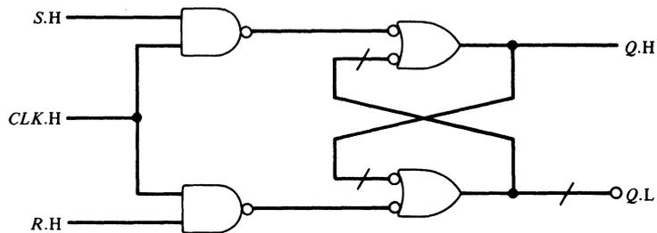
Figure 4-9. A clocked RS flip-flop circuit.
