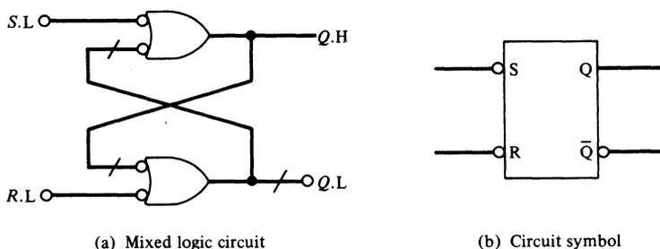
Figure 4-7. An asynchronous RS flip-flop constructed with Nand gates.
