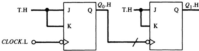
**Figure 4-14.** A binary ripple counter. The least significant bit is on the left. This circuit displays both logic and voltage, whereas the related Fig. 4-13 displays only logic.
