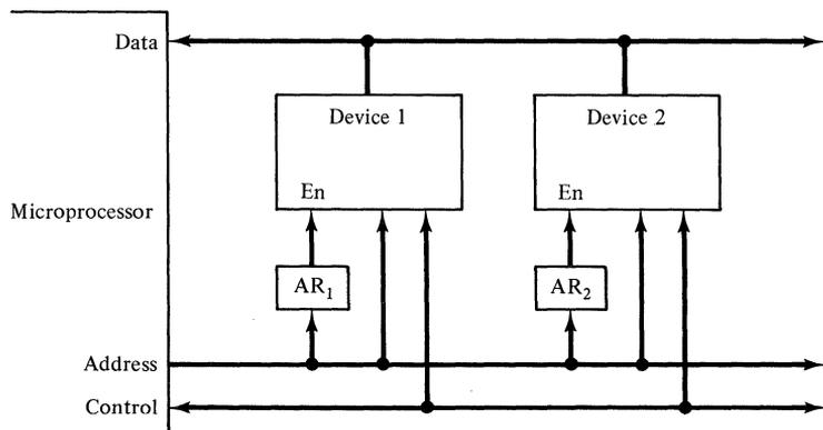
**Figure 11-1.** The bus structure of a microcomputer. Each device has an address recognizer *AR*.
