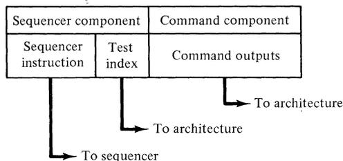
The sequencing component of the microinstruction becomes an instruction to be processed by a *microprogram sequencer*, contained within the microprogram control unit. The sequencer and its instruction input may be relatively simple,
