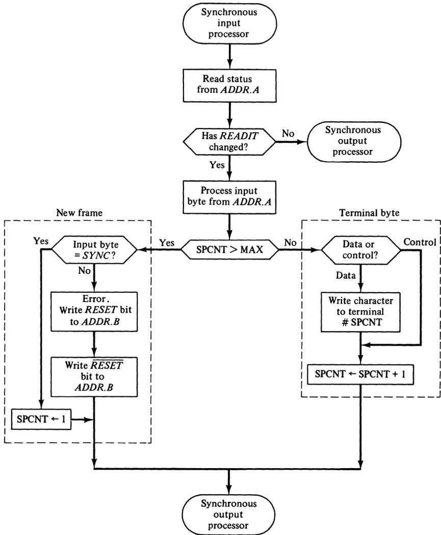
Figure 11-16. Algorithm for the terminal multiplexer: synchronous input (S → P) processing.
