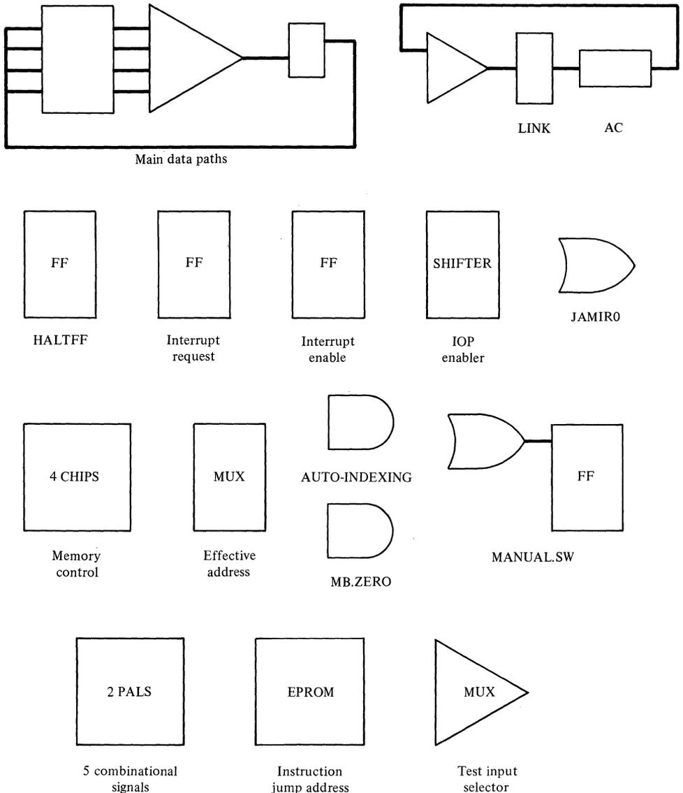
Figure 10-23 Hardware elements in the LD30.
