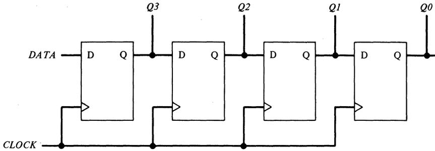
Figure 4-19. A simple shift register constructed with D flip-flops.
