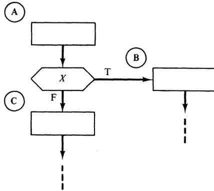
**Figure 5-6.** An ASM with a conditional branch.
