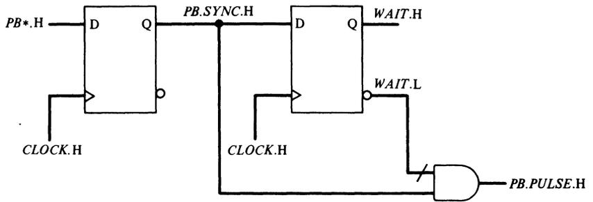
Figure 6-2 A single-pulser circuit.
