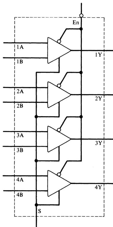
Figure 3-7. The 74LS157 Quad Two-Input Multiplexer.
