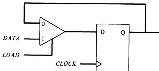
Figure 4–12. An enabled D flip-flop.
