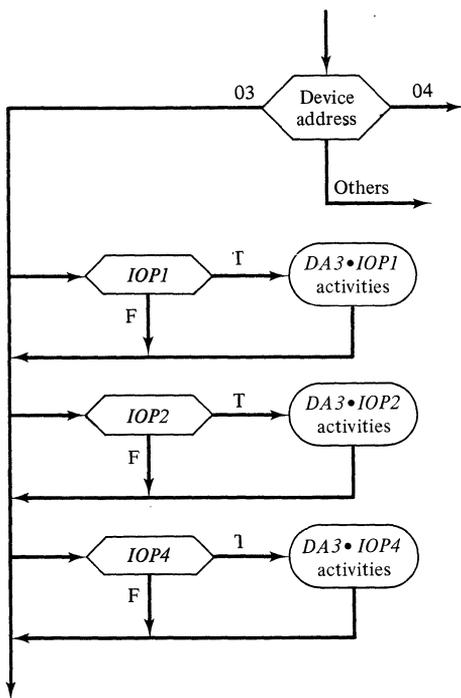
Figure 9-3 An asynchronous ASM for *IOP* signals.
