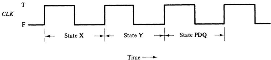
A sequence is an inherent property of an ASM chart; state Y follows state X, and so on. It is cumbersome to show time relations with a timing diagram such as the above; therefore, you should learn to think of time as rigorously implied in the ASM chart notation.
