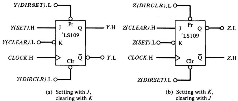
Figure 4–11. Two mixed-logic uses of the 74LS109 Dual JK Flip-Flop.
