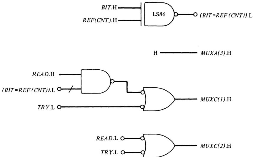
Figure 6-24 Some control mux inputs for an elegant combination lock.
