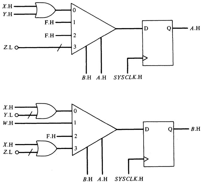
**Figure 5-14.** A multiplexer control for the ASM in Fig. 5-13.
