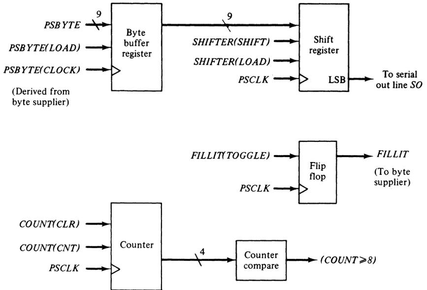
Figure 6-12 The logical structure of a parallel-to-serial converter.
