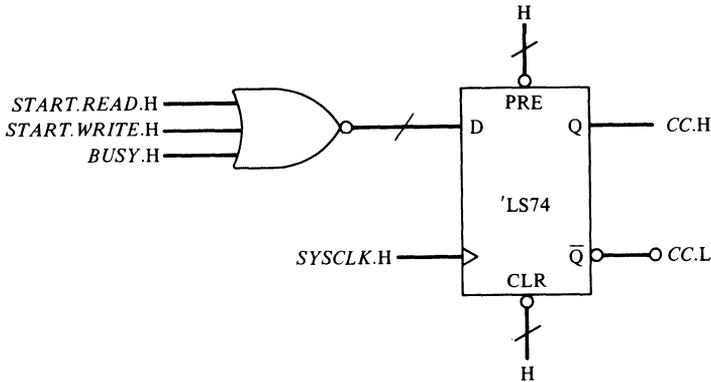
Figure 8-9 Extension of the standard memory interface of the LD20.
