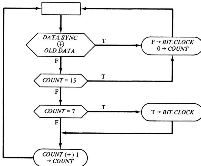
Figure 6-8 An ASM for a serial bit clock.
