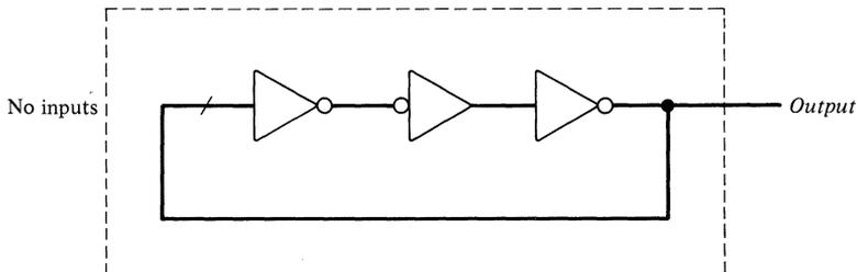
The voltage at the output is fed back into the input where, after a short time, it appears inverted on the output. The new voltage causes a similar inversion; the output voltage *oscillates* rapidly.
