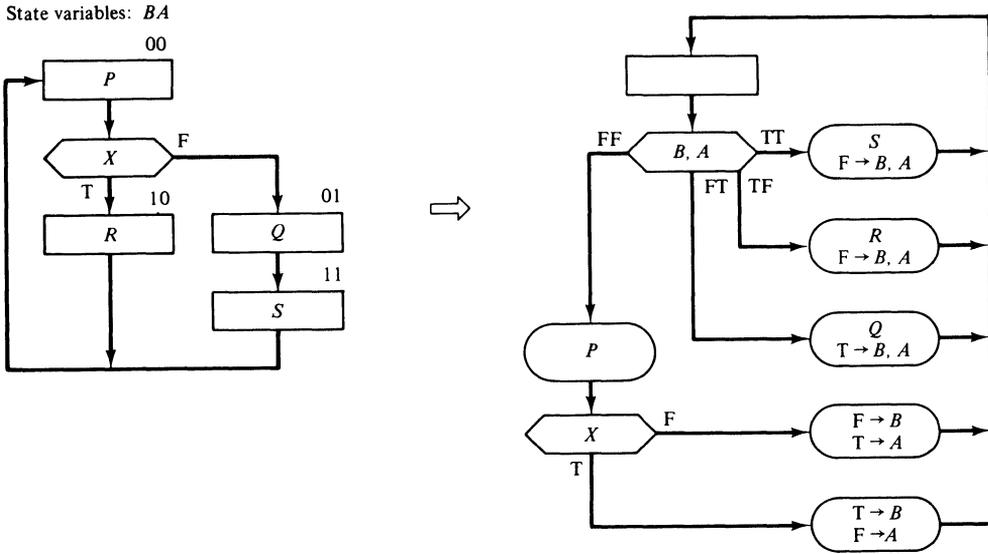
Figure 6-27 Converting a four-state ASM into a one-state ASM.
