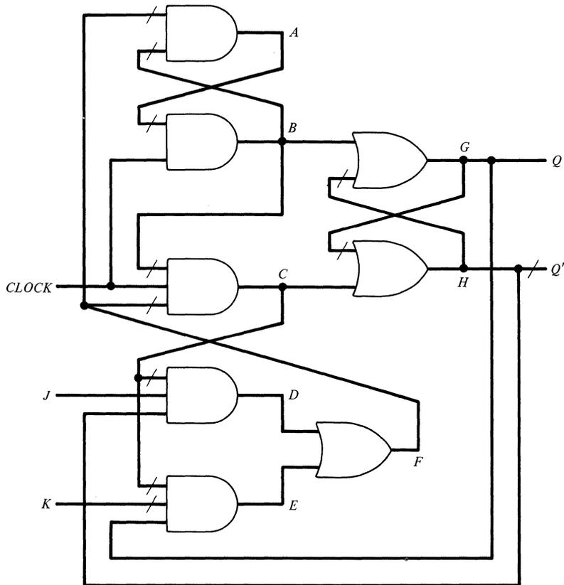
Figure 4-31. A 74LS109 JK flip-flop without an asynchronous set and clear.
