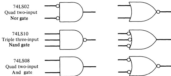
**Figure 2–5.** Mixed-logic symbols for some TTL gates.
