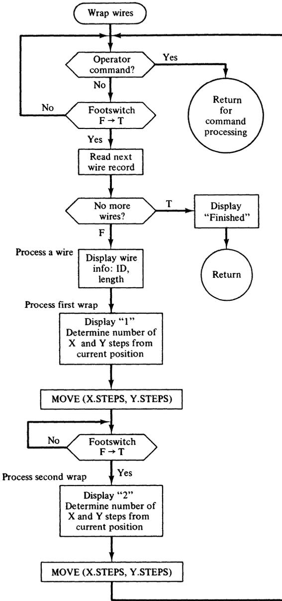
Figure 11-7. A software algorithm for wrapping wires in the wire list.
