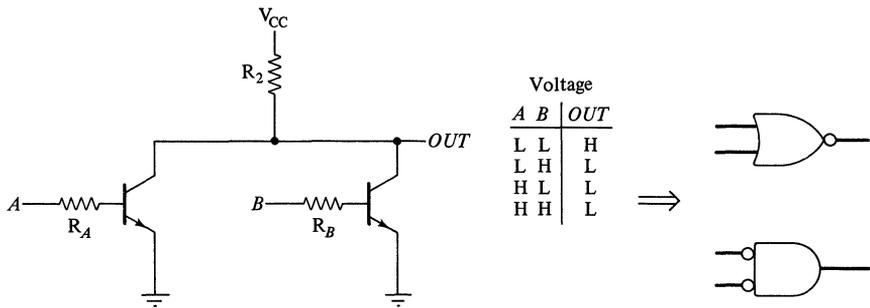
Figure 12-2. A 2-input gate made from two transistors.
