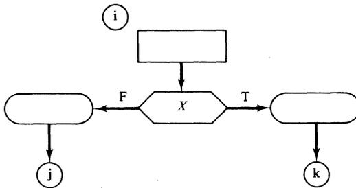
Figure 10-1 The ASM state executed by Wilkes's microprogramming machine.
