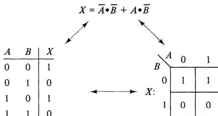
**Figure 1-4.** Three representations of a Boolean function.
