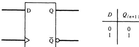
As an SSI device, the D flip-flop appears in these common varieties:
