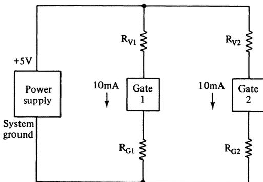
**Figure 12–15.** Two gates powered by one supply, with resistance in the power-distribution system. Line resistances are lumped for convenience. Logic inputs and outputs are omitted.
