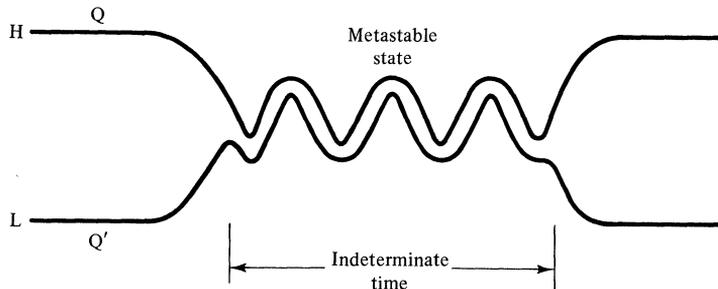
**Figure 12–20.** Metastability in cross-coupled 7400 Nand gates. When set or cleared with a runt pulse, the outputs may oscillate in phase.
