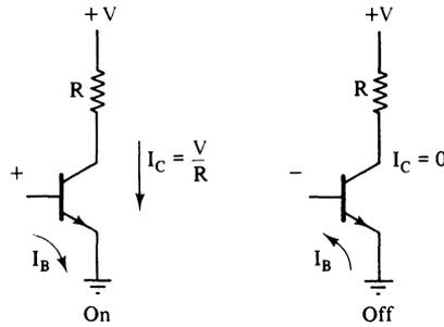
The transistor acts as an amplifier of current, in that a small base current can control a much larger current in the emitter-collector path. The term  $\Delta I_C / \Delta I_B$  defines the *gain* of the transistor; in common switching transistors, the gain is from 20 to 100.
