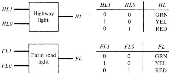
**Figure 6–19** A particular traffic light for Design Example 5.
