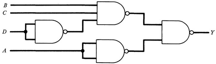
**Figure 2-20.** Positive-logic implementation of  $Y = A + B \cdot C \cdot \bar{D}$ , using Nand-gate rules.
