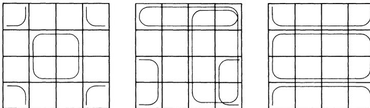
Figure 1-10. Typical circlings of four 1's and eight 1's on K-maps of four variables.
