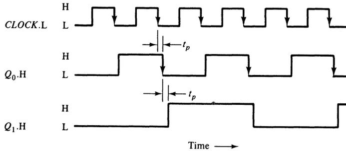
**Figure 4-15.** A timing diagram for a 2-bit ripple counter. Each stage suffers a cumulative propagation delay. In synchronous counters there is only one delay.
