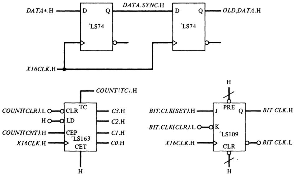
Figure 6-9 The architecture of a serial bit clock.
