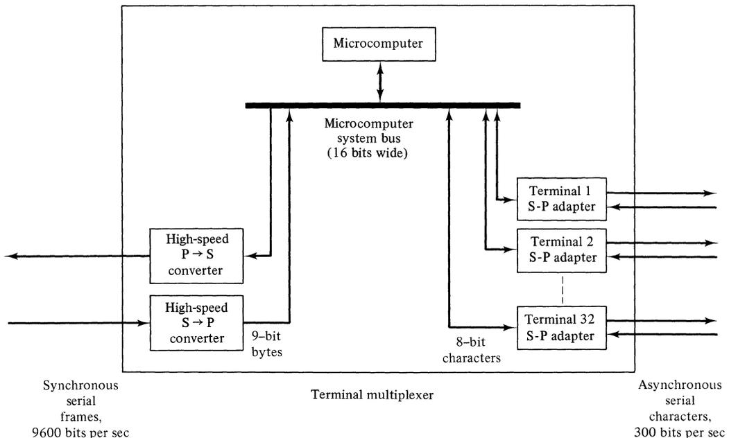
**Figure 11–13.** Components and data flow in the terminal multiplexer.
