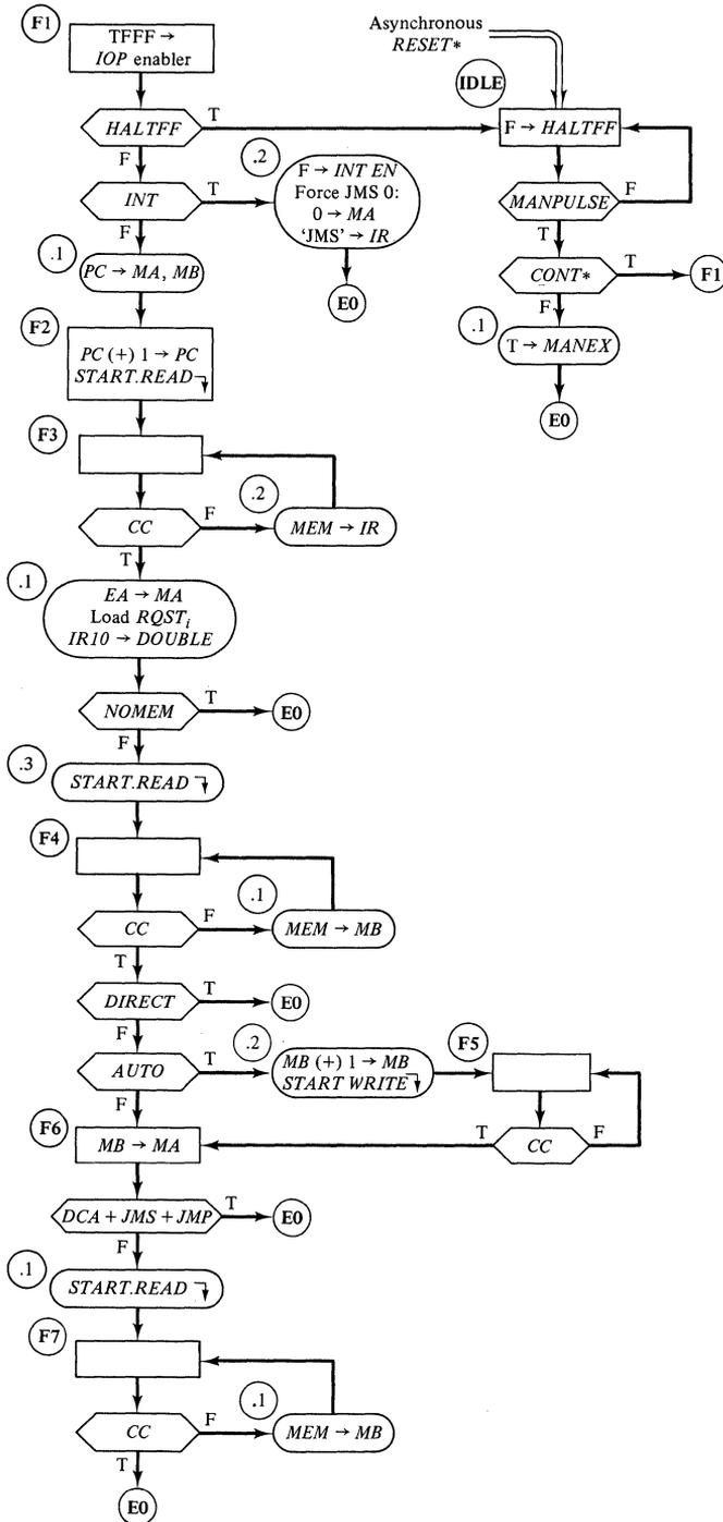
Figure 7-42 ASM of the LD20's fetch phase.
