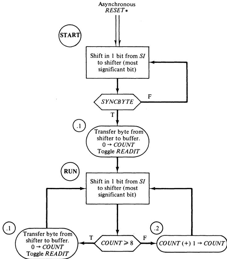
Figure 6-13 An ASM for serial-to-parallel conversion.
