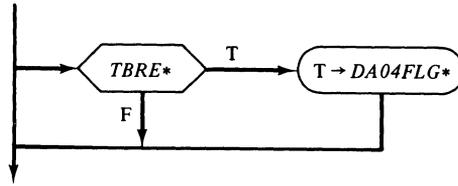
This implies a D flip-flop to hold *DA04FLG\**, as proposed earlier. The flip-flop will have *T* as its input and *DA04FLG\** as its output. The *F → T* transition of *TBRE\** will act as an active clock edge, which will transfer the true input into the flip-flop, where it will remain until an *IOP2* command clears the flag. After clearing, only a subsequent *F → T* transition of *TBRE\** will clock truth into *DA04FLG\** again.
