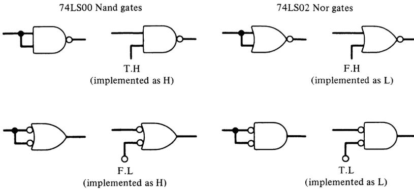
Figure 2-12. Nand and Nor gates used as voltage inverters.
