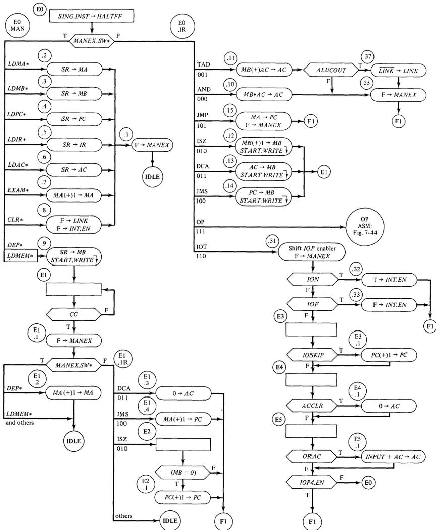
Figure 7-43 ASM of the LD20's execute phase, excluding the Operate instruction.
