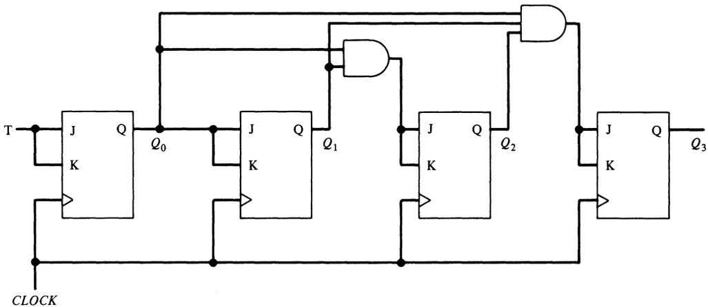
Figure 4-17. A 4-bit (modulo-16) synchronous counter.
