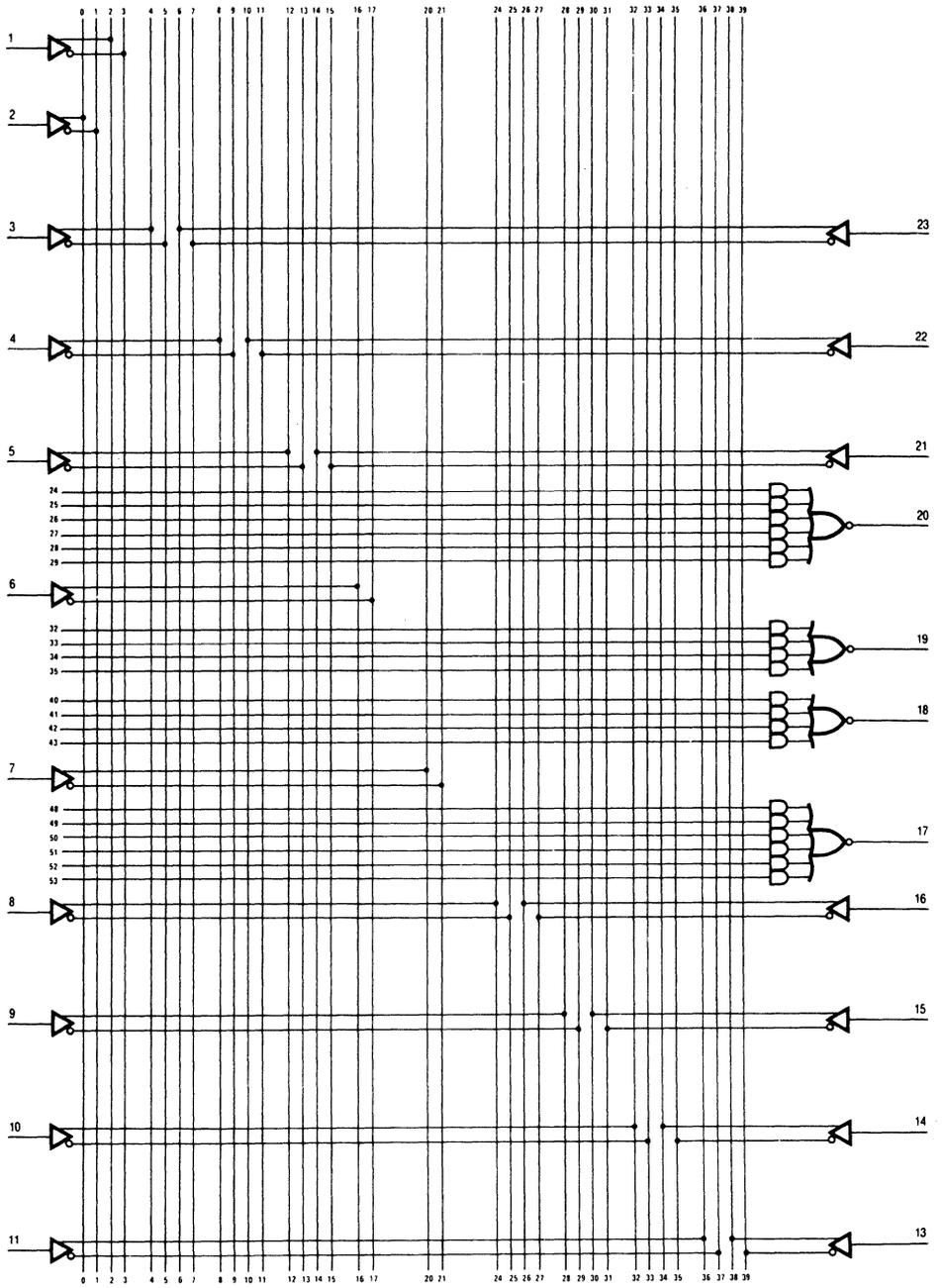
Figure 4-25. A PAL18L4. (Courtesy of Monolithic Memories, Inc.)
