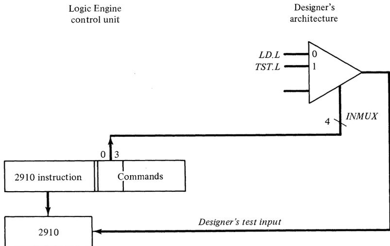
Figure 10-16 Structure of the test input in a microprogrammed design.
