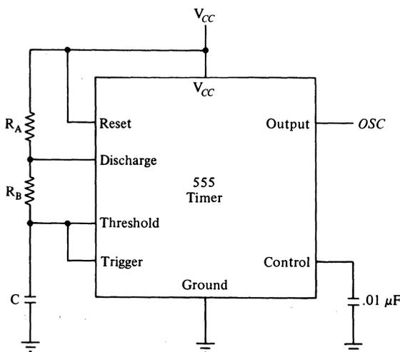
**Figure 12–11.** The 555 timer used as an oscillator.  $R_A$ ,  $R_B$ , and  $C$  control the frequency.
