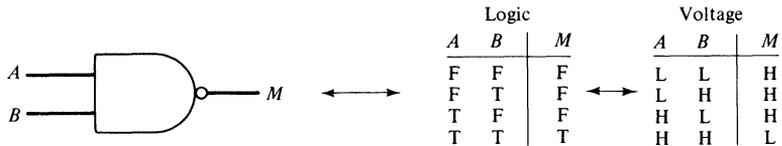
Here, the symbol completely defines the behavior of both the logic and the voltage. Can we find a physical device with this voltage table? If so, we can use this mixed-logic symbol to perform AND with a real device. A look at the first chip in a TTL data book shows that the 74LS00 Quad Two-Input Nand Gate behaves this way. Now we have a symbol that describes both a logic operation and a piece of hardware.
