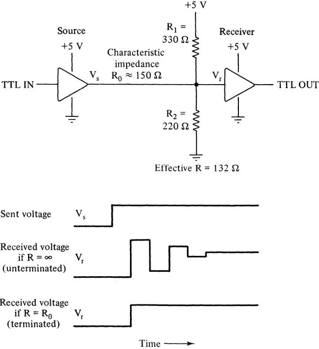
**Figure 12-17.** Signal transmissions on a long line. The unterminated line has reflections; proper termination solves the problem.
