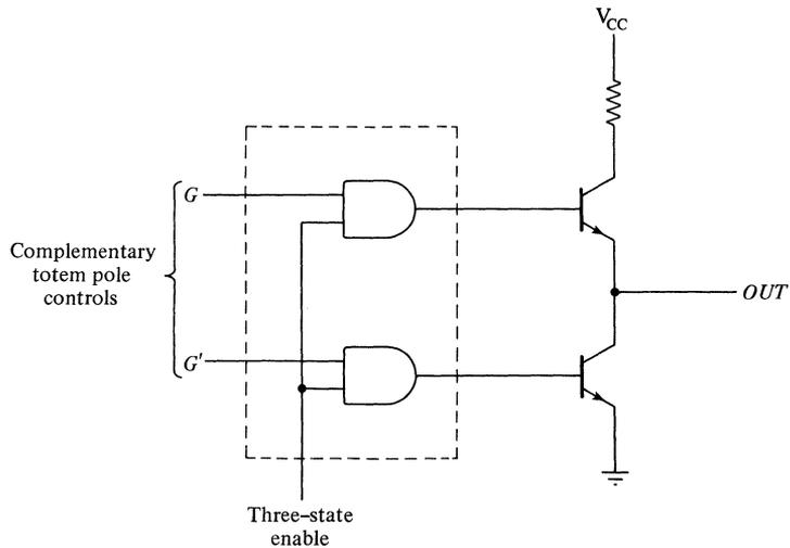
Figure 12-6. A model of TTL three-state output control.
