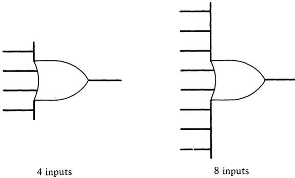
**Figure 2-2.** Symbols for OR with multiple inputs.
