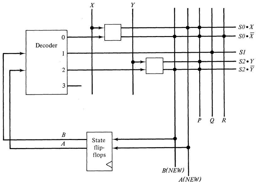
Figure 10-3 A diode-based microprogrammed implementation of Fig. 10-2.
