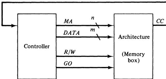
**Figure 5–2.** A diagram of a memory-write machine.
