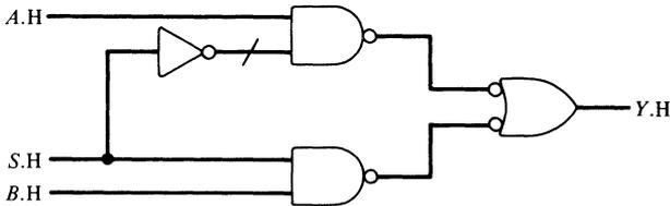
Figure 3-3. Implementation of the electronic switch  $Y = A \cdot \bar{S} + B \cdot S$ .
