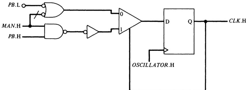
Figure 6–6 A circuit for a system clock.
