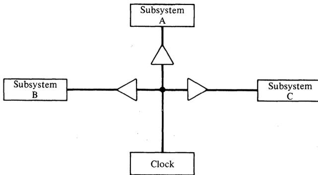
**Figure 5-18.** A buffered radial distribution system for the master clock.
