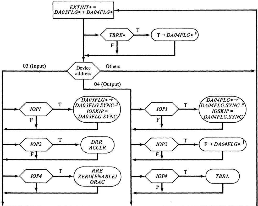
Figure 9-5 ASM chart of the interface between an LD20 and a terminal.
