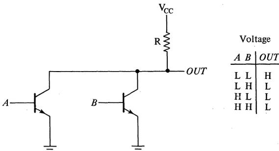
Figure 12-5. An open-collector wired OR.
