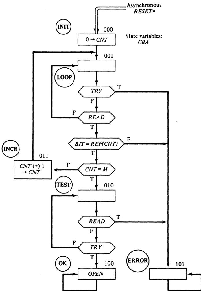
Figure 6-21 An ASM for an elegant combination lock.
