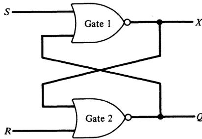
**Figure 4-6.** An asynchronous RS flip-flop constructed with Nor gates.
