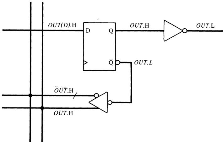
For emphasis, the diagram shows each signal and its polarity. If a  $T = H$  output is required, one useful technique is to produce the *inverse* of the required flip-flop input. Develop a standard mixed-logic diagram for an output stage of this PAL that produces an output having  $T = H$ .
