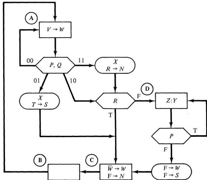
Figure 5-22. A "loaded" ASM for practice in implementing.
