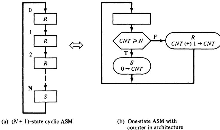
Figure 6-28 Equivalent formulations of a cyclic process of  $N + 1$  elements.
