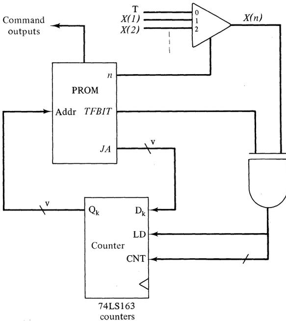
Figure 10-8 A counter-based implementation of the microinstruction control in Fig. 10-7b.
