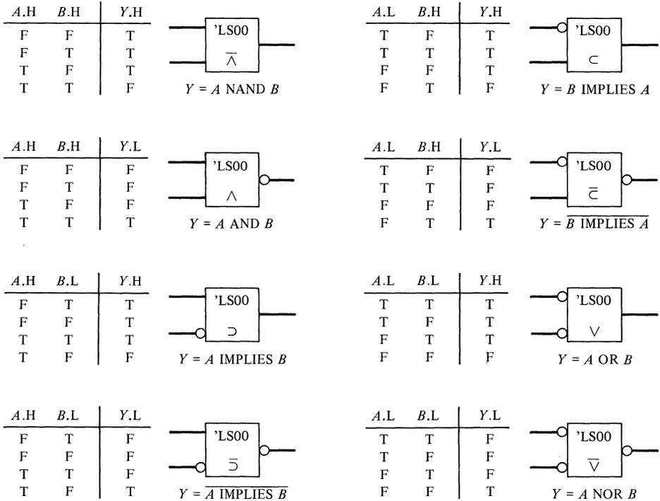
Figure 2-28. What logic does the 74LS00 Nand Gate perform?
