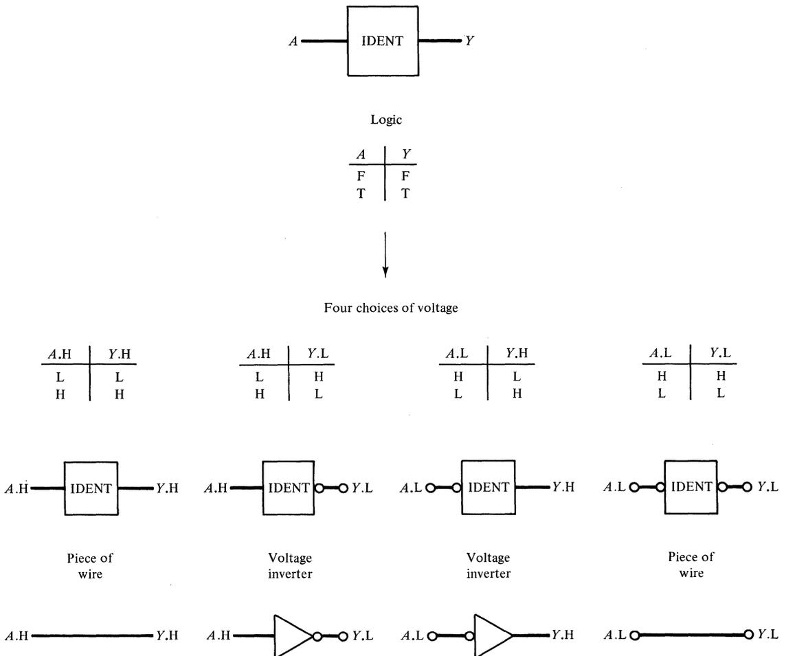
Figure 2-8. Realizations of the logical identity operation.
