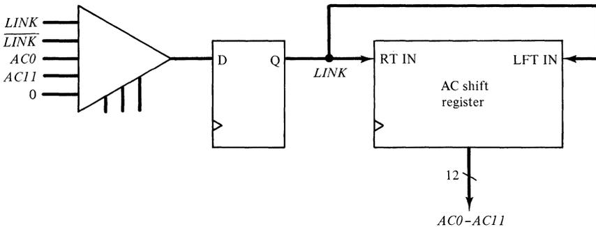
Figure 10-19 The accumulator and link of the LD30.
