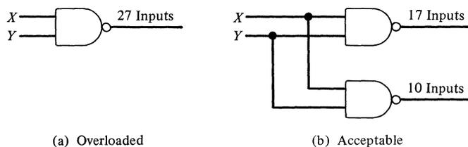
Another technique is to use a high-power amplifier called a *buffer* to drive the entire set of inputs. For instance, in a 74LS37 Quad Two-Input Nand Buffer  $I_{OH} = 1.2\text{ mA}$  and  $I_{OL} = 24\text{ mA}$ , three times the values of the standard 74LS gate output.
