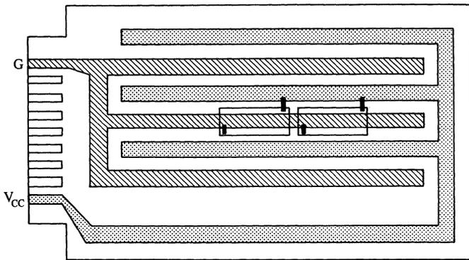
**Figure 12–16.** A circuit board with strip power busses. Two integrated-circuit chips are attached.
