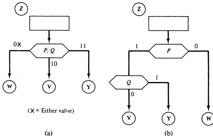
**Figure 5-7.** Alternative representations of a three-way branch.
