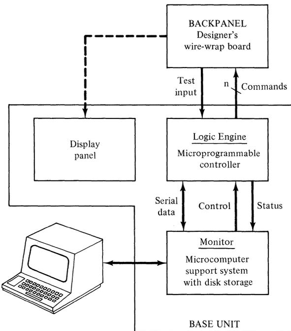
Figure 10-13 The Logic Engine.
