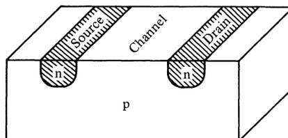
The p-type region between the n-type diffusions is called the *channel*. This arrangement appears similar to the bipolar npn transistor, except that the channel is several microns wide—much wider than the base region in a bipolar transistor.
