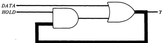
**Figure 4-4.** A latch circuit; the heavy line is the feedback path.
