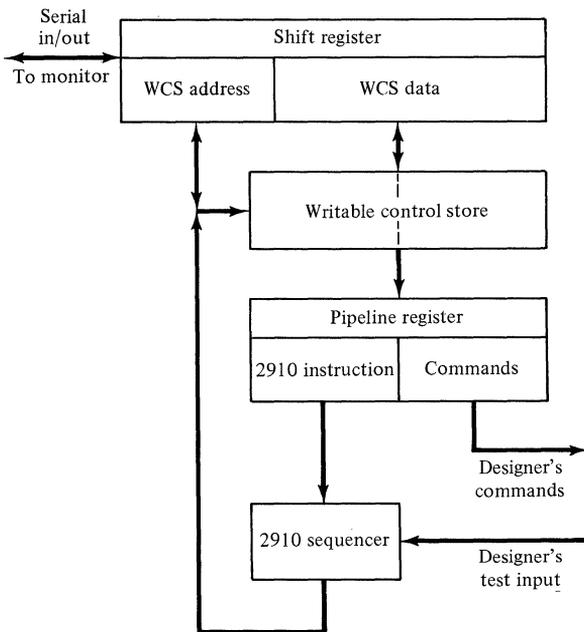
**Figure 10-14** The architecture of the Logic Engine controller.
