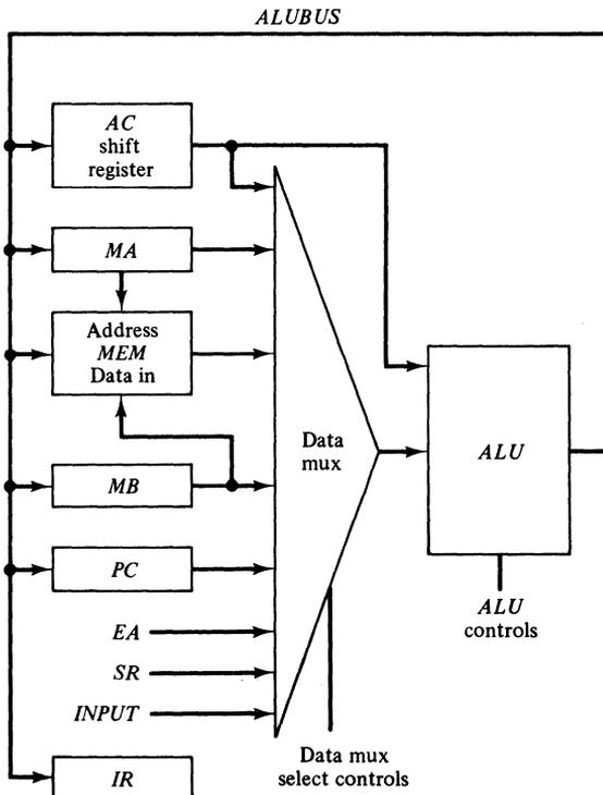
Figure 7-41 Architecture of the LD20: main data paths; one of twelve 1-bit slices.
