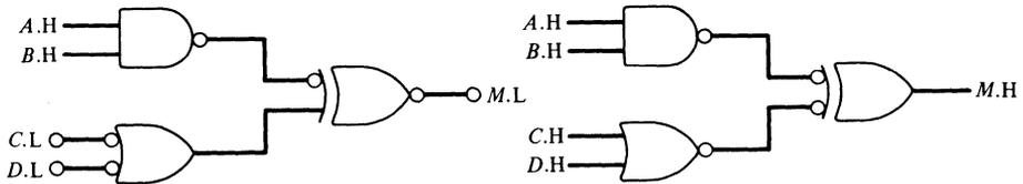
Figure 2–25. Mixed-logic circuits for  $M = (A \cdot B) \oplus (C + D)$ .
