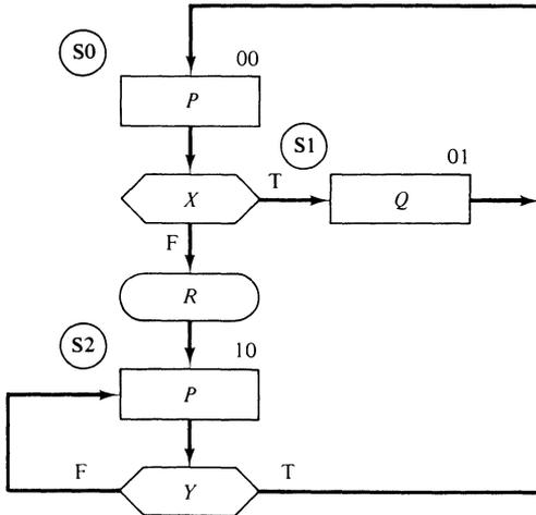
**Figure 10-2** An ASM with three states, to illustrate classical microprogrammed control.
