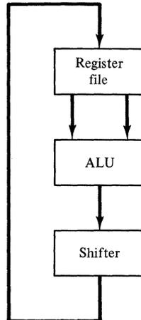
**Figure 4-21.** The architecture of a typical processor.
