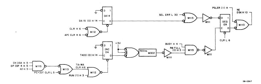
Figure 4-32 NonExistent Disk by Sequence Error
