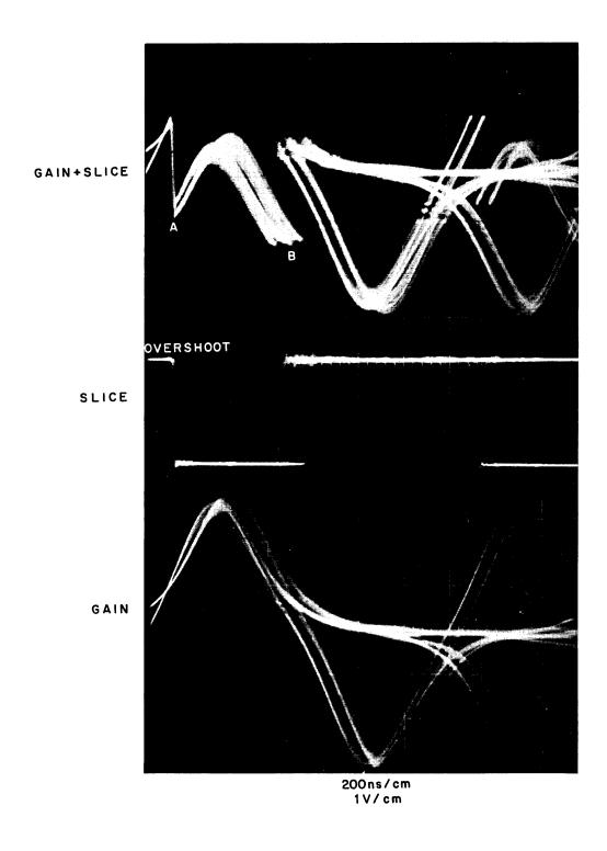
Figure 6-4 Measuring the Slice of the B Track
