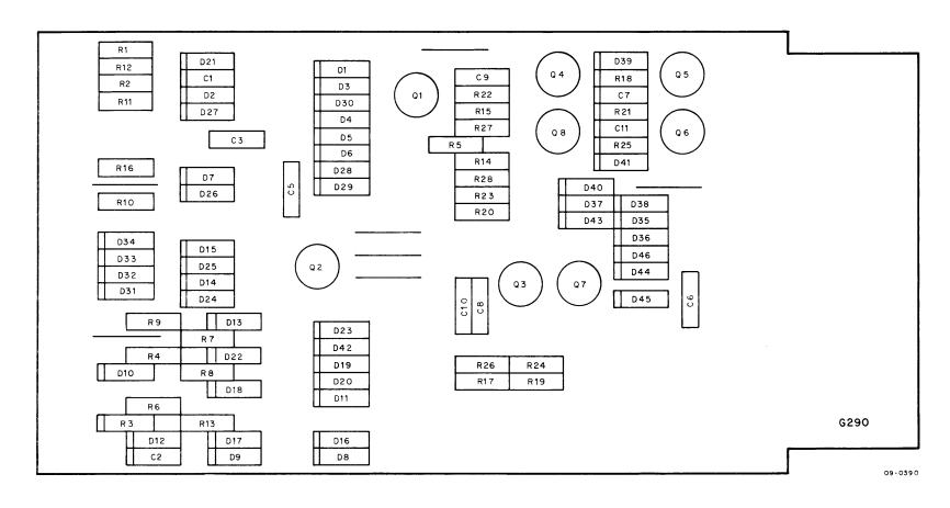
Figure 2-14 G290 Writer Flip-Flop, Parts Location Diagram
