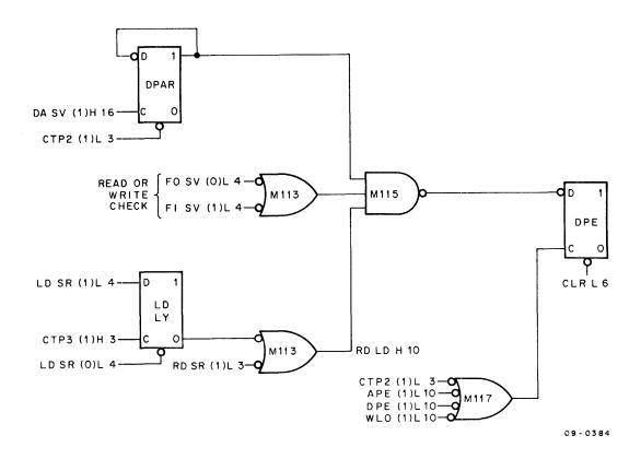
Figure 4-29 Data Parity Error
