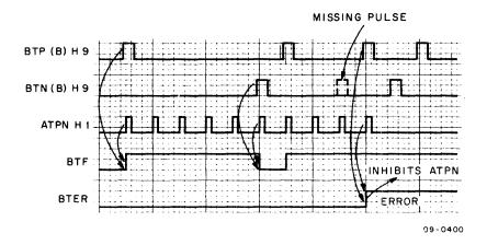
Figure 4-4 B Track Timing Diagram
