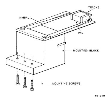
Figure 7-7 Aligning the Heads
