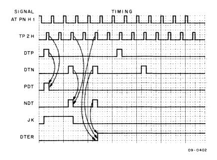
Figure 4-6 Data Track Timing Diagram
