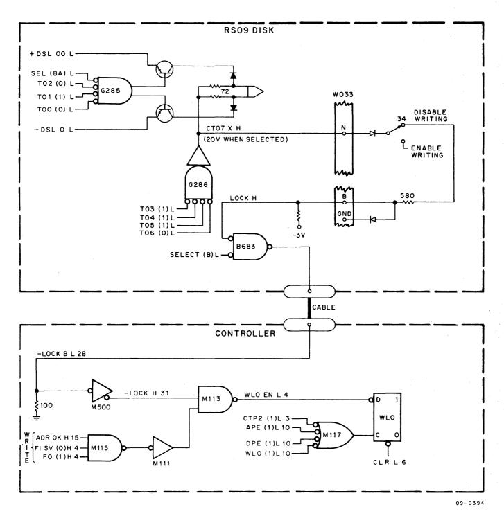
Figure 4-30 Write LockOut Error
