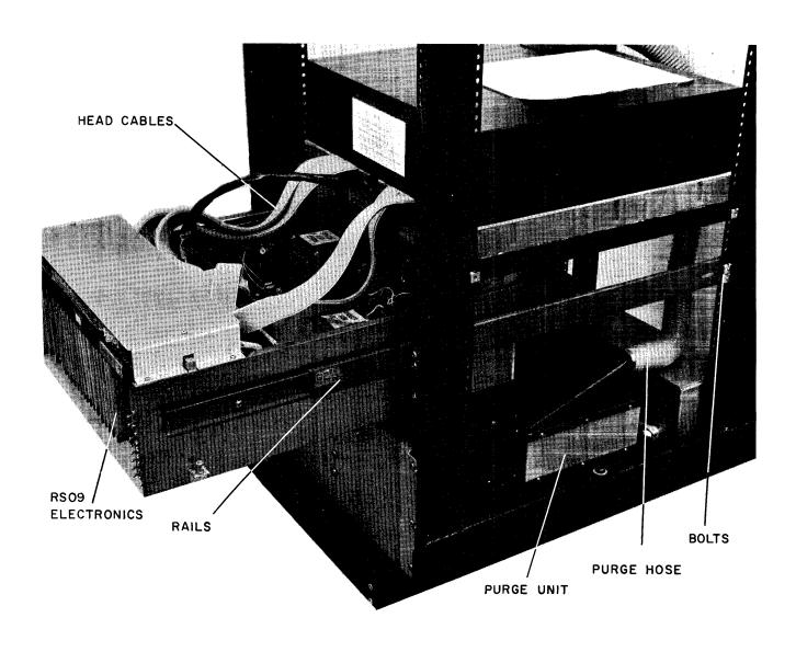
Figure 7-2 Removing the Disk Assembly from the Cabinet
