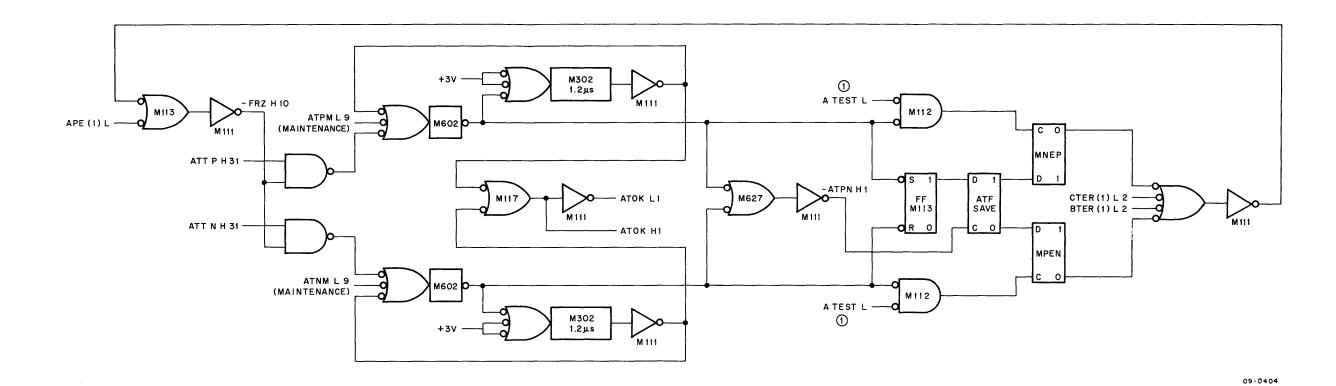
Figure 4-1 A Track Error Detection
