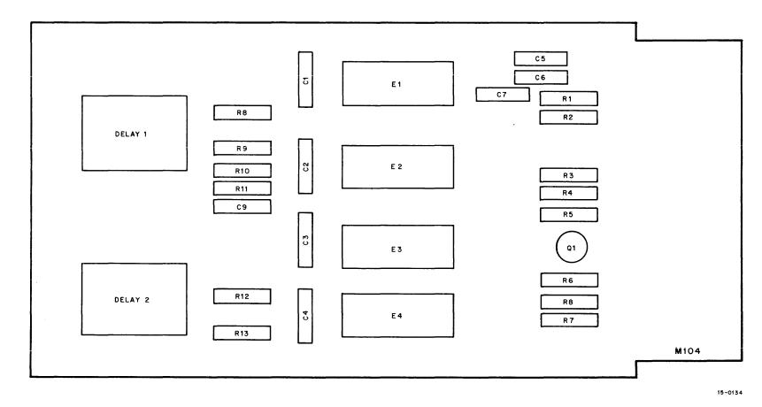
Figure 2-24 M104 Multiplexer, Parts Location Diagram
