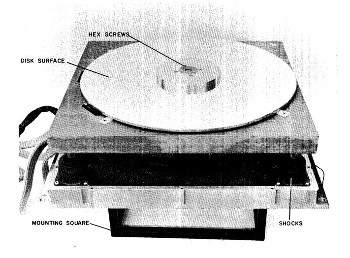
Figure 7-4 Disk Assembly With Cover Removed
