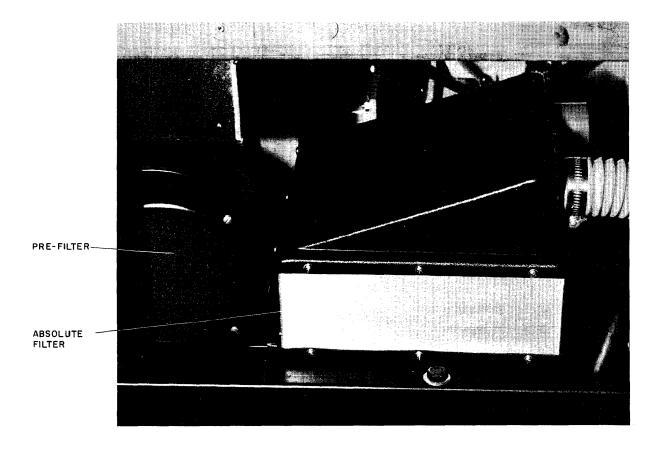
Figure 6-1 Purge Unit and Filters
