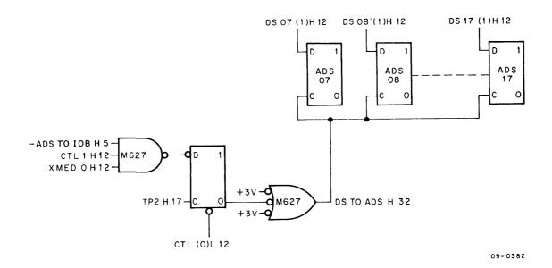
Figure 4-16 ADS Register Logic
