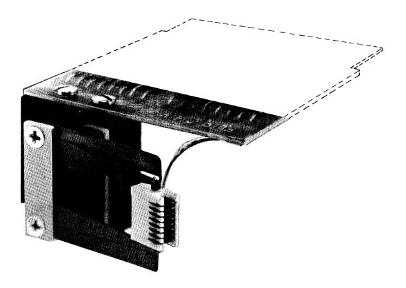
Figure 7-6 Shoe Assembly Removed
