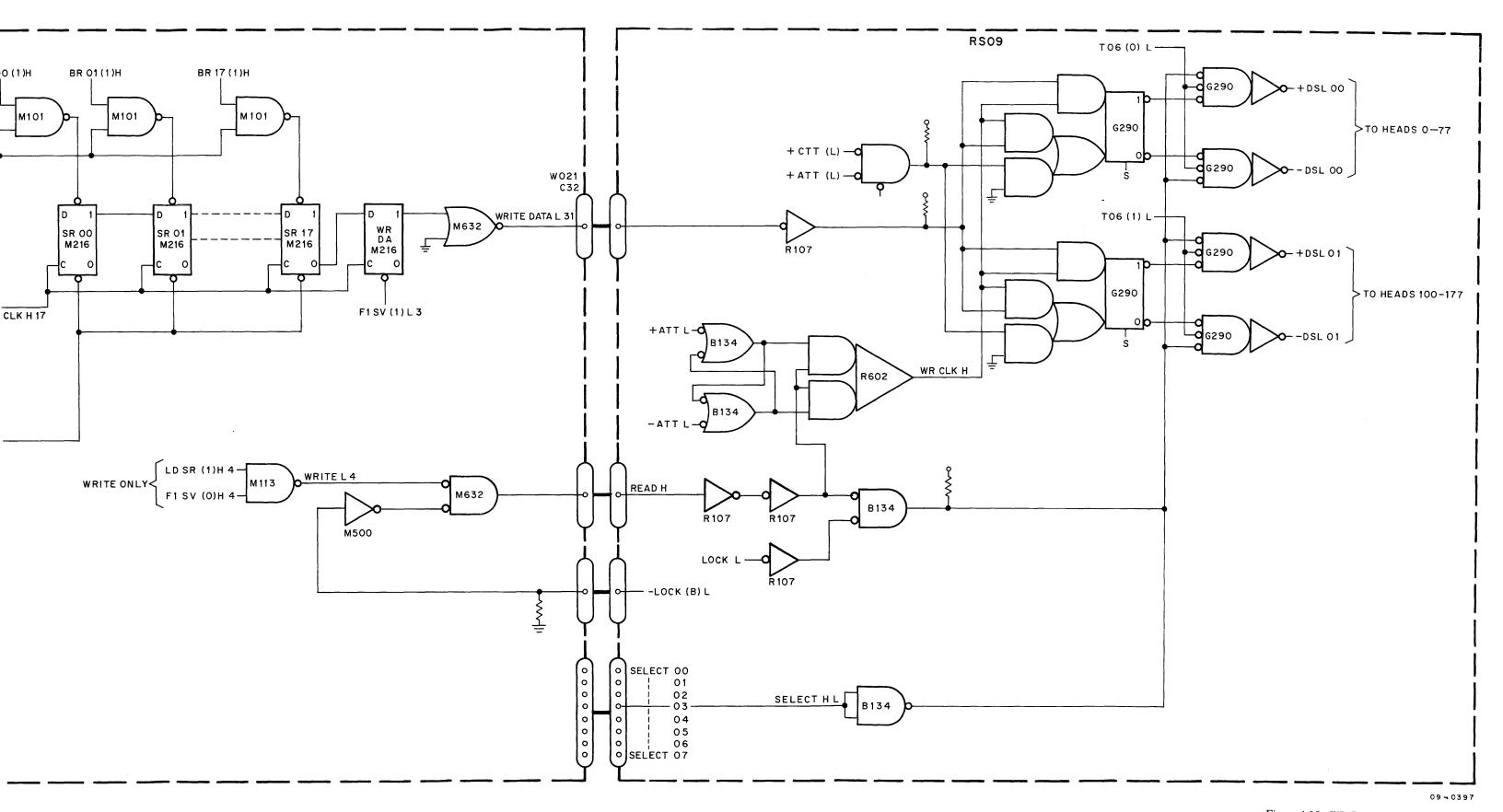
Figure 4-19 WRITE Circuitry
