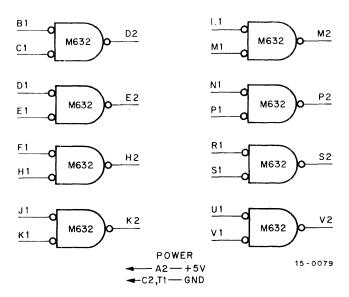
Figure 2-32 Negative Driver, Block Schematic
