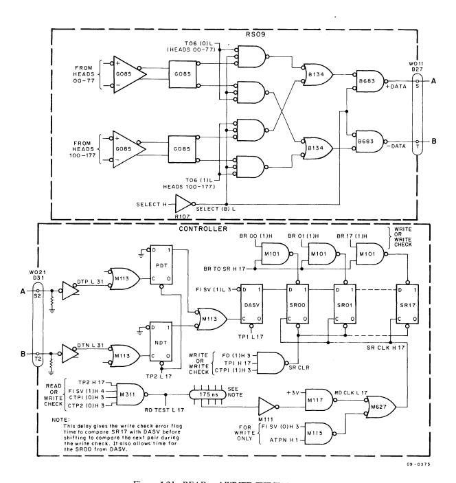
Figure 4-21 READ and WRITE CHECK Logic
