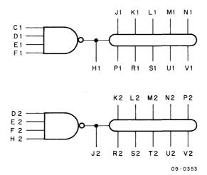
Figure 2-26 M311 Tapped Delay, Block Schematic
