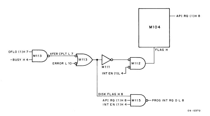
Figure 4-35 Automatic Priority Interrupt and Program Interrupt Logic
