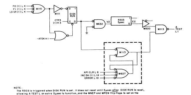
Figure 4-36 Disk Run Logic
