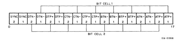
Figure 1-9 AC Bit Usage for IOT DGSS
