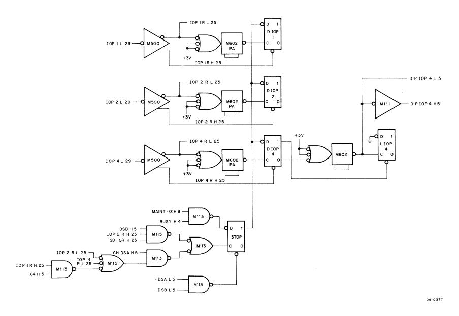
Figure 4-7 IOT TRAP Logic
