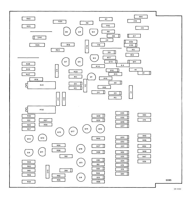
Figure 2-5 Disk Read Amplifier and Slice, Parts Location Diagram
