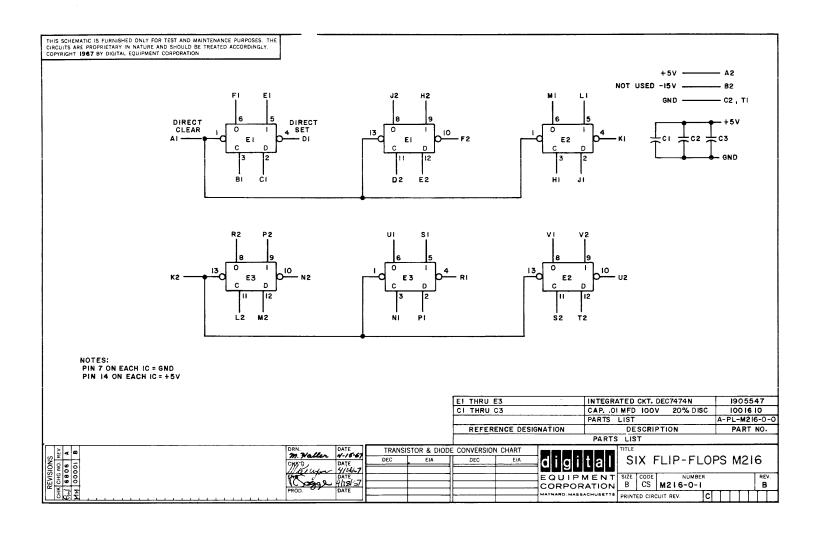
Figure 2-25 M216 Six Flip-Flops, Circuit Schematic
