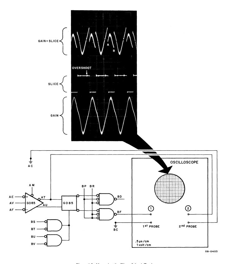
Figure 6-3 Measuring the Slice of the A Track
