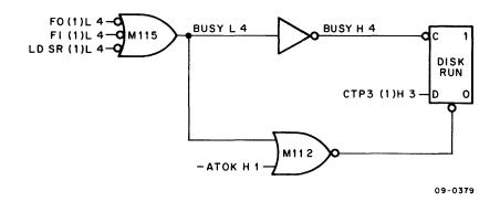
Figure 4-11 Unlock Sequence Logic
