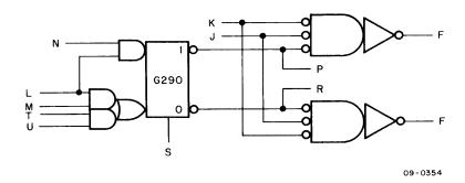
Figure 2-12 G290 Writer Flip-Flop, Block Schematic
