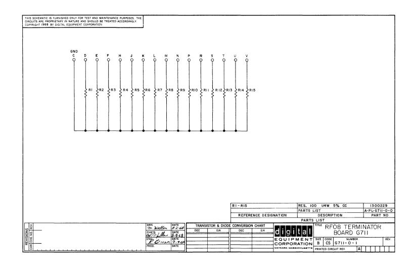
Figure 2-16 G711 RF08 Terminator Board, Circuit Schematic
