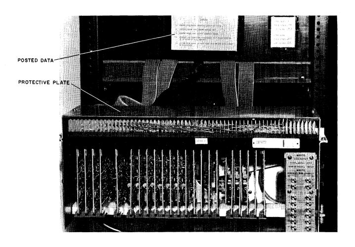
Figure 6-6 RS09 Electronics Showing Posted Data
