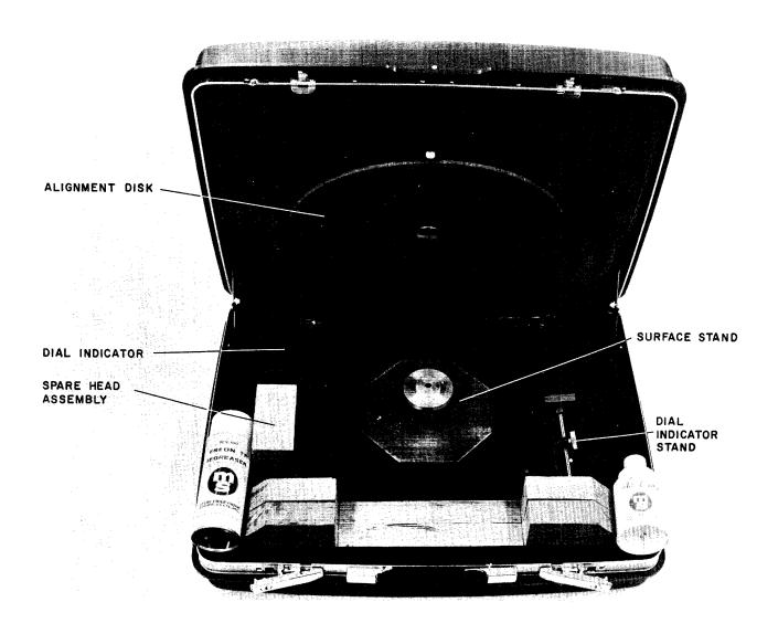
Figure 7-1 Disk Assembly Dismantling Kit
