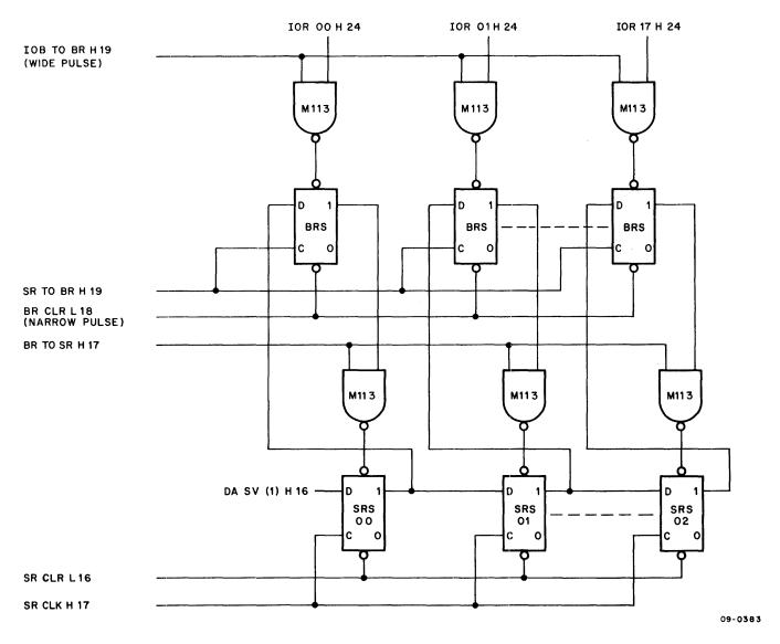
Figure 4-17 Buffer Register and Shift Register Interconnections
