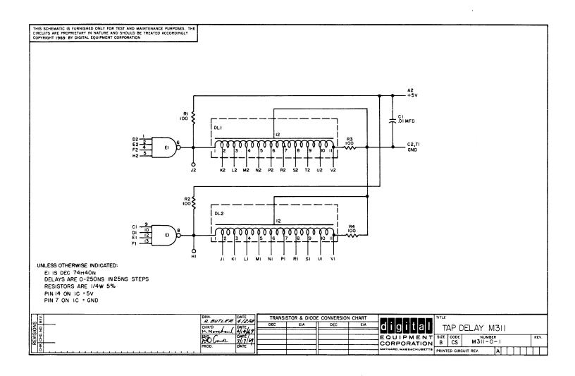
Figure 2-27 M311 Tapped Delay, Circuit Schematic
