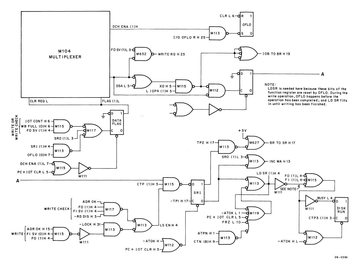
Figure 4-18 DCH Control for WRITE and WRITE CHECK
