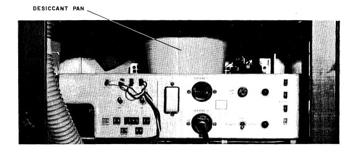
Figure 5-6 The Disk Assembly with Desiccant Pan
