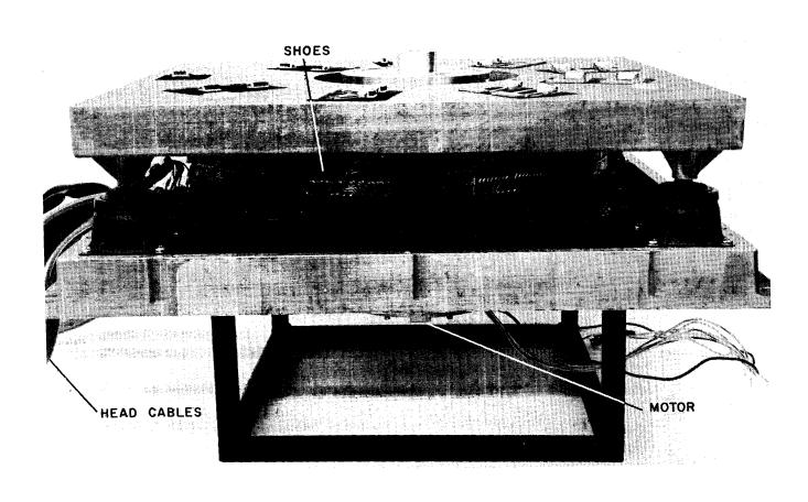
Figure 7-5 Disk Assembly With Cover and Surface Removed
