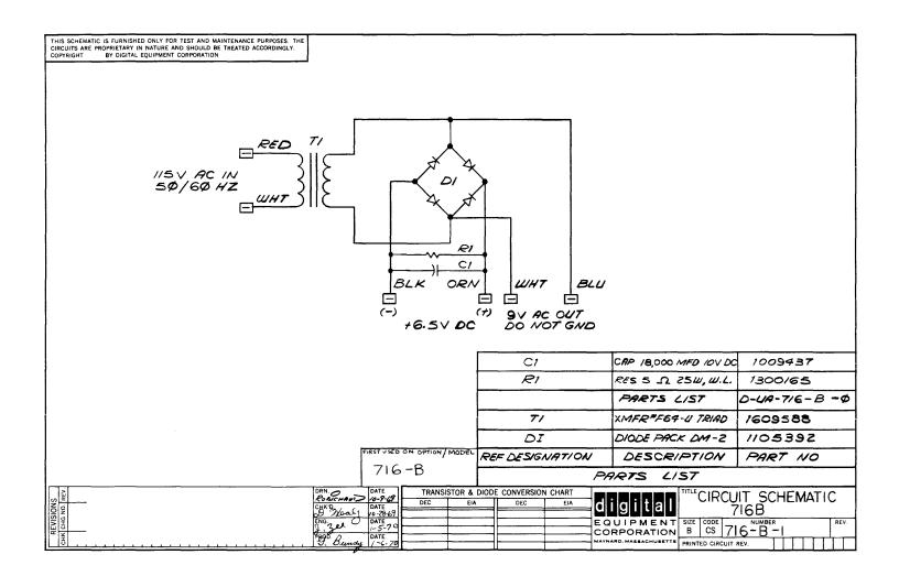
Figure 2-37 716 Indicator Supply, Circuit Schematic
