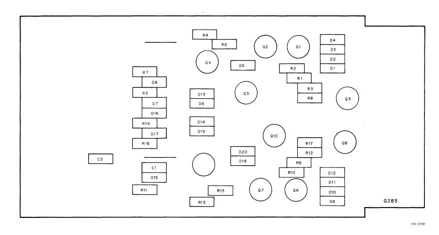
Figure 2-8 G285 Series Switch, Parts Location Diagram
