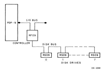
Figure 1-1 DECdisk System Configurations
