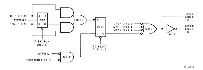
Figure 4-3 B Track Error Detection
