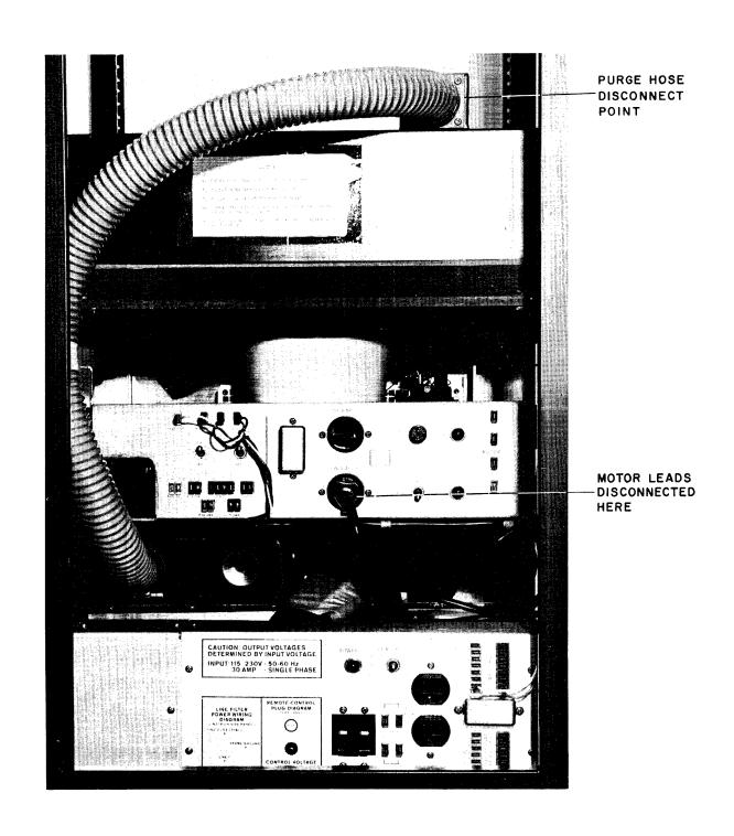
Figure 7-3 Disconnecting Motor Leads and Purge Hose
