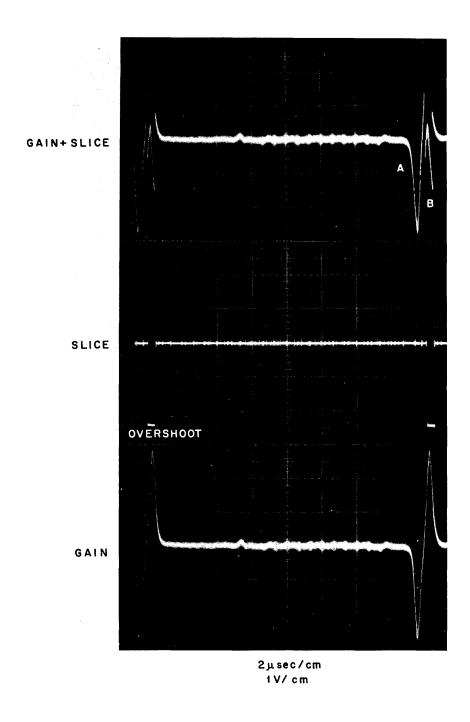
Figure 6-5 Measuring the Slice of the C Track
