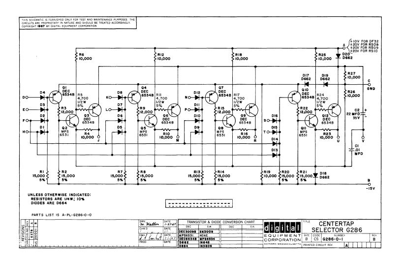
Figure 2-10 G286 Centertap Selector, Circuit Schematic
