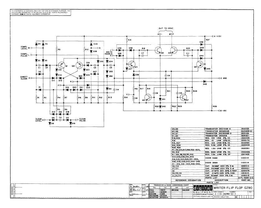
Figure 2-13 G290 Writer Flip-Flop, Circuit Schematic
