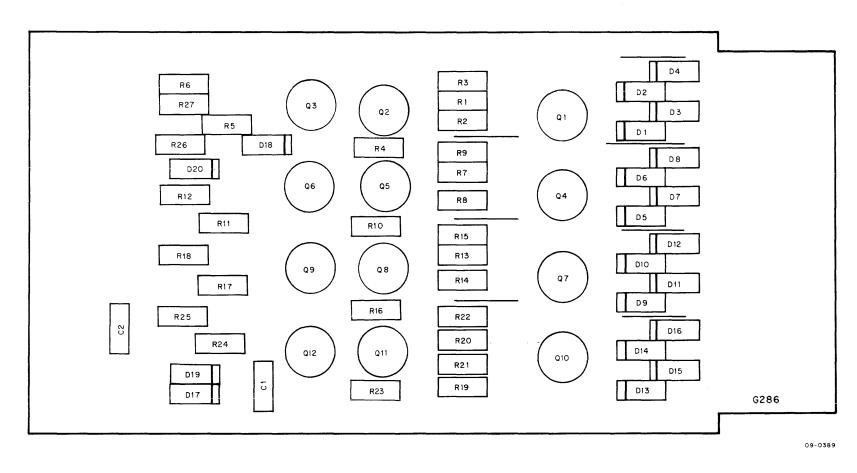
Figure 2-11 G286 Centertap Selector, Parts Location Diagram
