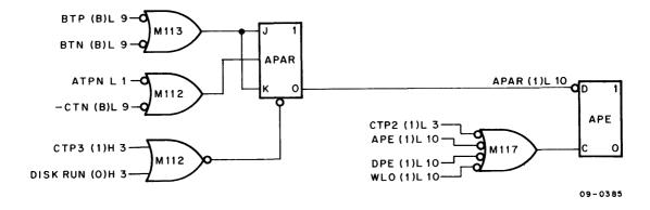
Figure 4-27 Address Parity Error
