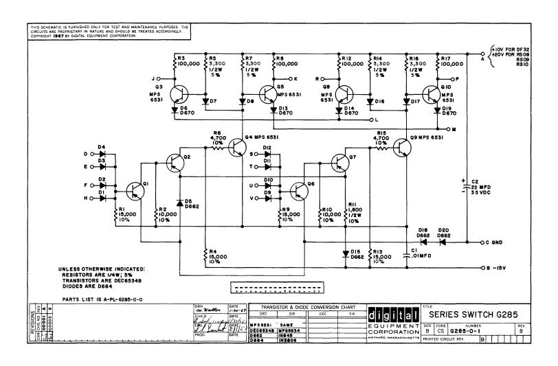
Figure 2-7 G285 Series Switch, Circuit Schematic
