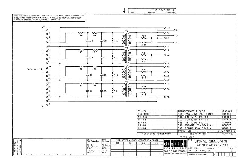
Figure 2-19 G790 Signal Simulator Generator, Circuit Schematic
