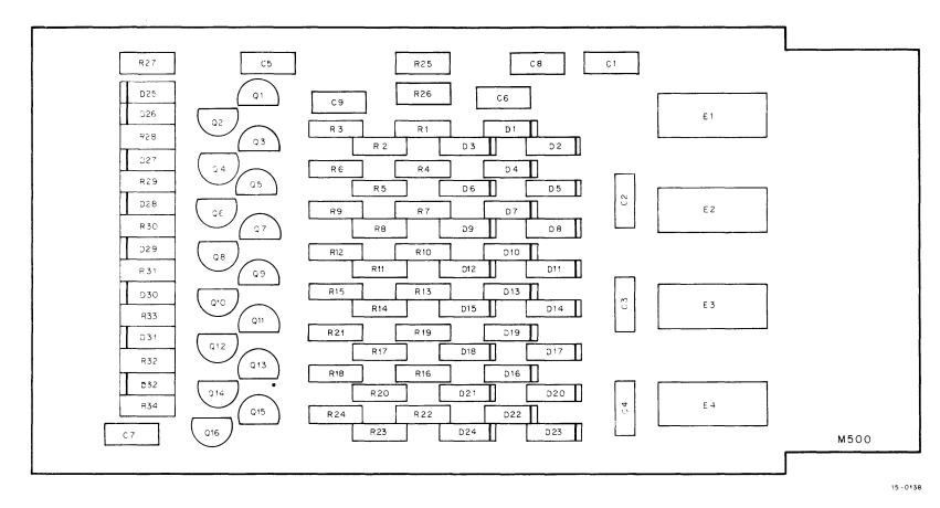
Figure 2-31 M500 Negative Receiver, Parts Location Diagram
