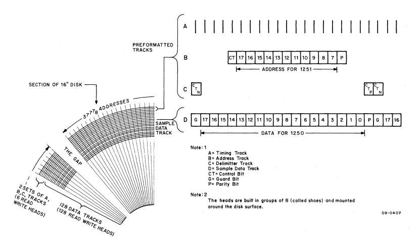
Figure 1-4 Disk Surface Recording Format
