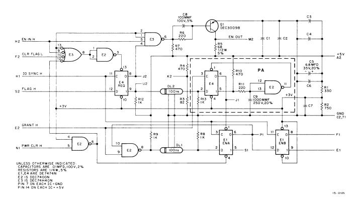
Figure 2-23 M104 Multiplexer, Circuit Schematic
