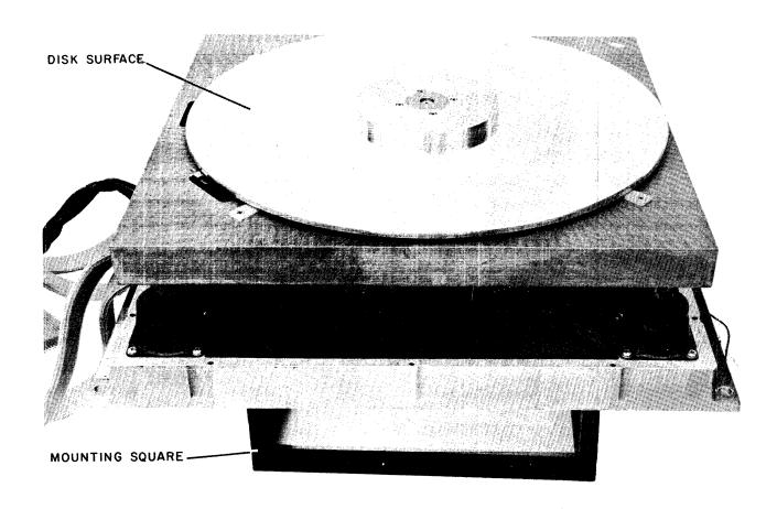
Figure 3-1 Disk Assembly With Cover Removed
