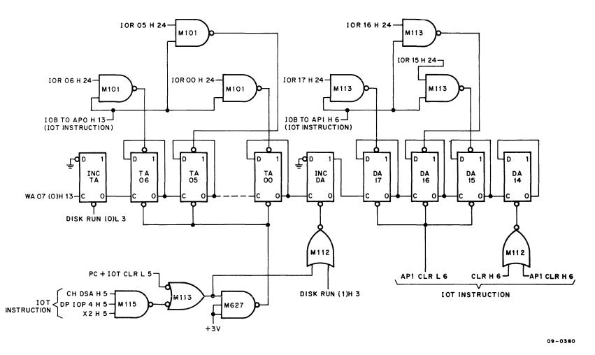
Figure 4-12 Track and Disk Address Register
