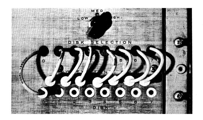
Figure 1-11 Transfer Rate Selection Switch and Disk Address Select Jacks
