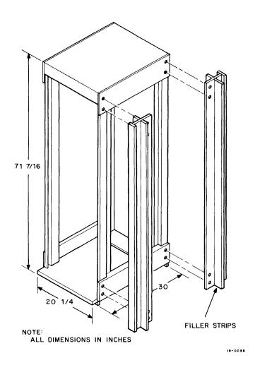
Figure 5-3 Cabinet Bolting Diagram
