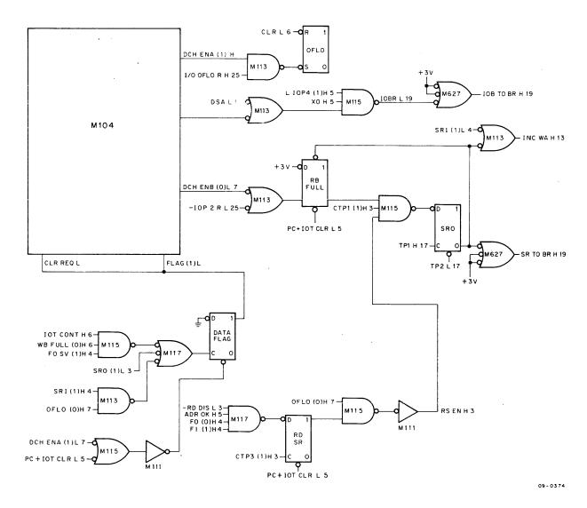
Figure 4-22 DCH Control for READ
