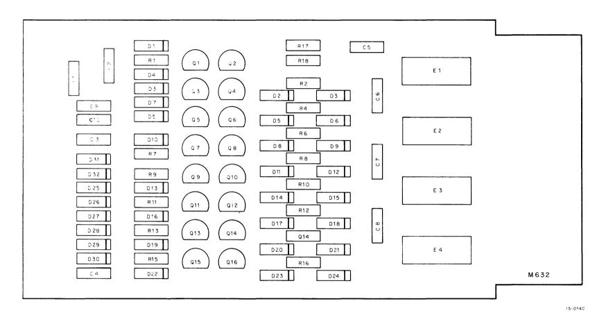
Figure 2-34 M632 Negative Driver, Parts Location Diagram
