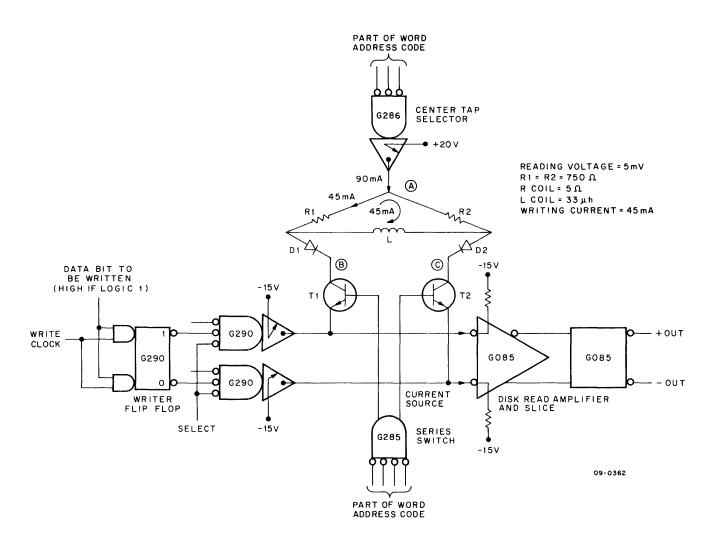
Figure 3-5 DECdisk READ/WRITE Electronics
