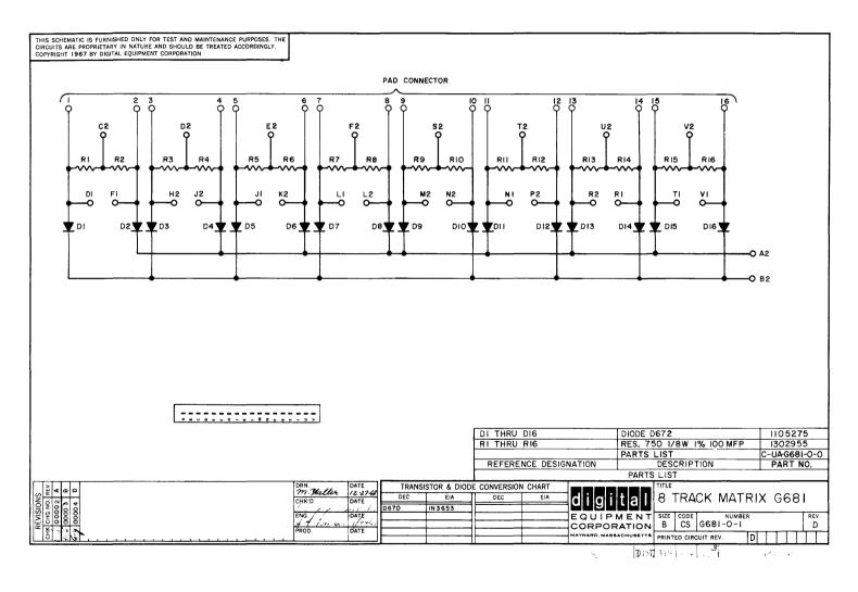
Figure 2-15 G681 Track Matrix, Circuit Schematic
