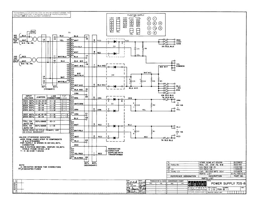
Figure 2-36 · 705B Power Supply, Circuit Schematic
