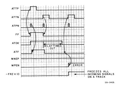
Figure 4-2 A Track Error Detection, Timing Diagram
