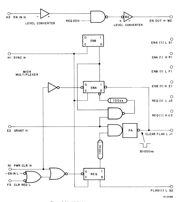
Figure 2-21 M104 Multiplexer, Block Schematic
