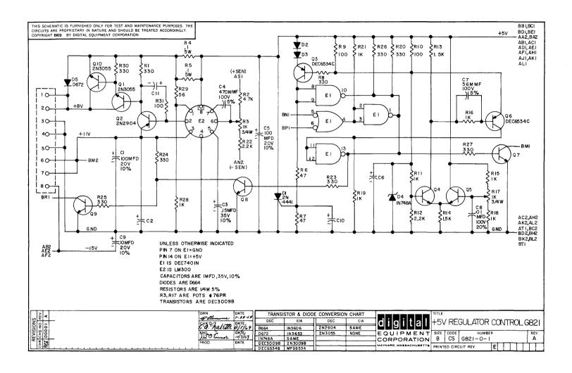
Figure 2-20 G821 +5V Regulator Control, Circuit Schematic
