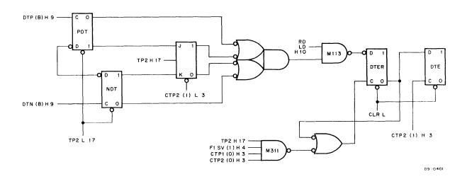
Figure 4-5 Data Track Error Detection Logic
