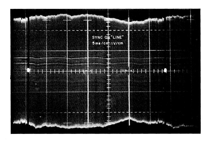
Figure 7-10 Measuring Surface Modulation on the A Track
