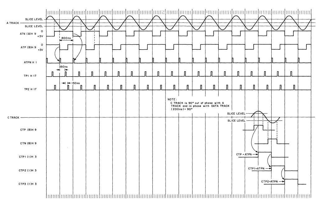
Figure 4-10 Timing Generator, Timing Diagram
