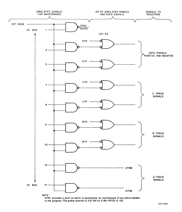
Figure 1-8 Simulating the RS09 with the Maintenance Logic
