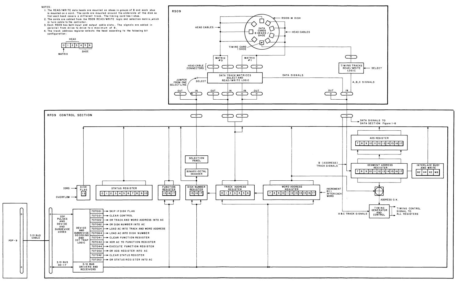
Figure 1-5 DECdisk Control Section 09-0413
