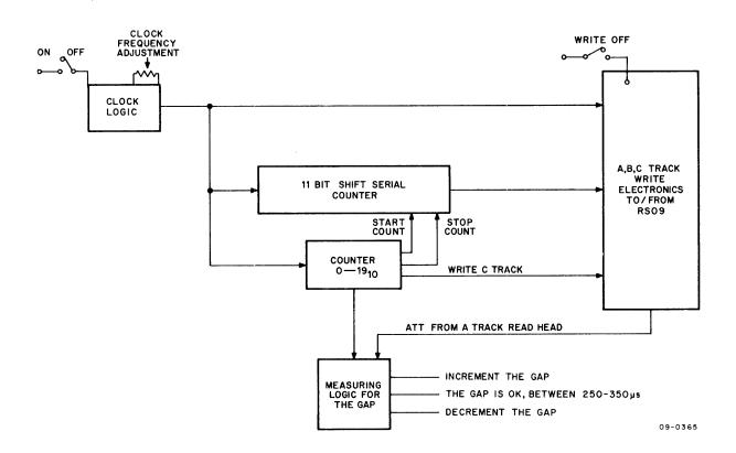
Figure 3-9 Timing Track Writer, Block Diagram
