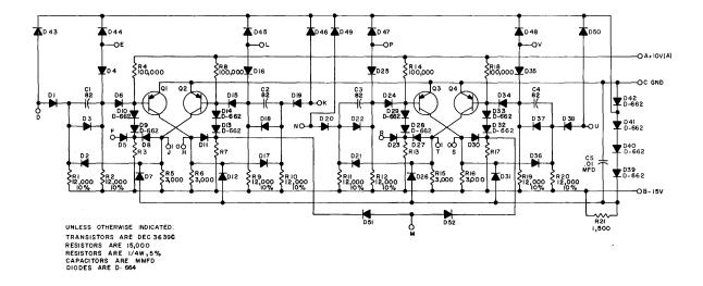
B-CS-S202-0-1 Dual Flip-Flop S202, Circuit Schematic
