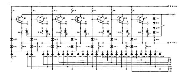
B-CS-S181-0-1 DC Carry Chain S181, Circuit Schematic
