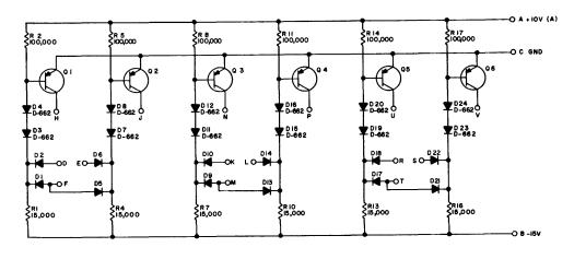
UNLESS OTHERWISE INDICATED: TRANSISTORS ARE DEC 3639 RESISTORS ARE 1/4 W,5% DIODES ARE D-664
