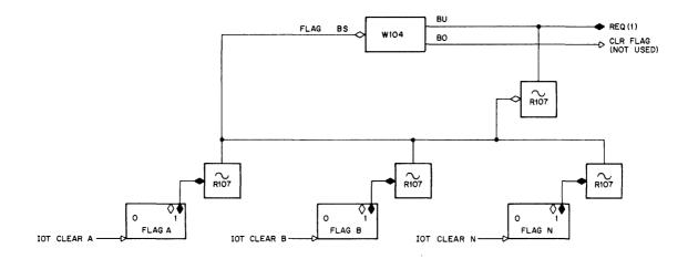
Figure 2-4 Single Device with Multiple Flags
