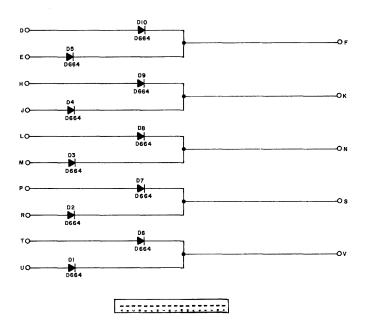
B-CS-R002-0-1 Diode Network R002, Circuit Schematic
