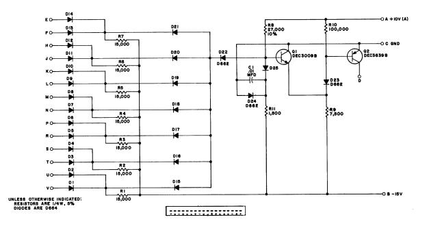
B-CS-R141-0-1 AND/OR Gate R141, Circuit Schematic
