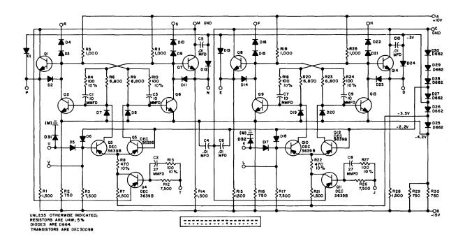
B-CS-B213-0-1 Dual Flip-Flop B213, Circuit Schematic
