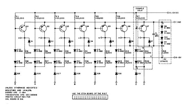
B-CS-S107-0-1 Inverter S107, Circuit Schematic
