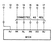
Figure 2–2 Connections for Trap Addresses Between  $100_8$  and  $137_8$
