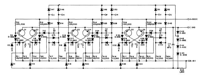
UNLESS OTHERWISE INDICATED: RESISTORS ARE 1/4W;5% CAPACITORS ARE MMFD DIODES ARE D-664 TRANSISTORS ARE DEC 3639C
