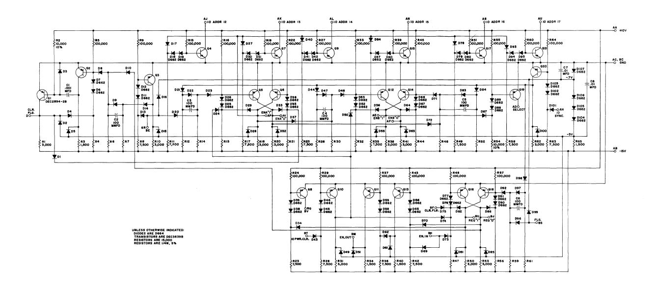
D-CS-W104-0-1 Multiplexer W104, Circuit Schematic
