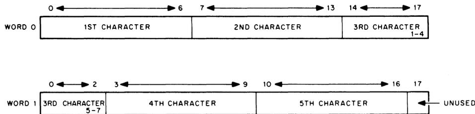
Figure 2-7 5/7 ASCII Packing Scheme
