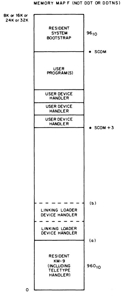
The System Loader learns which I/O handlers are required by the Linking Loader, loads them relocatably and then loads the Linking Loader relocatably.
