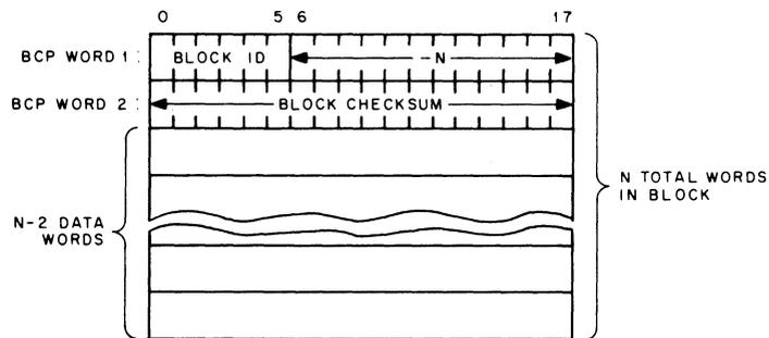
Figure 5-4 Block Format, File-Structured Mode
