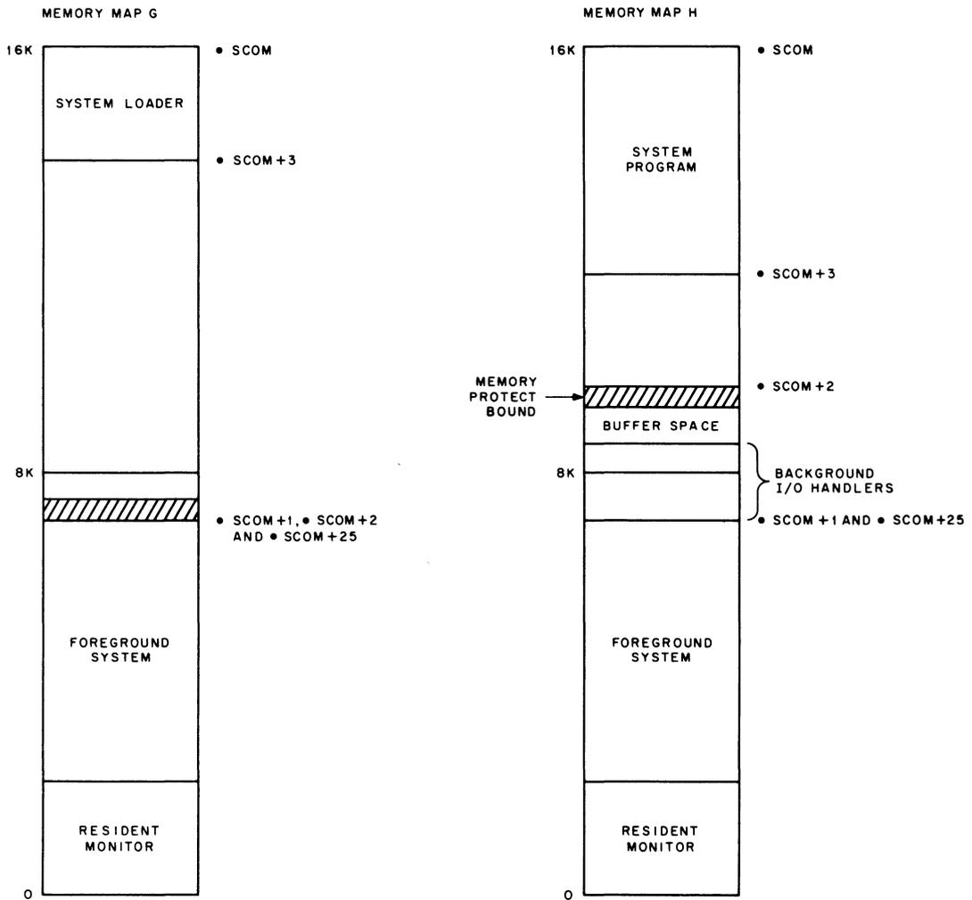
When a keyboard command requests loading of a BACKGROUND system or user program, the non-resident Monitor brings in the System Loader, overlaying itself.
