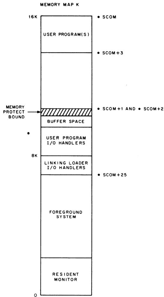
The .EXIT from the Linking Loader causes the user program I/O handlers to be block transferred to their running position, the memory protect bound to be set just above the buffer space, and control given to the user program.
