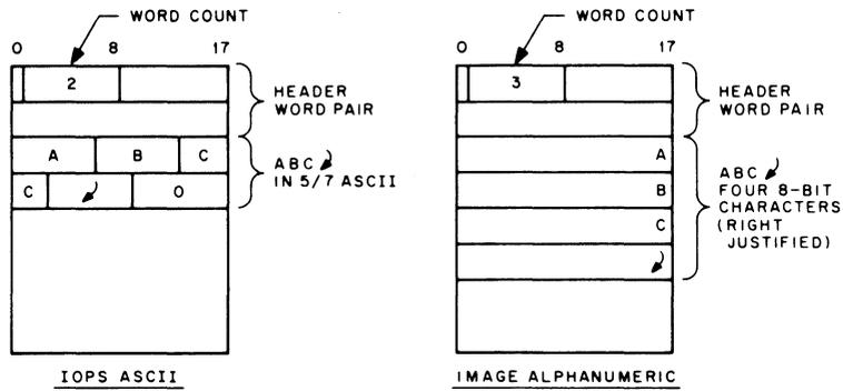
Figure 2-9 IOPS ASCII and Image Alphanumeric Data in Line Buffers
