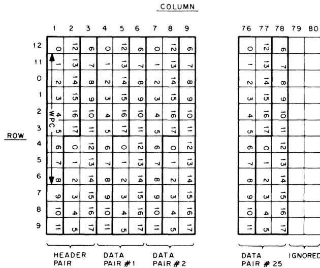
Figure 7-2 IOPS Binary Input Card Format
