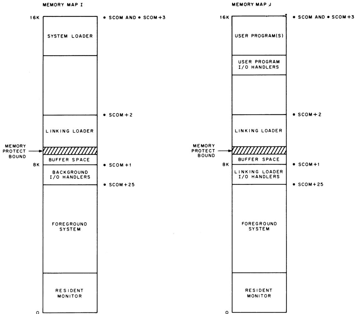
If the BACKGROUND program is a user program, the System Loader loads the Linking Loader I/O handlers up from the top of the FOREGROUND system, allocates buffer space, and loads the Linking Loader such that the memory protect bound can be set just below it.
