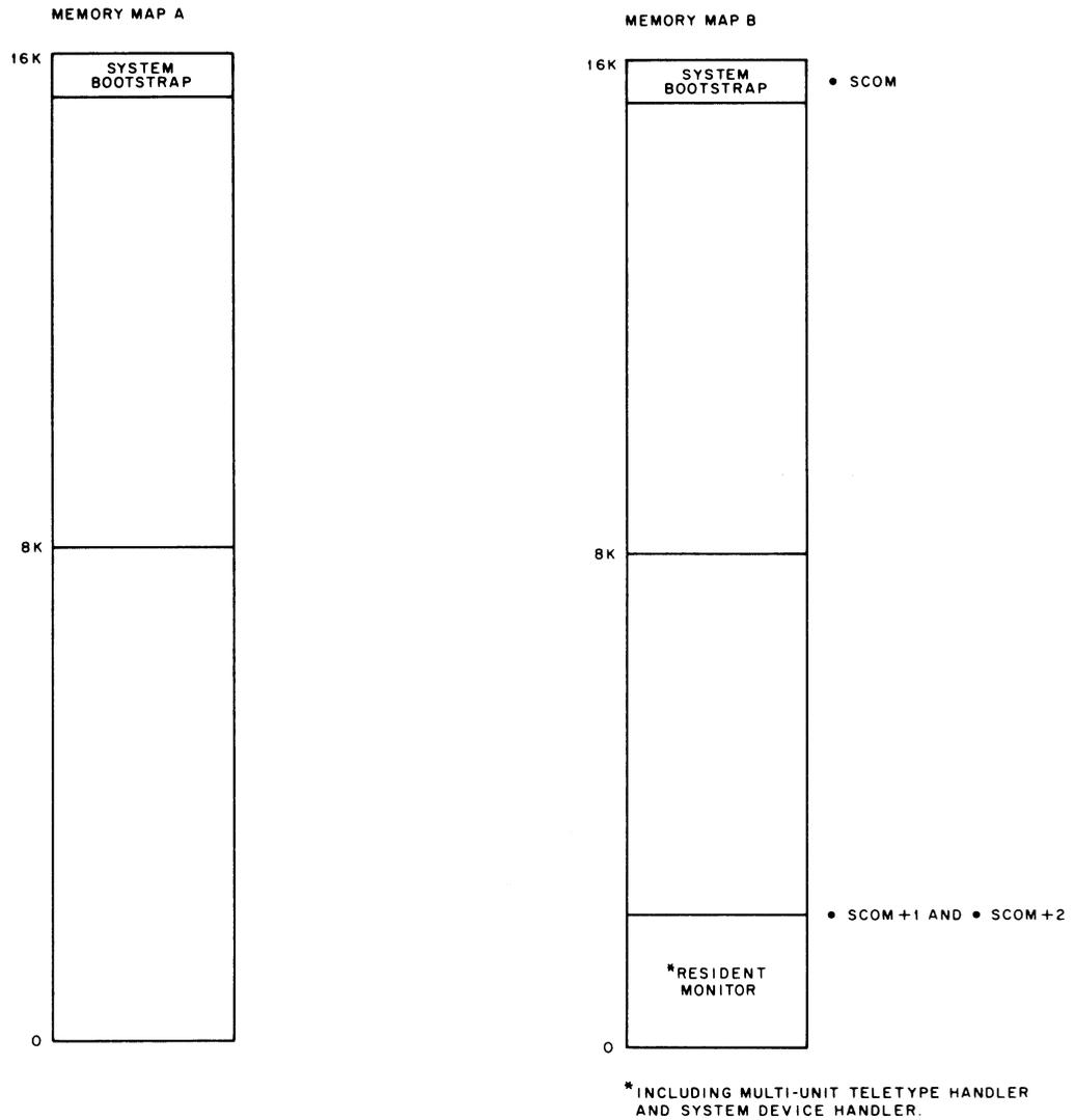
The System Bootstrap is loaded at the top of core via the paper tape reader in HRM format.
