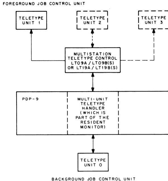
Figure 6-1 Keyboard Communication in Background/Foreground Monitor System
