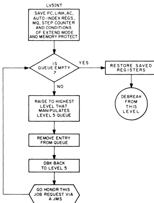
Figure 7-1 Structure of API Software Level Handler
