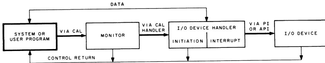
Figure 2-1 General I/O Communication in Monitor Environment
