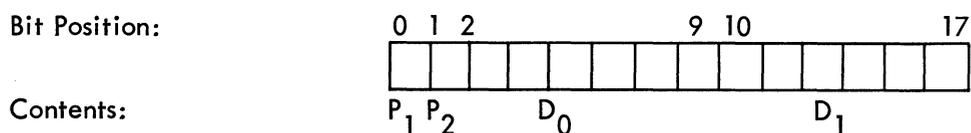
Parity Bits ( $P_0$ ,  $P_1$ ): Bits 0 and 1 of the PDP-9 word are used as parity bits for the two 8-bit data bytes ( $D_0$  and  $D_1$ ), respectively, in the low-order portion of the register. During an output (write) transfer, these bits are ignored. The hardware generates the proper parity for each data frame. During an input (read) transfer, these bits are set to the actual parity values for the two data frames as read from tape.
