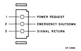
Figure 2-2 Signal Bus Connector
