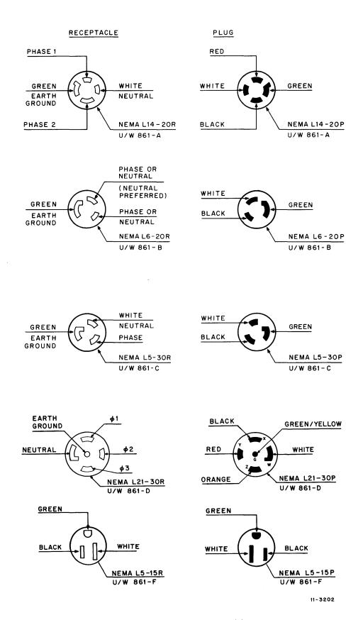
Figure 2-1 Connector Wiring
