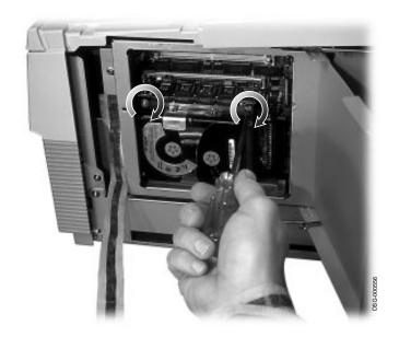
5. Wiggle the disk drive option to unplug and remove it.
