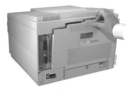
2. Press the green lever  $\mathbf{0}$  to release the paper then remove the jammed paper from the printer.
