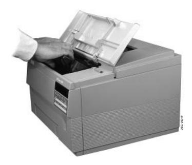
3. Clean the anti-static teeth using the green cleaning brush (stored in the printer).
