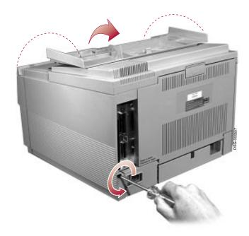
3. Remove the side cover by sliding it toward the back of the printer and then tilting it out.
