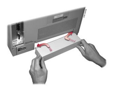
2. Insert the paper length stop and the paper width stop into the slots that represent the paper size you want to load.
