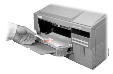
$\sqrt{\phantom{a}}$  If the jammed paper is not accessible or easily removed from the front tray, go to Section 9.3.
