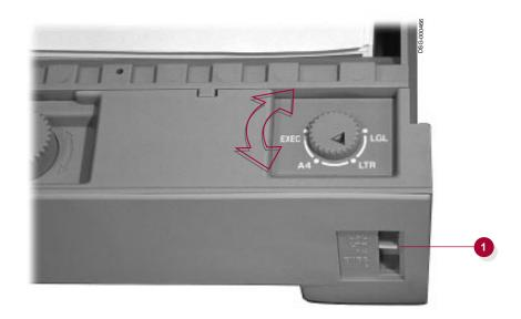
4. If you are loading paper for the first time, you must adjust the tray spring tension for optimum paper handling performance. If you do not adjust the spring tension, the paper may not feed correctly resulting in excessive paper jams. Always adjust the tray spring tension with the tray fully loaded (about 500 sheets).
