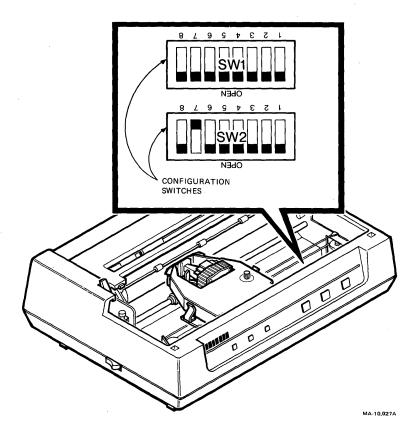
Figure 3-2 LA50 Printer Configuration Switches
